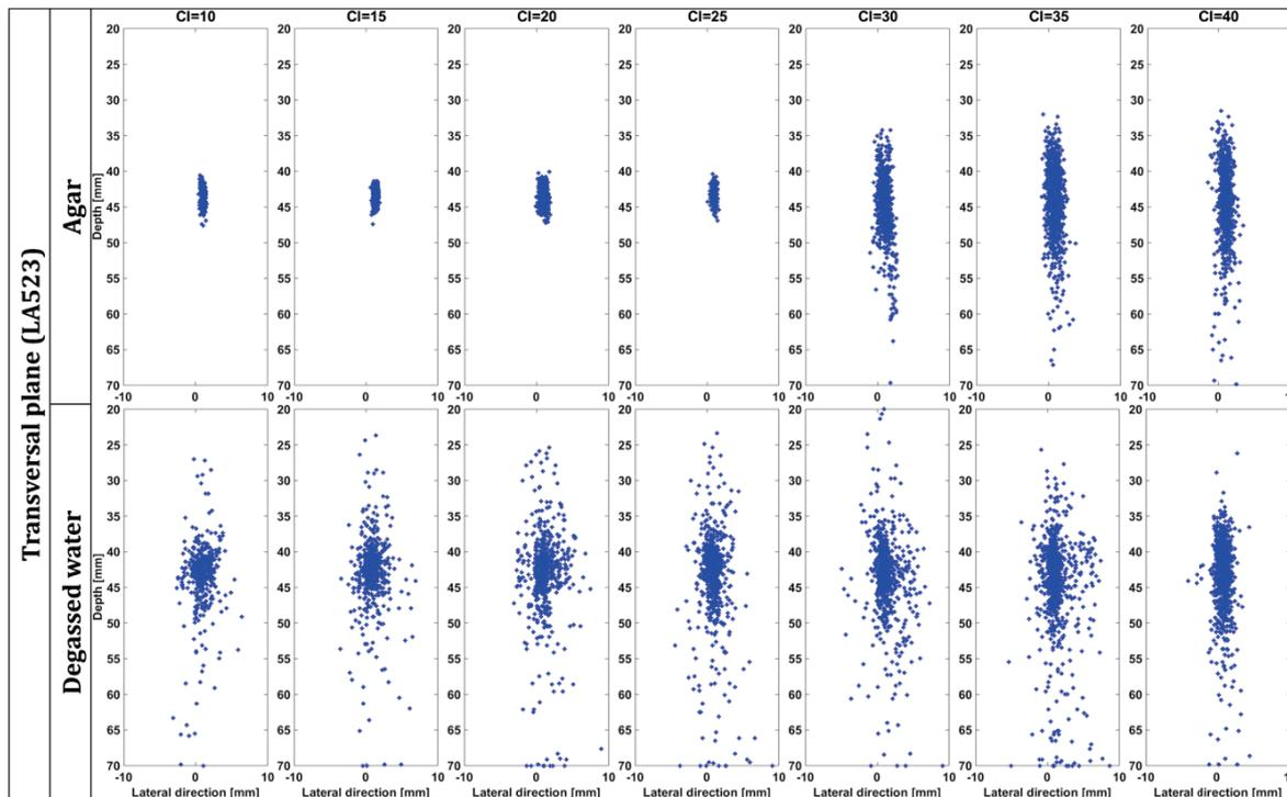
Figure III-6: Two dimensions focal cavitation point (FCP) positions along 500 ms of overall sonication for the cavitation transversal plane (LA523) with or without agar gel and with an increasing cavitation index (CI).
