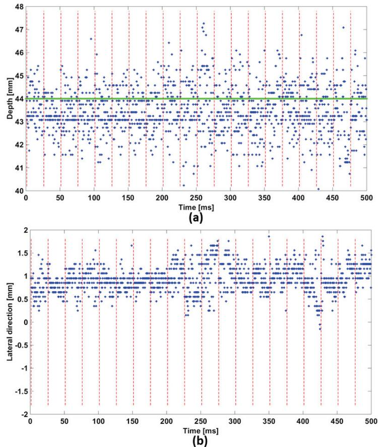
Figure III-5: Enhanced scale for the FCP localization temporal profile along 500 ms of sonication for both (a) depth and (b) lateral imaging direction.
