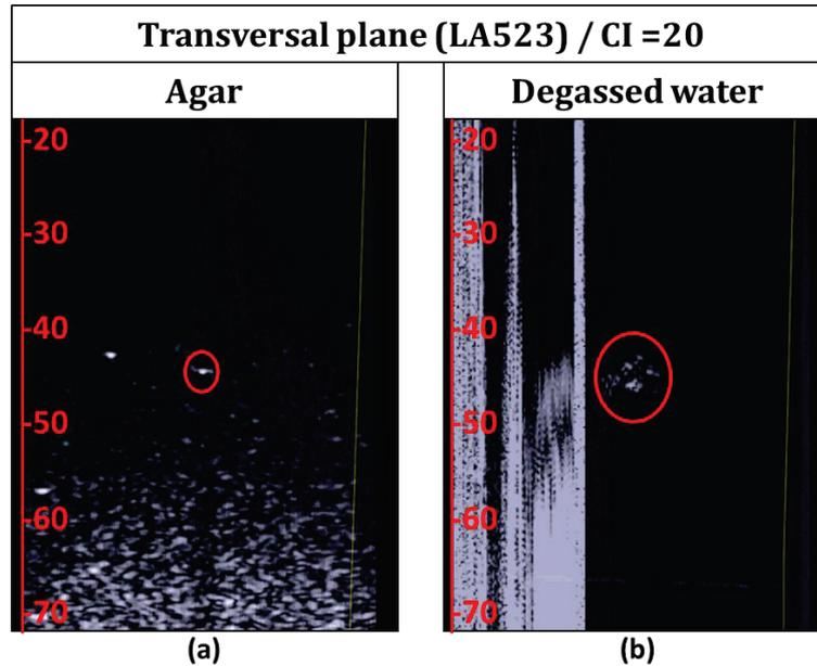
Figure III-11: Screenshots of the B-mode visualization for the cavitation transversal plane (LA523), for a cavitation index  $CI=20$ , and (a) with or (b) without agar gel. The white flash observed on the left side of the B-mode image in degassed water corresponds to the end of the sonication pulse. The red oval-circle delimits the hyperechoic area observed during the B-mode visualization.
