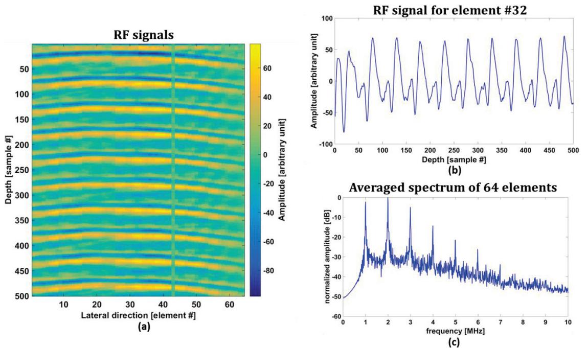
Figure III-24: Reference non-saturated RF pre-beamformed signal recorded by the LA332 probe during the one-spot cavitation experiment in degassed water, with  $Cl=20$ , and for frame #36: (a) the 64 total RF signals, (b) the RF signal plot for central element number 32, and (c) the averaged spectrum over the entire 64 total active elements. Element number 43 was damaged and so the corresponding RF signal wasn't considered.
