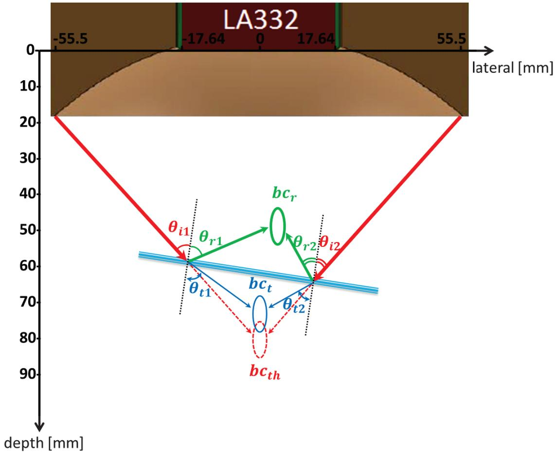
Figure III-38: Illustration presenting the refraction/reflection ultrasound propagation mechanism impact on the bubble cloud (therapy focus) generated by the ultrasound sonication therapy.  $bc_{th}$  = theoretical bubble cloud,  $bc_t$  = transmitted bubble cloud, and  $bc_r$  = reflected bubble cloud. The blue triple line corresponds to the water-balloon-skin-tissue interface.
