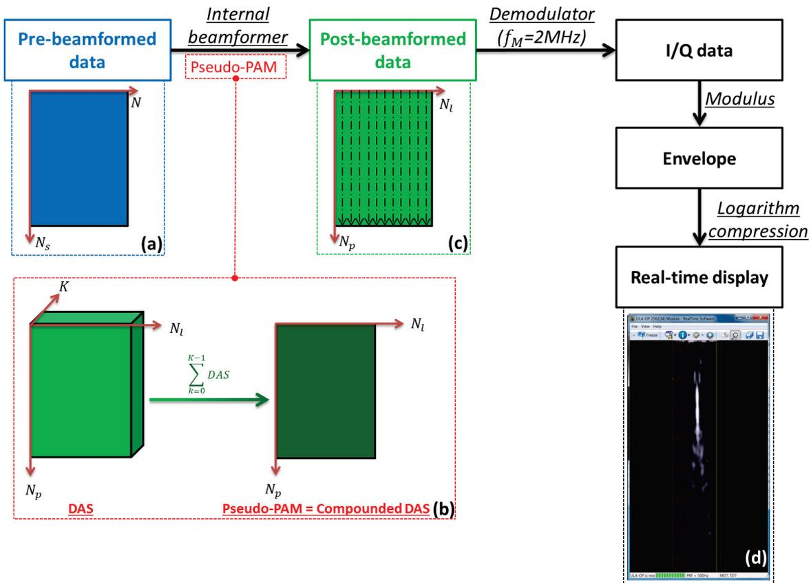
Figure IV-16: Real-time display implementation in the ULA-OP 256 platform of (b) the “Pseudo-PAM” technique passing from (a) pre-beamformed data to (c) post-beamformed data and finally to (d) passive images displayed in real-time (screenshot of the real-time visualization tool). The experiment on a wire was considered in this example for real-time display with a 500 Hz frame rate and  $k=10$  (number of compound).
