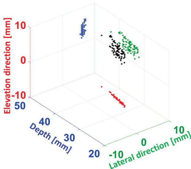
Figure IV-5: The FCP 3D positions recovered from the 100 PAM-PCF reconstructed maps for the cavitation experiment. The positions for the three directions are plotted in black. The position projections are plotted on the lateral direction ( $x=10$ ) in green, on the depth direction ( $y=50$ ) in blue, and on the elevation direction ( $z=-10$ ) in red.
