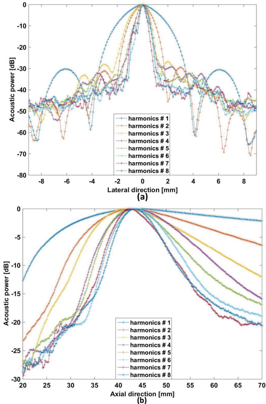
Figure IV-14: The acoustic pattern profiles in the (a) lateral and (b) axial direction for the 8 different harmonic number choices.
