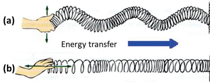
Figure I-1: (a) Transverse wave with oscillations perpendicular to the energy transfer propagation. (b) Longitudinal wave with oscillations parallel to the energy transfer propagation [33].
