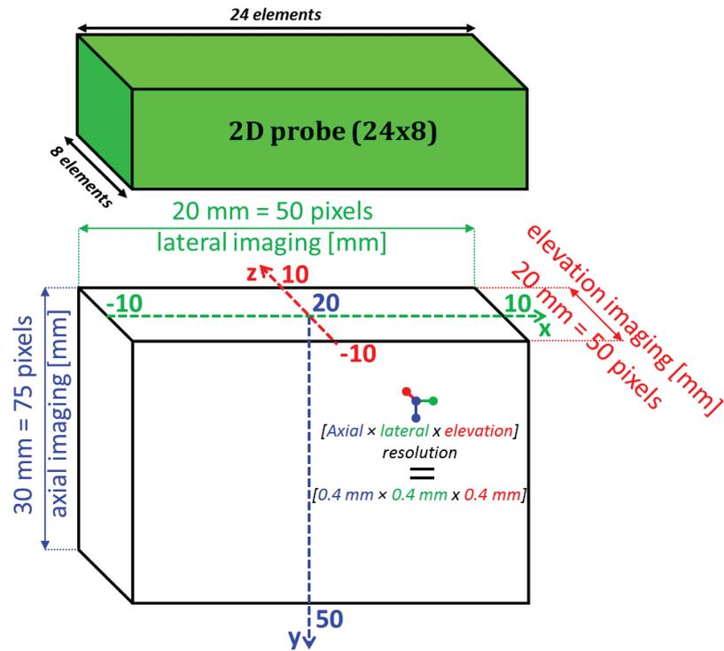
Figure IV-3: The image reconstruction parameters for the 2D matrix array imaging both cavitation transversal plane  $(x, y) = (\text{lateral, axial})$  imaging direction and cavitation frontal plane  $(z, y) = (\text{elevation, axial})$  imaging direction.
