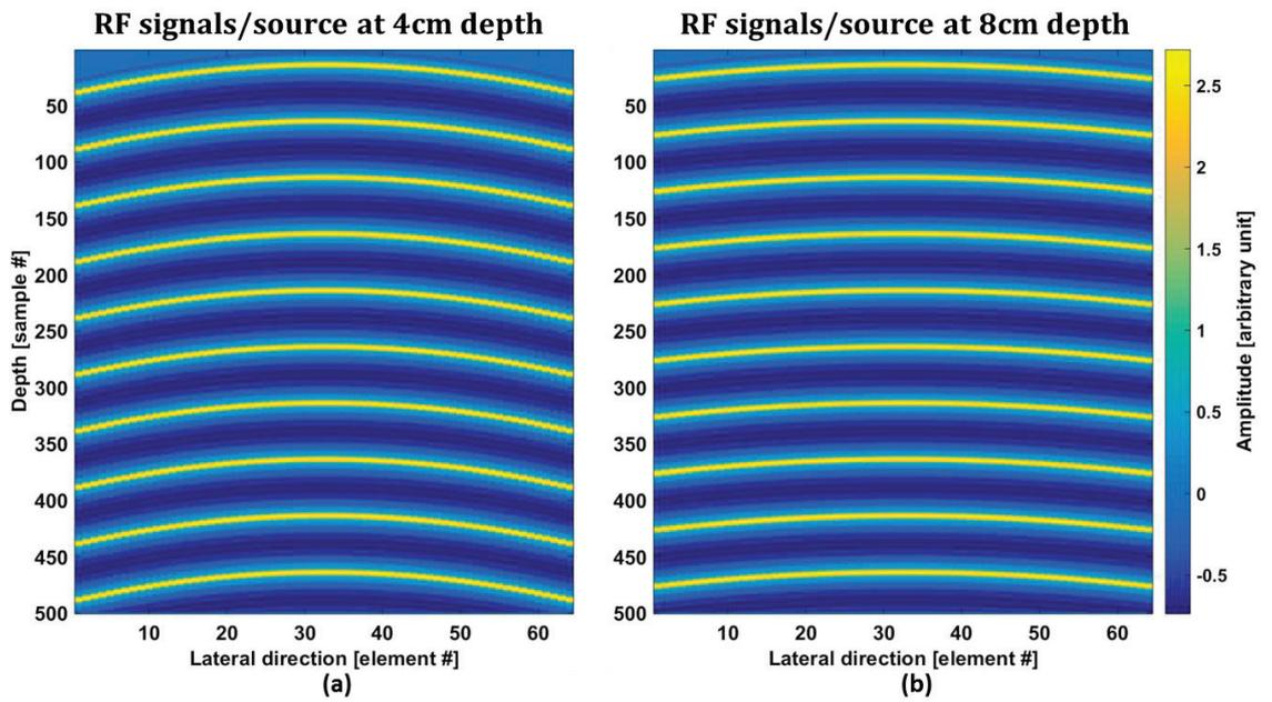
Figure II-9: Pre-beamformed simulated RF signals using 64 central elements.
