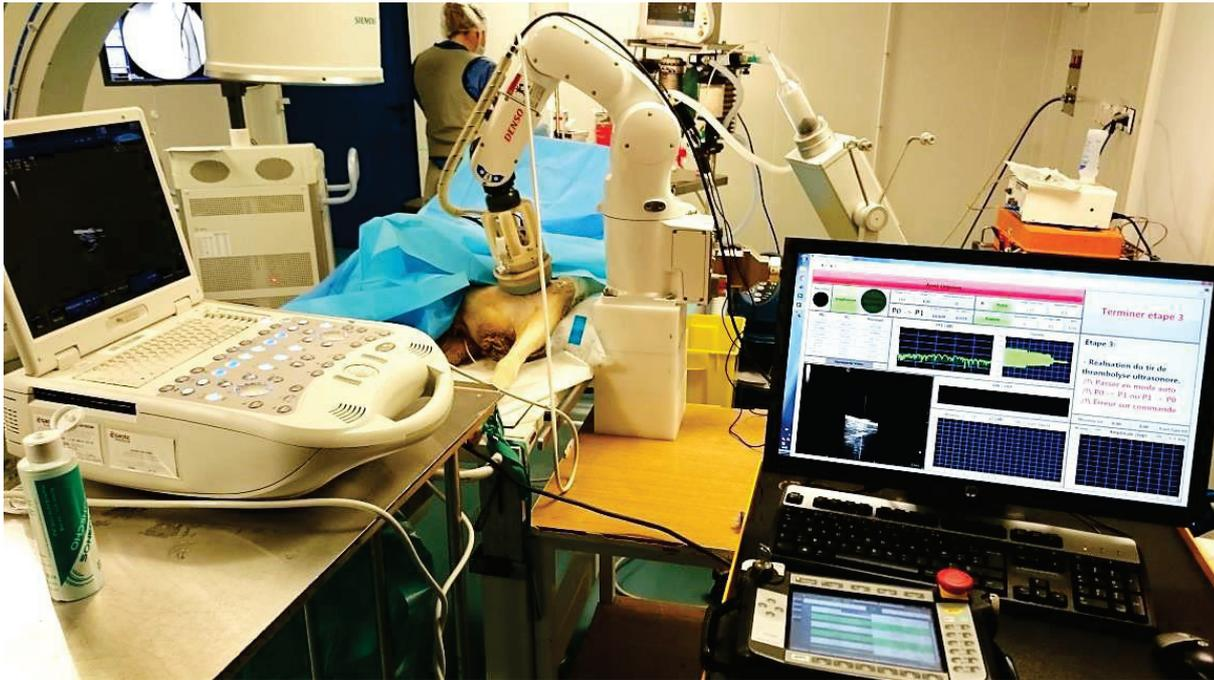
Figure III-32: Picture of the *in vivo* experimental testing during ultrasound sonication shots. The therapy device is placed on the sheep's leg thanks to the robotic arm system. [97]
