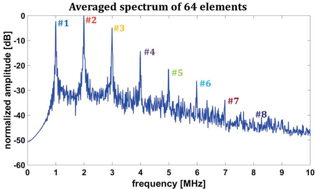
Figure IV-12: Averaged spectrum along the entire 64 active elements of the LA523 imaging probe before any additional frequency-harmonics filtering process with the harmonics number # ( $n_h$ ) outlined on the plot. Harmonic #1 corresponds to the fundamental signal.
