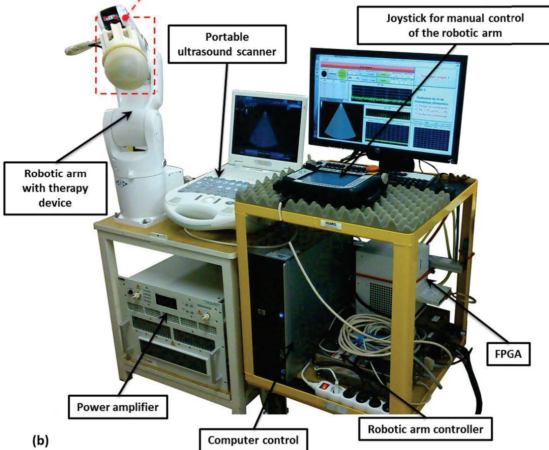
Figure III-31: (a) Cut plane of the *in vivo* therapy device including mainly the therapeutic transducer, the hydrophone, the imaging probe LA332, and a coupling balloon. (b) *In vivo* complete experimental thrombolysis setup including the regulated induced-cavitation generator system, an ultrasound scanner, and a 6-axis robotic arm system. [97]
