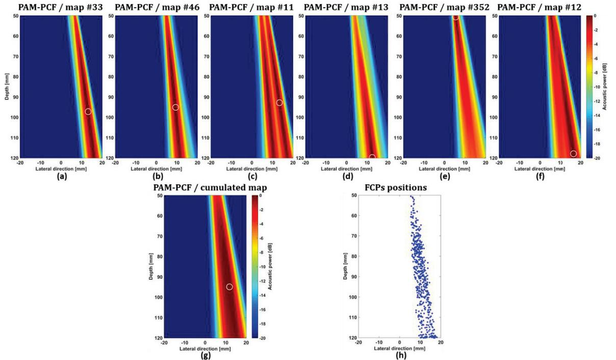
Figure III-27: Results for case #2 where only the  $out_2$  was ON (only  $bc_2$  bubble cloud was present). (a-f) The cavitation map reconstructed with the PAM-PCF method from six different passive acquisition frames. (g) The cumulated map along 616 maps and (h) the FCP 2D positions. The white circle corresponds to the FCP localization.
