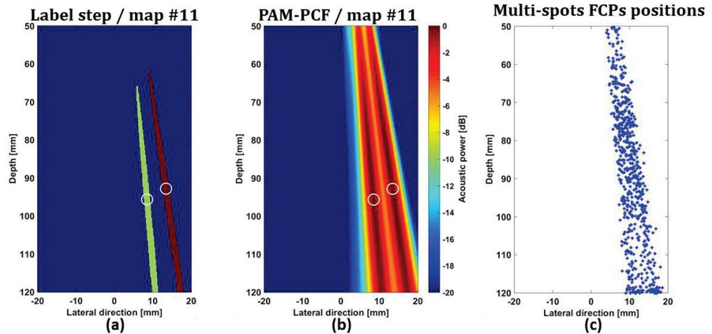
Figure III-29: For case #2 where only the  $out_2$  was ON (only  $bc_2$  bubble cloud was present). (a) The 2 connected objects (cavitation spots) recognition after applying the threshold then the label segmentation step on the PAM-PCF cavitation map frame #11. (b) The PAM-PCF cavitation map frame #11 with multi-spots FCP localization. The white circle corresponds to the FCPs localization. (c) The overall 2D FCPs positions including all multi-spots cavitation recognized.
