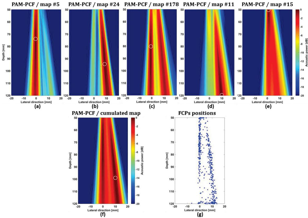
Figure III-28: Results for case #3 where both  $out_1$  and  $out_2$  was ON (both  $bc_1$  and  $bc_2$  bubble clouds were present). (a-e) The cavitation map reconstructed with the PAM-PCF method from five different passive acquisition frames. (f) The cumulated map along 616 maps and (g) the FCP 2D positions. The white circle corresponds to the FCP localization.
