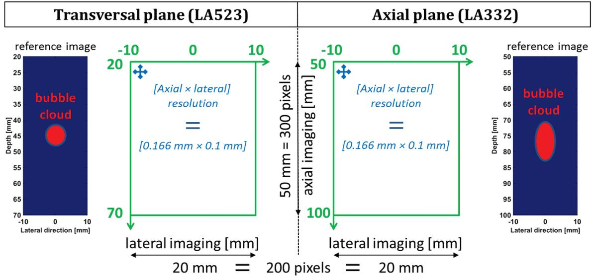
**Figure III-3:** Image reconstruction parameters for both probes LA523 and LA332 respectively imaging the cavitation transversal plane ( $x, y$ ) and the cavitation axial plane ( $x, z$ ). Reference images are displayed to outline the bubble cloud shape and focal point localization for each cavitation planes. The bubble cloud limits are not at the right scale, it is used as a representative reference image.
