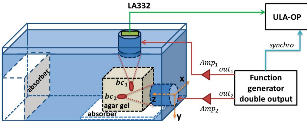
Figure III-20: Cavitation experiment setup using two therapeutic transducers to induce two separate bubble clouds ( $bc_1$  and  $bc_2$ ). The imaging system with one imaging probe (LA332) is synchronized with both sonication pulses.
