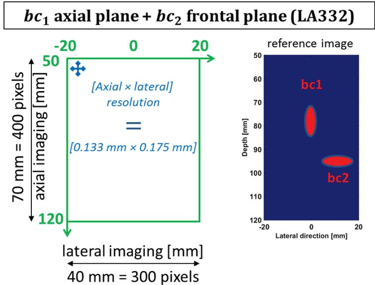
Figure III-25: Image reconstruction parameters for LA332 probe imaging the  $(z, y)$  plane corresponding to the cavitation axial plane of the bubble cloud ( $bc_1$ ) and the cavitation frontal plane of the bubble cloud ( $bc_2$ ). A reference image is displayed to outline the bubble cloud shape and focal point localization. The bubble cloud limits are not at the right scale, it is used as a representative reference image.
