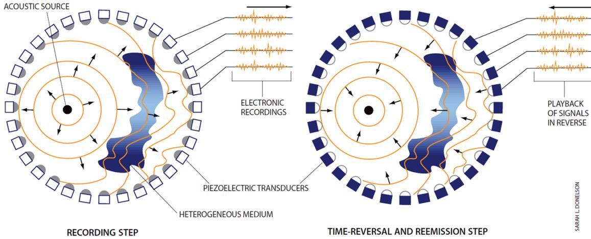
Figure II-1: Time reversal mirrors technique [118].
