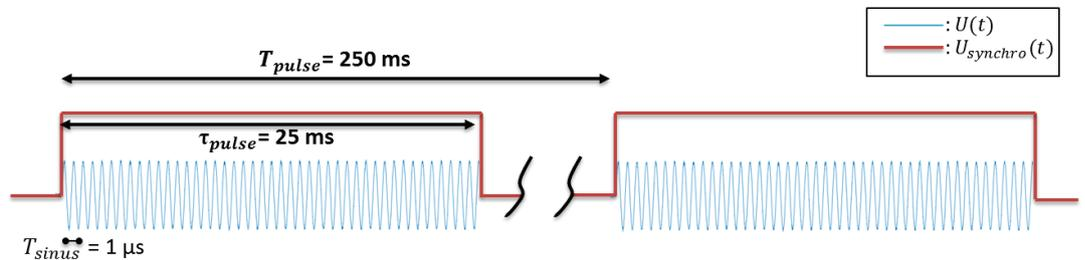
Figure II-4: Two synchronous signals are generated by the FPGA module of the US cavitation generator system: the sonication signal  $U(t)$  sent to the therapeutic transducer and the output synchronization signal  $U_{\text{synchrono}}(t)$ .
