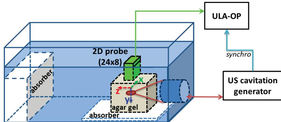
Figure IV-1: Cavitation water tank experiment setup using the regulated US-induced cavitation generator to induce a bubble cloud in an agar gel, with a CI=30dB. In addition, a 2D imaging matrix probe with 24 by 8 elements is combined with the ULA-OP synchronized with the ultrasound sonication pulses.
