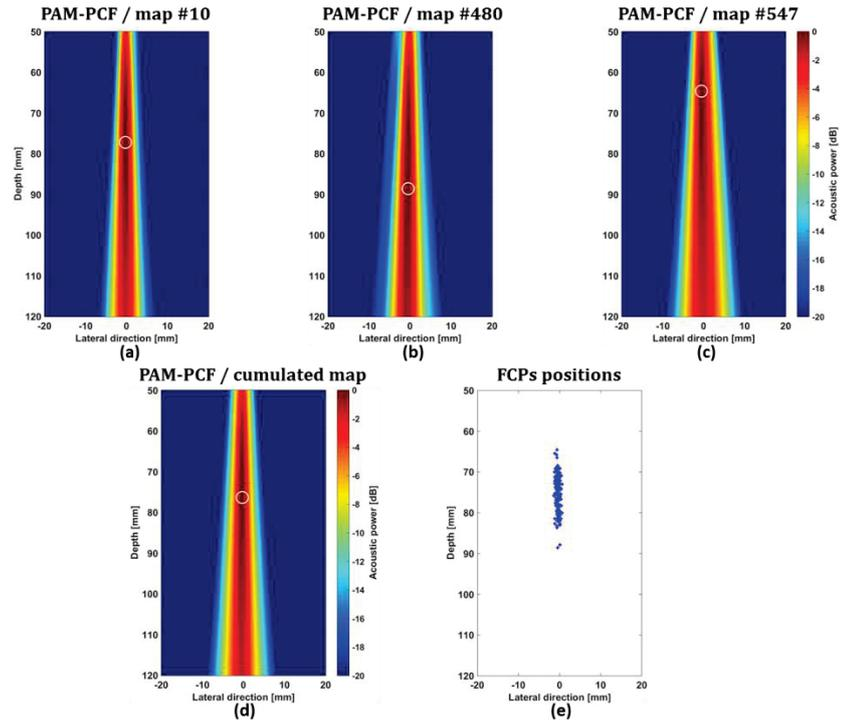
Figure III-26: Results for case #1 where only the  $out_1$  was ON (only  $bc_1$  bubble cloud was present). (a-c) The cavitation map reconstructed with the PAM-PCF method from three different passive acquisition frames. (d) The cumulated map along 616 maps and (e) the FCP 2D positions. The white circle corresponds to the FCP localization.
