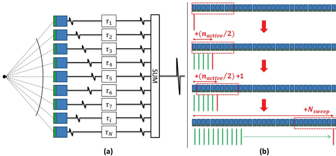
Figure I-3: (a) Delay and sum (DAS) beamforming method allowing focalization in reception. (b) Electronic sweep of the active elements ( $n_{active}$ ) on the entire imaging array. The vertical lines correspond to the post-beamformed lines.
