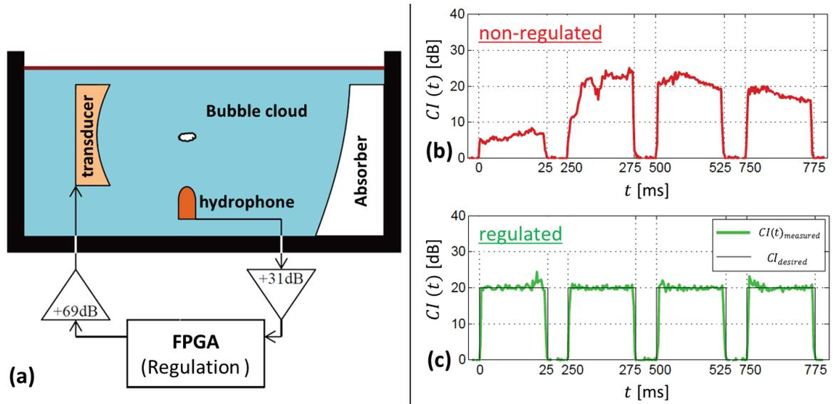
Figure I-7: (a) experimental setup. Temporal evolution of the real time computed cavitation index  $CI(t)$  (b) without regulation or (c) with regulation [97].
