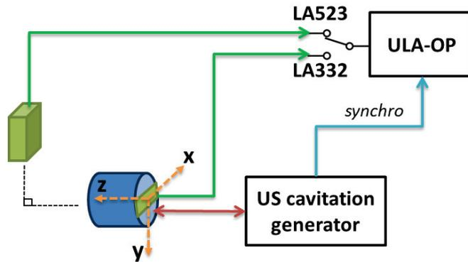
Figure II-2: General setup using both the therapeutic system (US cavitation generator) and the imaging system with ULA-OP paired with two imaging probes (LA523, LA332) synchronized with the therapeutic pulses.
