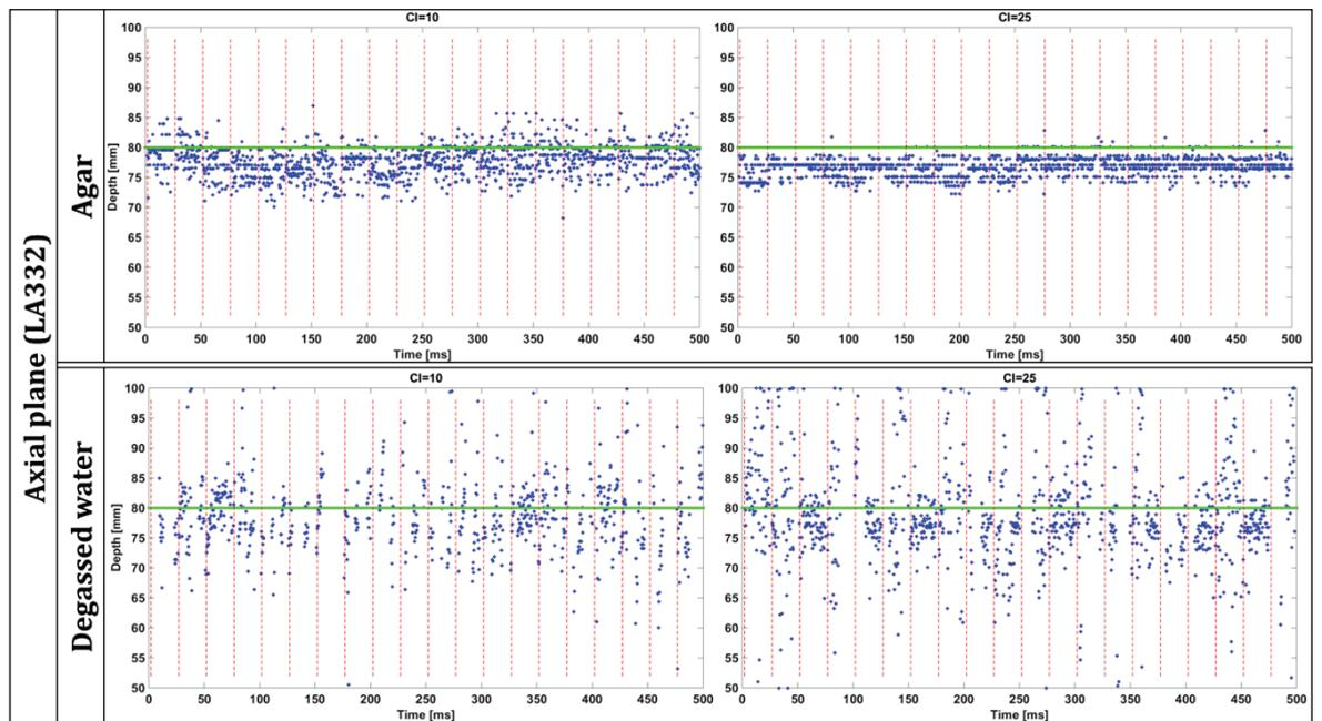
Figure III-9: The FCP localization temporal profile along 500 ms of sonication for the cavitation axial plane (LA332), with or without agar gel and for cavitation index (CI) equal to 10 or 25. The horizontal green line represents the FCP theoretical depth reference and the vertical red dotted line corresponds to the start of each sonication pulse.
