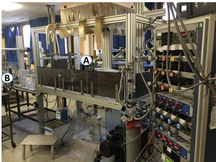
**Figure 3.2** Image of the laser pyrolysis setup.
