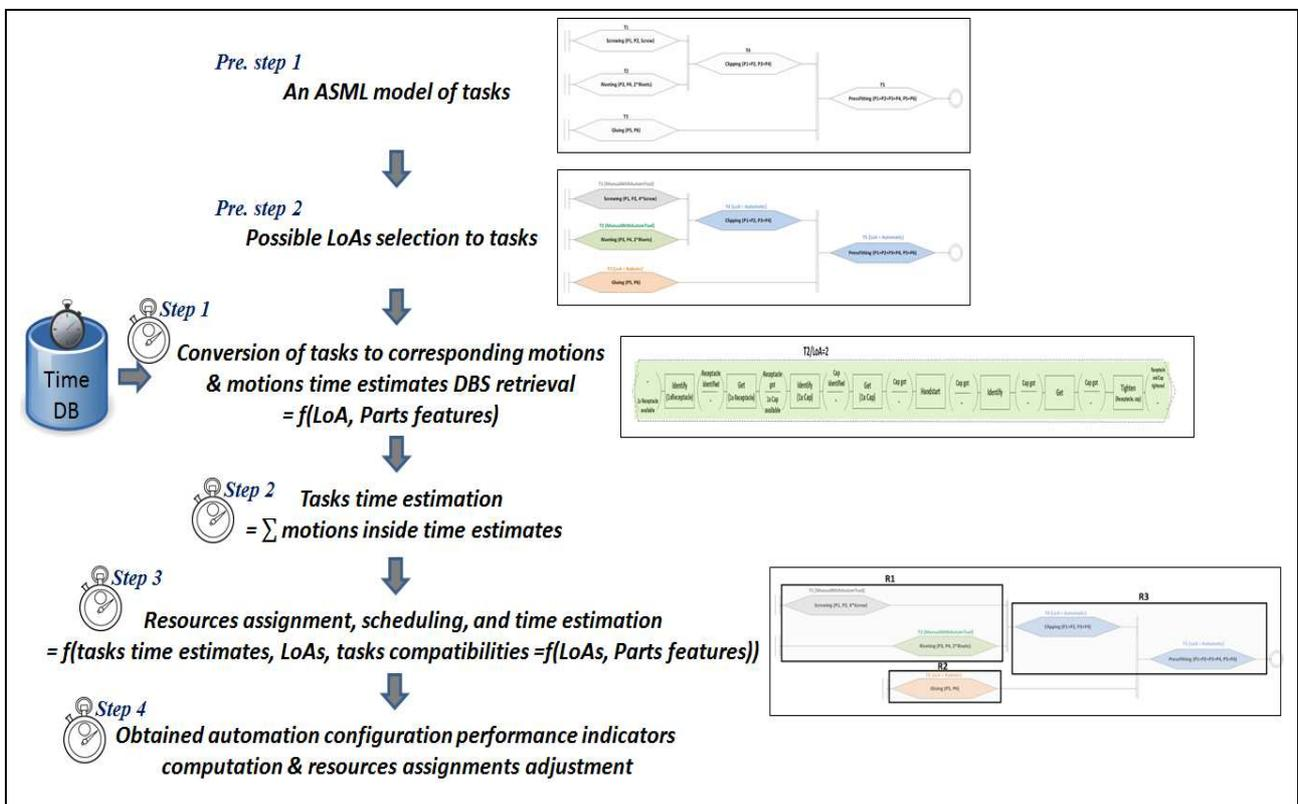
Figure 12: The decomposition of the previously considered automation configuration to motions
