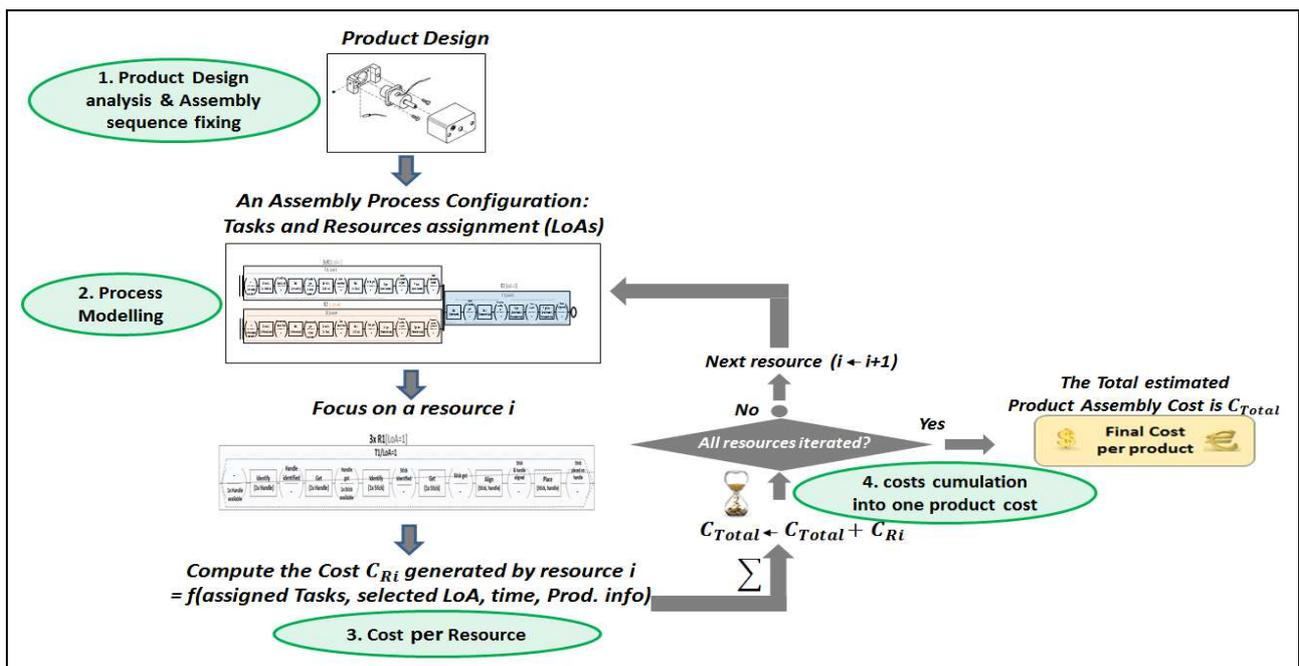
**Figure 20:** The product assembly cost estimation approach
