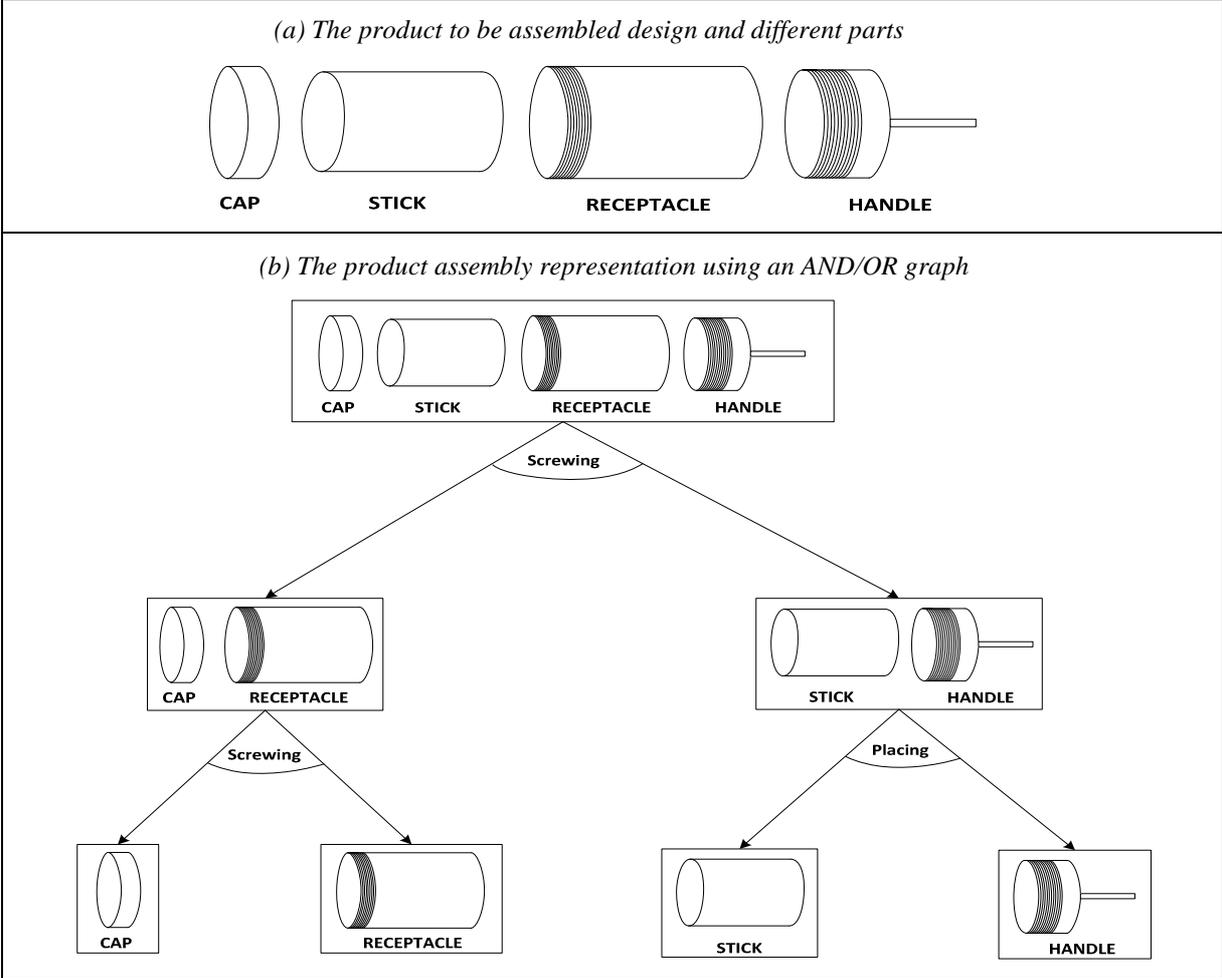
**Figure 8:** An example of an assembly system alternative
