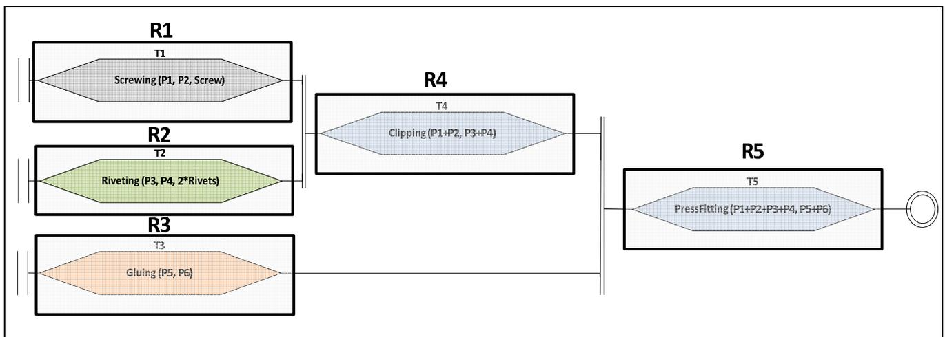
**Figure 18:** An alternative of resources assignments to tasks
