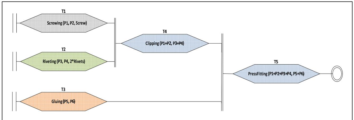
**Figure 17:** An automation combination to process tasks for a product assembly example
