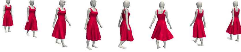
Figure 4.9: Our nodal algorithm efficiently handles the frictional contacts between the mannequin and her dress during a walking cycle.
