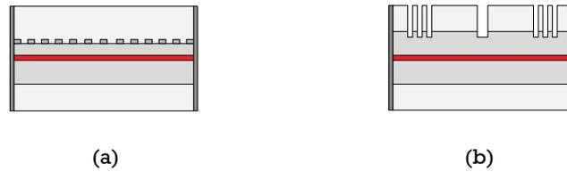
Figure 2.26: (a) Buried Bragg grating (darkest gray pattern). (b) Surface Bragg grating etched directly at the top of the cavity.
