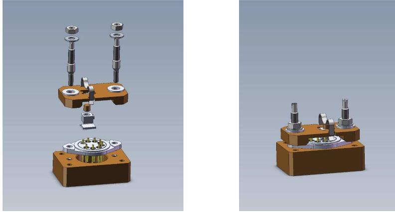
Figure 3.36: Mechanical assembly for TO3, peltier and C-mount soldering. Left: exploded view. Right: mounted assembly
