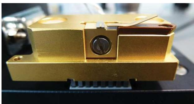
Figure 10: Platform onto which a laser packed on a C-mount is fixed. Thermal adjustment and stabilization is obtained by a Peltier element placed below the platform and a temperature controller. A cap (not shown) ensures proper protection against air fluxes.
