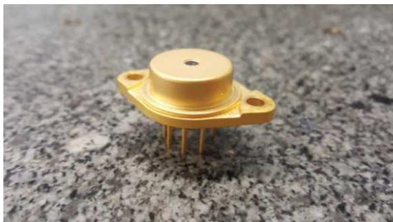
Figure 16: Example of TO3 packaged laser for direct use in atomic clock setup
