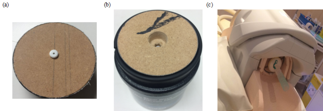
FIGURE 4.2: MRE experimental installation for the calibrated phantoms. A home-made cylindrical wood block with an acoustic adapter inserted in the center (a) was used to induce a point source excitation (b) and a knee coil (c) was used for signal reception.
