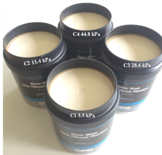
FIGURE 4.1: Four calibrated phantoms C1-C4 with corresponding Young's modulus 3.5, 11.4, 28.6, and 44.4 kPa
