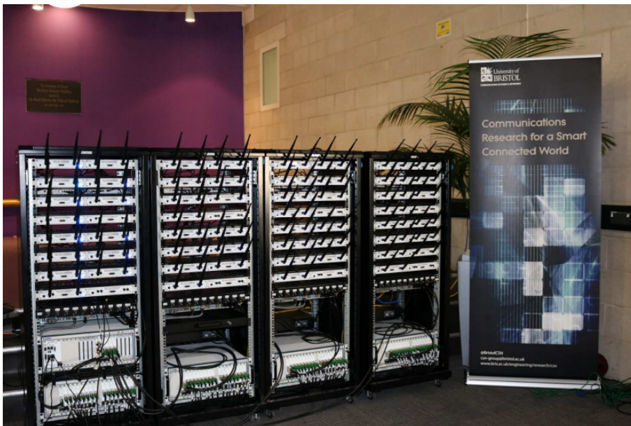
Figure 10.3: Bristol’s massive MIMO testbed.
