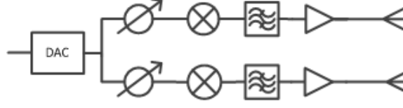
Figure 6.4: Equivalent hybrid structure where shared hardware components (mixers, filters) on RF chain are copied on each branch with phase shifters. The hardware components are then re-ordered such that all components in \mathbf{T}_A go to the front end near the antennas.
