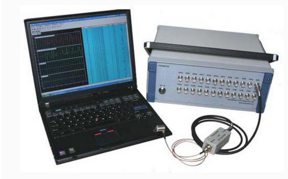
Fig. 6.2 Acoustic emission monitoring equipment.
