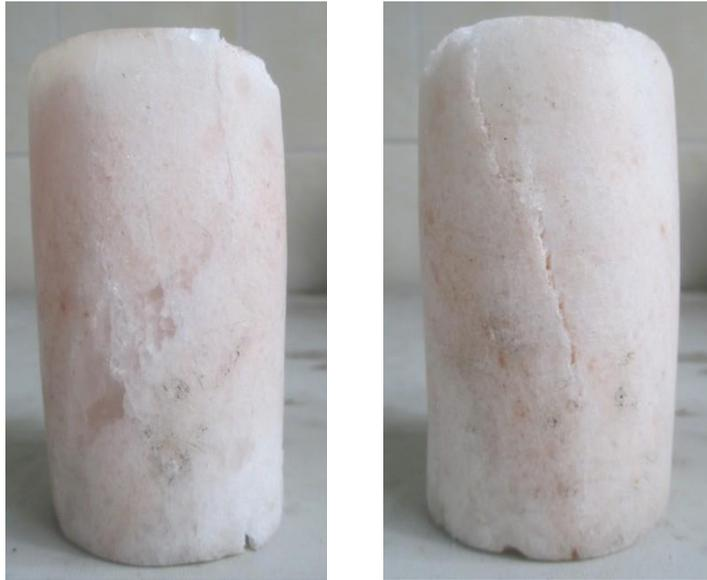
Fig.2.11 Specimen failed in the uniaxial test
