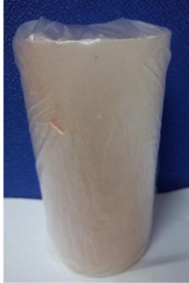
Fig.5.3 Sample encased in a plastic fresh-keeper bag.
