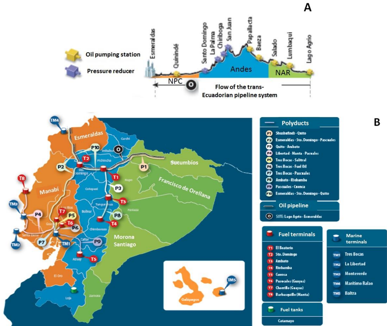
Figure IV. Oil transport and storage system in Ecuador. A. Trajectory of the Trans-Ecuadorian oil pipeline system, from the North Amazon region (NAR) to the North Pacific Coast (NPC). B. Polyducts, fuel terminals, tanks and marine terminals. (Modified from: EP Petroecuador, 2016)
