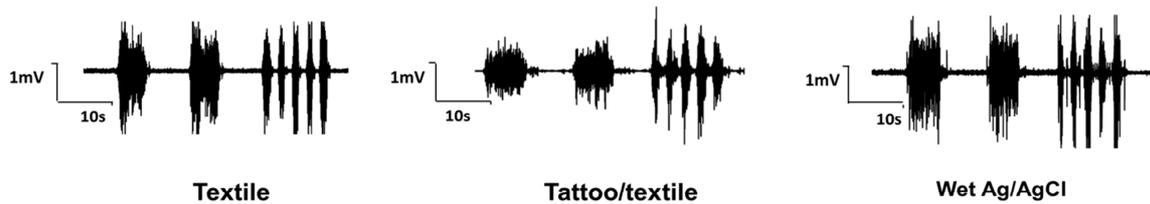
Figure 5.5 **EMG recordings of the biceps contraction on a volunteer.** Comparison between the EMG signals measured from the textile electrodes, tattoo-textile electrodes and for wet Ag/AgCl electrodes after 2 long contractions (10s) and 5 short contractions (1s) at T0
