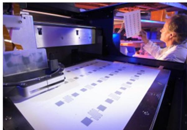
Figure 1.9 Inkjet printer using Clevios™ ink [Reproduced with permission from Heraeus]
