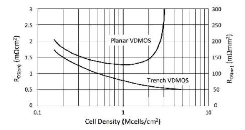
Figure 12: Impact of cell density on  $R_{DS(on)}$ . Planar VDMOS exhibits a minimum while trench VDMOS benefits from scaling [Wil17].
