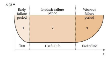
Figure 15: Bathtub curve of failure rate.
