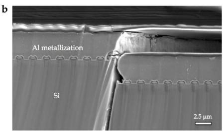
Figure 112: (a) SEM cross-sectional imaging of the naked metallization between the two bonding wire of the 70 °C aged module, showing different types of cracks: fatigue cracks in the metallization layer and fragile cracks in the Si substrate; (b) at higher magnification, the Al top metallization continuity results abruptly compromised as result of the crack propagation in the Si substrate until the surface.
