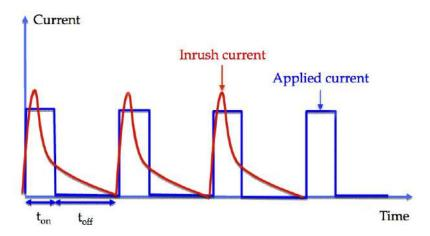
Figure 26: IOL (Intermittent Operating Life) test: the device undergoes electrical pulses during the time interval  $t_{on}$ . The test current and  $t_{on}$  values are generally limited by the control die, that protects the control die from "bulb inrush" phenomena.
