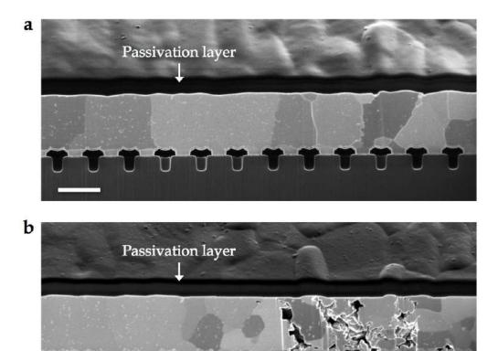
Figure 94: SIM image of the Al top metallization coated by  $SiO_2$  passivation from two close cross-sections in a  $70^{\circ}C$  aged module.
