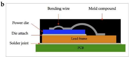
Figure 13: (a) Power MOSFET device from NXP Semiconductors for low voltage applications. (b) Schematic representation of the cross-section of the power MOSFET. The lead frame, made out of Cu, serves as heat sink and is directly soldered on the PCB. The bonding wires are cold welded on the Al top metallization by ultrasonic process. The device is encapsulated in a plastic mold compound.
