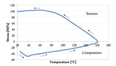
Figure 124: Stress-temperature plot for a 20-160  $^{\circ}$ C temperature cycle performed on a naked SPDo6 die. The stress is directly deduced from the die curvature (measured by laser reflectometry - see Appendix B ) using the Stoney equation (chapter 2, section 2.2.2).
