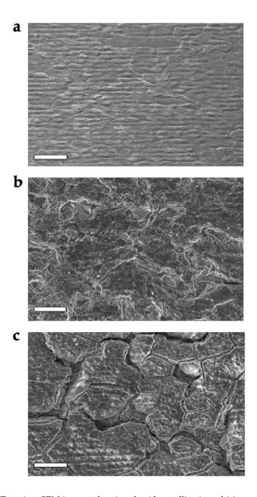
Figure 75: Top view SEM images showing the Al metallization of (a) an as-is module and (b), (c ) a failed one at two different locations. The grain structure is visible in all of them as GBs are slightly grooved in (a) and more heavily cracked in (b) and (c). Scale bar 10  $\mu$ m.
