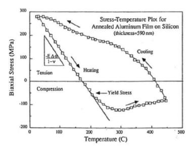
Figure 137: Typical stress-temperature cycle for a 590 nm thick poly-crystalline Al film on oxidized Si substrate ( $T_{max} \sim 450^{\circ}$ C) [Fli87].
