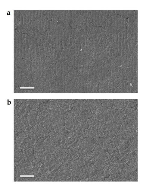
Figure 89: SEM images of the Al metallization close to the bonging wire in a (a)  $25^{\circ}C$  aged module (failed after 5.3 million cycles) and in a (b)  $70^{\circ}C$  aged one (failed after 300 kcycles). Scale bar 10  $\mu m$
