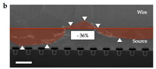
Figure 103: SIM images of the wire-metallization interface in two close areas under the same bonding wire. The images refer to a non-aged module. The red straight line represents the initial metallization surface. White arrows show how the interface moved from this initial position after wire bonding. Scale bar 2.5  $\mu m$ .
