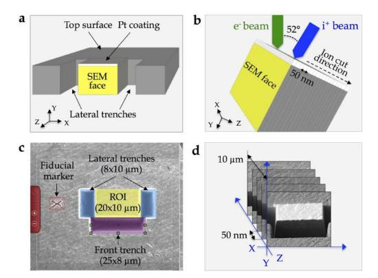
Figure 57: Schematic illustration of the serial sectioning procedure by dual-beam FIB: (a) front view and (b) lateral view of the  $52^{\circ}$  tilted sample inside the FIB chamber. (c) Slice and View FEI software interface for the preliminary trenching preparation. (d) Stack of SEM images with a z-spacing of 50 nm, through 10  $\mu$ m (200 images in total).
