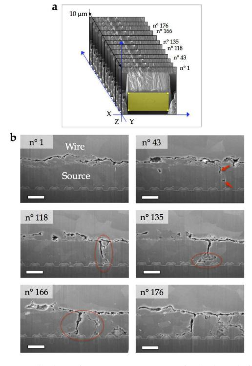
Figure 100: (b) Selection of six non consecutive SEM images from the data stack of the wire-metallization interface (according to the schema in (a)) of a 70  $^{\circ}\text{C}$  aged device (slicing distance 50 nm). The yellow rectangle in (a) represents the milled imaging face. Scale bar 2.5  $\mu m$ .
