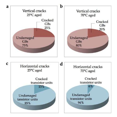
Figure 95: Ratio of cracked vs undamaged GBs in (a) a  $25^{\circ}$ C aged module and in a (b) 70 °C aged one.
