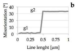
Figure 97: (a) ACOM map of the wire-metal interface of an as-processed module. (b) Misorientation between the grains 1 and 2 along the white dashed line respectively in (a). The standard stereographic triangle gives the color codes of the grain orientations, taken here along the horizontal direction.
