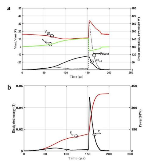
Figure 30: (a) Typical signals during a short cycle event in the power MOSFET by activation of overload protection. (b) Dissipated energy (E) and power (P) during the SC phase.
