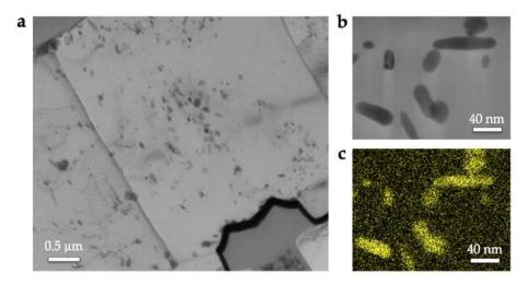
Figure 72: (a) TEM image of the Al metallization decorated with Cu/W precipitates. (b) Higher magnification TEM image of some of these precipitates and (c) relative EDX map, corresponding to the Cu element.
