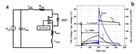
Figure 32: (a) Normal protection mode circuit and (b) waveforms,  $V_{SUP}=30V$ ,  $T_{ON}=200\mu s$ ,  $T_{AMB}=25^{\circ}C$ .
