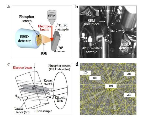
Figure 43: (a) SEM-based EBSD schema and (b) Helios microscope chamber configuration during an EBSD experiment. (c) Kikuchi lines formation schema. (d) Pattern recognition by AZtecHKL
