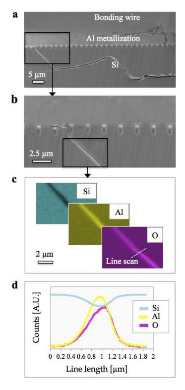
Figure 111: (a) Low and (b) high magnification SEM image of the cracked Si bulk under the bonding contact. (c) EDX mapping of the crack in the Si bulk and (d) relative line scan plot showing the element distribution along the dashed line in (c).
