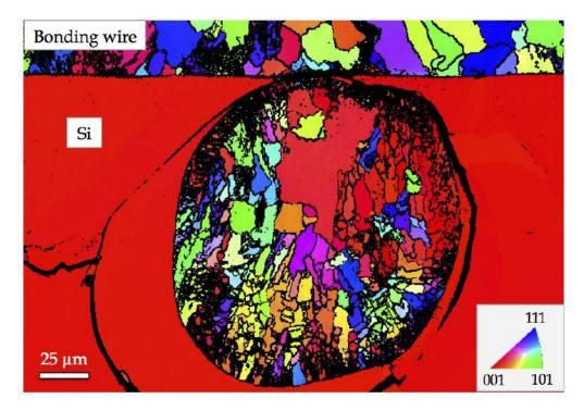
Figure 116: EBSD map of the melted area at the wire-metal cross-sectional interface from a 25  $^{\circ}$ C aged module. The standard stereographic triangle gives the color codes of the grain orientations, taken here along the horizontal direction.
