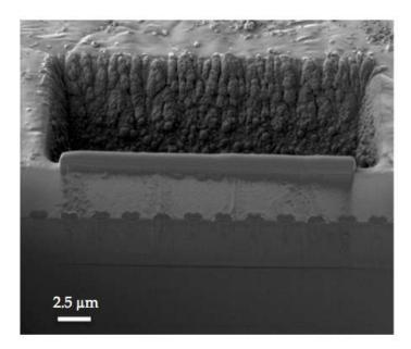
Figure 63: SEM image of the step 2: preparation of a  $\sim$  2  $\mu$ m thick lamella, by removing matter behind the region of interest.
