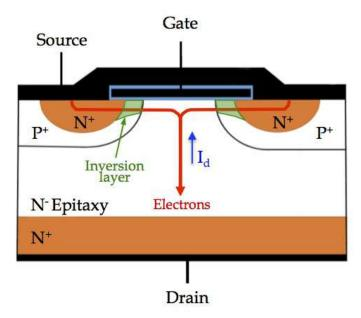
Figure 10: Schema of a VDMOS.
