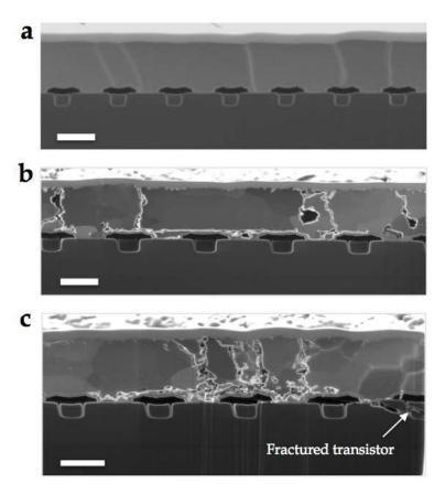
Figure 90: SIM images of the naked metallization cross-sections of (a) as-is, (b)  $70^{\circ}$ C aged and (c)  $25^{\circ}$ C aged power modules. The top layer (~ 1 $\mu$ m thick) is the Pt protective coating to prevent curtaining artefacts on the imaging faces. Scale bar 2.5  $\mu$ m.
