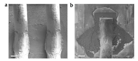
Figure 118: Burnout spots detected after failure (a) between two bond wires in a SPDo6 module and (b) at the bonding connection in a To7D17 module. Scale bar: 250µm.
