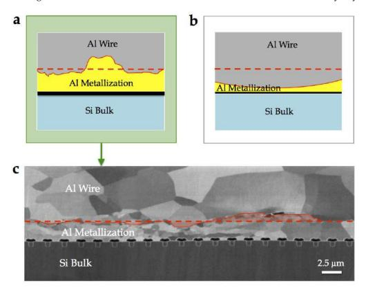
Figure 133: (a) Schema of the wire-metallization interface corresponding to (a) a uniform and (b) non uniform bonding stress along the interface. (c) SEM image of the uneven wire-metallization interface of a LFET1T power device, according to the schema in (a).
