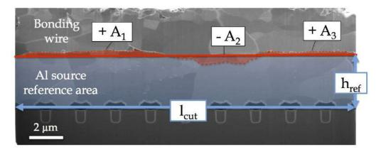
Figure 102: Schematic illustration of the area-based measurement method of the plastic deformation imposed to the Al source metallization by the bonding process.  $h_{ref}$  = initial metallization thickness,  $h_{ref}$  = image width.
