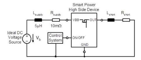
Figure 29: Accelerated aging test circuit.
