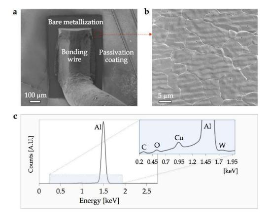
Figure 42: (a) SEM image of an Al bond wire welded on the Al source metallization. (b) At higher magnification, bare metallization of a reference module. (c) EDX spectrum from the Al metallization.
