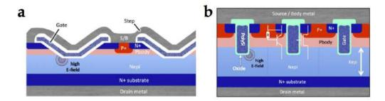
Figure 11: Cross section of (a) a v-groove VDMOS (or VMOS) and (b) of a trench gate vertical MOSFET (or trench VDMOS) [Wil17].
