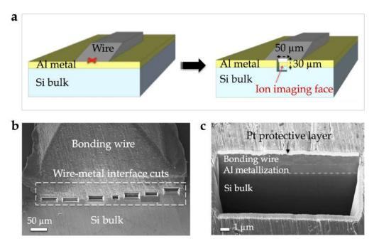
Figure 51: (a) Schematic representation of FIB cross-section from a region of interest (red cross) of the power die wire-metal interface. (b) SEM image of FIB cuts along the wire-metal interface and (c) higher magnification of a single cut, showing the layered structure: Al bonding wire, Al top metallizaiton, MOSFET area and Si substrate.
