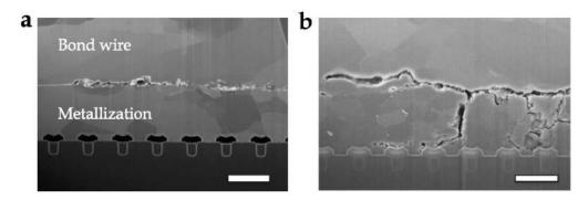
Figure 134: Wire-metallization interface (a) before and (b) after aging (at  $70^{\circ}$ C). The Al-Al interface of as-processed modules presents initial imperfections, consisting in small cavities and native Al oxide residues. During aging, cracks propagate along these imperfections, causing a reduced contact between the wire and the metallization. Scale bar  $2.5\mu m$
