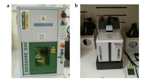
Figure 40: Equipment used for the decapsulation semiconductor devices. (a) IR laser decapsulation system. (b) Pressurized jet system.
