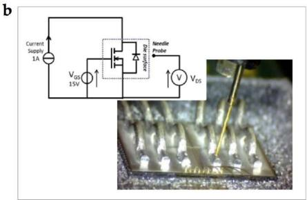
Figure 37: (a) Experimental set-up for source potential mapping of the power die. (b) Spring probe for source potential mapping,  $V_{GS}=15V$ ,  $I_{DS}=1A$ .
