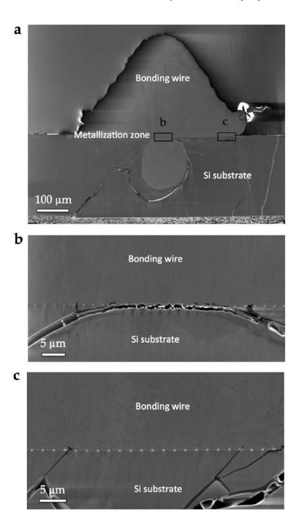
Figure 114: (a) SEM cross-sectional imaging of the bonding wire from an aged power module (25 °C aged) showing different types of cracks; (b), (c) higher magnification images of the wire- metallization interface located in the boxes (b) and (c) in (a). The die crack resulted from an electro-thermal event occurring at failure time.
