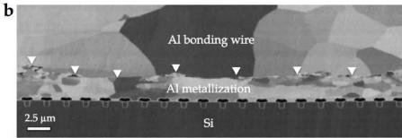
Figure 132: High magnification SIM image of the (a) non-bonded region and (b) the welded one, showing that no Al-Al interdiffusion between the two metallic parts occurred during the bonding process.
