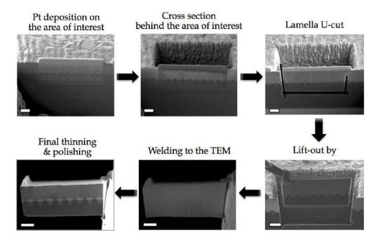
Figure 67: Summary of a FIB lamella preparation for the TEM inspection of the device top Al metallization. Scale bar 2.5 µm.
