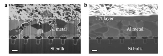
Figure 48: Cross-sectional SEM images of the Al metallization in an aged modules (a) without and (b) with Pt protective layer. Scale bar 1  $\mu$ m.
