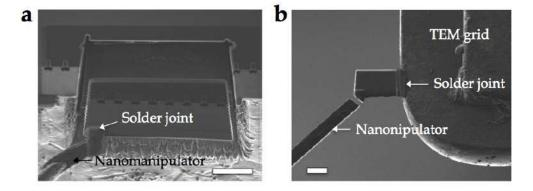
Figure 65: FIB images of the step 4: (a) lamella lift-out and (b) lamella bonding to the TEM grid. Scale bar 5  $\mu m.$
