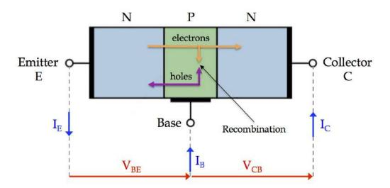
Figure 3: Bipolar transistor general structure.
