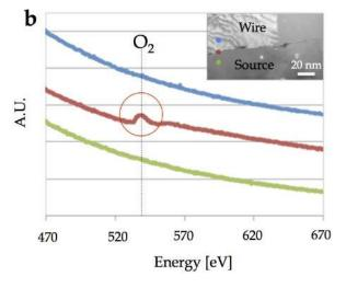
Figure 99: (a) SIM image of the initial artifacts which characterize the wire-metallization bonding of an as-is module. (b) EELS spectra from the wire (in blue), the metallization (in green) and the wire-metallization interface (in red). The red spectrum at the wire-metallization interface reveals the presence of oxygen.
