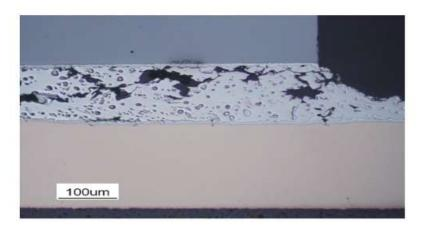
Figure 17: Delamination of a lead-free solder joint between the die Si substrate and the Cu lead frame [Bouo8].
