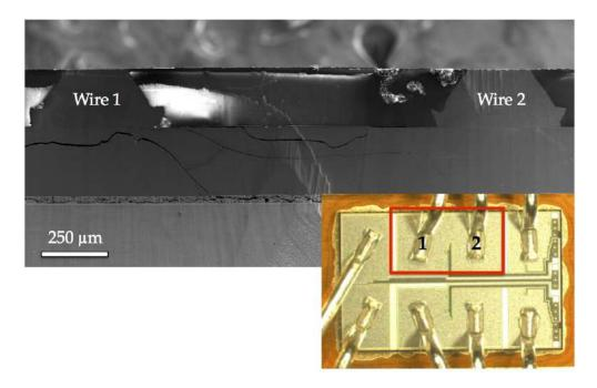
Figure 109: SEM overview of a 70°C aged module prepared by CP for the SEM/SIM inspection. In the insert, optical image image of the To7D17 device, showing the position in the aged module (in red) of wire 1 and 2 under investigation
