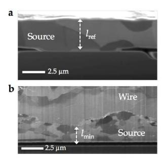
Figure 84: SIM images of the Al metallization (a) away and (b) under the bonding wire. The naked metal thickness ( $l_{ref}$ ) serves as reference for the measurement of the minimum thickness ( $l_{min}$ ) in the deformed sections under the bonding wires.
