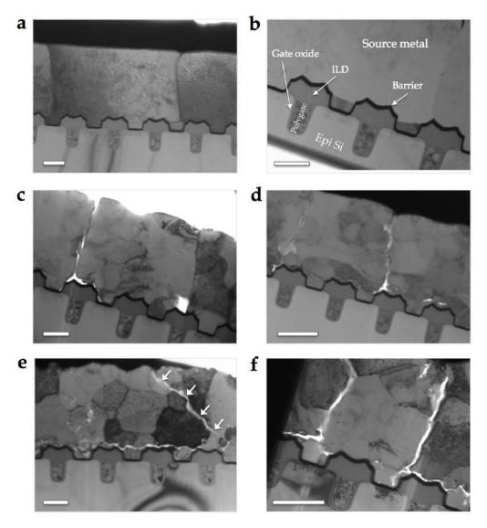
Figure 91: TEM images of some details of the transistor/metallization area from the naked metallization of an (a, b) as-is, (c, d)  $25^{\circ}$ C aged and (e, f) 70/degree C aged power modules. The trench MOSFET layered structure is described in (b) and consists in: source metal, inter-layer dielectric (ILD), gate oxide and polySi (Polygate), epitaxial Si. Scale bar: 1  $\mu$ m.
