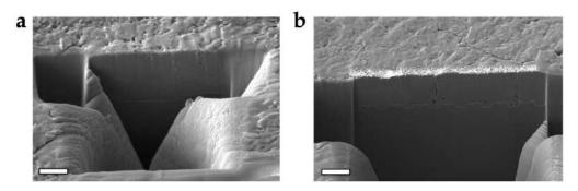
Figure 58: Comparison between two SEM imaging faces during the last steps of the serial milling. (a) The redeposition hides part of the face to be inspected because of a bad preliminary trenching. (b) The imaging face is redeposition-free thanks to an adequate trench size setting. Scale bar 2 µm.
