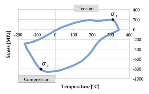
Figure 140: Stress-Temperature cycle for the Al thin film deposited onto the Si wafer. The relative stress is measured along the larger die dimension, and the zero value is here taken at  $350^{\circ}$ C. The cycle is initiated at  $T = -190^{\circ}$ C, and the T gradient is set to  $20^{\circ}$ C/min during heating and cooling.
