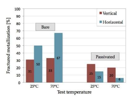
Figure 129: Metallization crack statistics for a To7D17 module aged at 25  $^{\circ}$ C and 70  $^{\circ}$ C, in non passivated –bare– (left) and passivated (right) zones.
