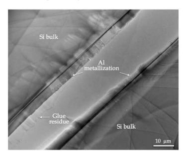
Figure 136: Low magnification TEM image showing the electron transparent cross-section of two bulk-film-film-bulk sandwich prepared by tripod and ion milling.
