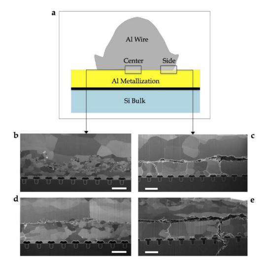
Figure 98: (b) Central and (c) side SIM images of the wire-metallization interface in a  $25^{\circ}C$  aged module. (d) Central and (e) side SIM images of the wire-metallization interface in a  $70^{\circ}C$  aged module. The images correspond to the FIB cross-section locations ("center" and "side") in the schema in (a). Scale bar  $2.5~\mu m$ .
