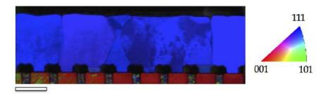
Figure 8o: ACOM mapping of the cross-section of an as-is module, showing a strong <111> texture of the Al grains along the deposition direction. The standard stereographic triangle gives the color codes of the grain orientations, taken here along the vertical growth direction. Scale bar 2.5  $\mu$ m.
