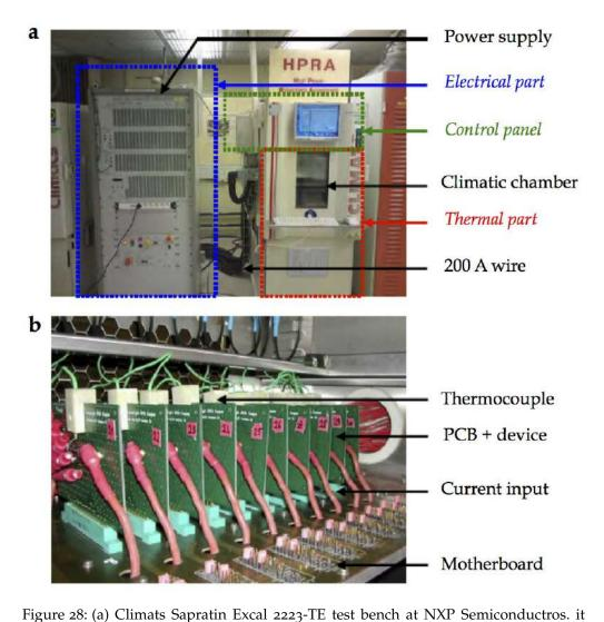
consists in an electrical part (in blue), equipped with a 80 V, 200 A power supply and an active charge (5 - 200 A), a climatic chamber (-80°C - 180°C) containing the devices under test (in red), and a control panel (in green) with an electronic board that control the devices switching.
