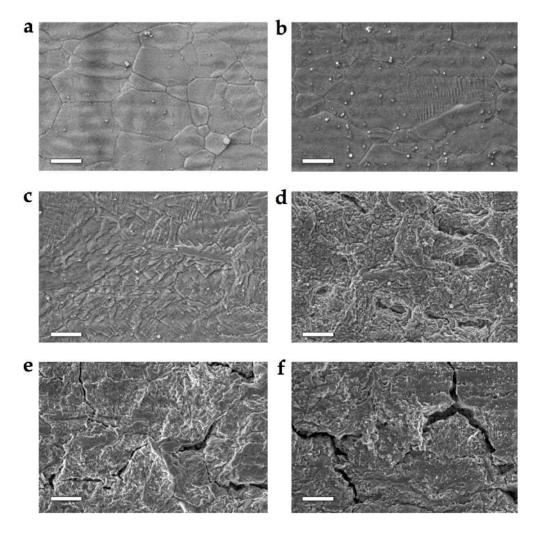
Figure 77: Top view SEM images showing the evolution of the Al source metallization surface. Grain structure (a) before starting the accelerated aging and after (b) 1 kcyles, (c) 10 kcycles, (d) 100 kcycles, (e) 200 kcycles and (f) 300 kcycles. Scale bar 5  $\mu$ m.
