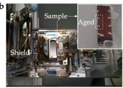
Figure 53: (a) Cross Section Polisher IB-09010CP from JEOL USA. (b) CP inner chamber: the shielding plate is in its lifted position to allow the sample (also visible at higher magnification in the upper-right insert) to be positioned.
