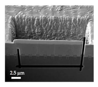
Figure 64: SEM image of the step 3: lamella U-cut prior to the lift-out.
