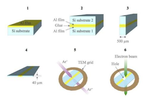
Figure 135: Sketch of the conventional TEM sample preparation procedure.
