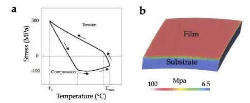
Figure 19: (a) Typical stress-temperature cycle for a 1- $\mu$ m-thick poly-crystalline Al film on oxidized Si substrate ( $T_{m\alpha x} \sim 450^{\circ} C$ ). (b) Finite element simulation showing the Von Mises stresses generated by a temperature change of 50 °C in a 1 cm x 2cm x 0.5 mm specimen (typical size used in wafer curvature) [Lego9].
