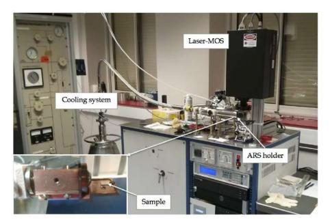
Figure 138: Laser reflectometry test bench assembled for curvature experiments. The sample (reference SPD06, before assembly) is placed under vacuum on a Cu support, inside the ARS sample holder.
