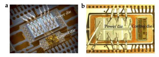
Figure 23: LFET1T smart power MOSFET device from NXP Semiconductors. (a) 45V, 12V SPD06, (b) 65V, 24V T07D17.
