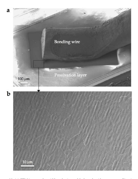
Figure 88: (a) SEM image of an Al bond wire welded on the Al source metallization on an as-is module. Away from the bonding area the metallization is coated by a  $SiO_2$  passivation layer. (b) Higher magnification of the bare metallization close to the bonding wire.
