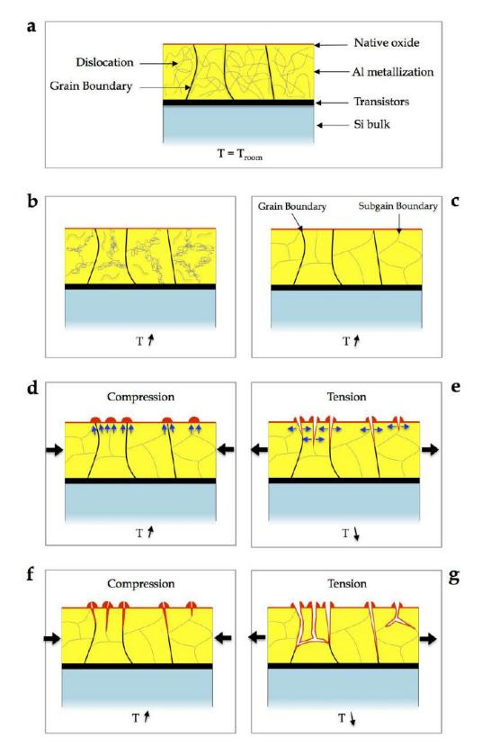
Figure 125: Gao's model extended to Al layers undergoing tension and compression stresses during thermal cycles [Mar14]. (a-c) The dislocation density decreases by recombination in sub grain boundaries and absorption at GB interfaces. (d-g) Al diffusion along grain boundaries, and subsequent oxidation causing crack propagation through the Al layer.
