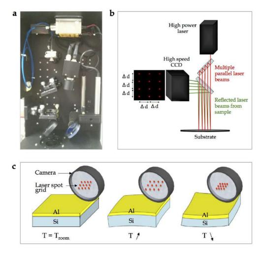
Figure 139: (a) MOS K-space module interior and (b) laser operating principle. (c) The larger CTE of the Al film compared to the Si substrate induces elastic and plastic strains in the film. The Al film is then stressed in compression during the heating phase and in tension upon cooling.
