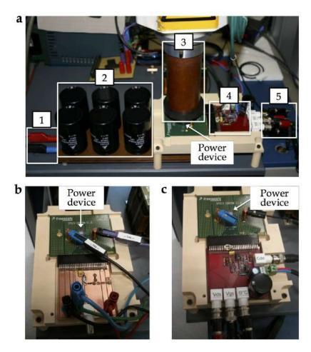
Figure 31: (a) Accelerated aging test bench set up at the Satie laboratory. The device under test can be connected to (b) a measuring board or to (c) the driving board.
