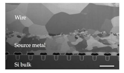
Figure 96: SIM images of the wire-source metallization interface, at the center of the bonding wire, in an as-processed module. Scale bar  $2.5 \mu m$ .
