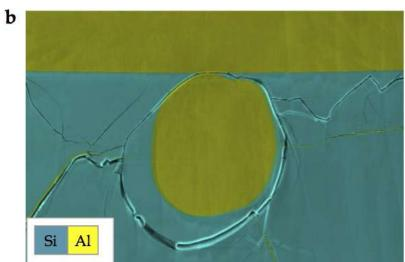
Figure 115: (a) SEM cross-sectional imaging of the round shape feature in the Si substrate (Al contrasted like) from an aged power module (25 °C aged); in (b) the corresponding EDX maps of the Si (in light blue) and Al (in yellow) are overlapped, showing that the round shape feature in the Si substrate is made out of Al. This has probably diffused from the top wire during the short-circuit event, because of the local melting of the metallic parts at high temperature.
