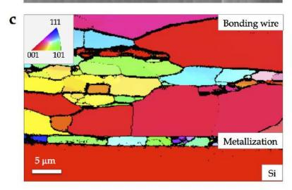
Figure 117: (a) SEM cross-sectional imaging of the wire-metallization interface pointed by the white arrows, (a) at the center and (b) at the extremity of the bonding area. (c) Relative EBSD map of the wire-metallization-semiconductor layered structure. The standard stereographic triangle gives the color codes of the grain orientations, taken here along the horizontal direction.
