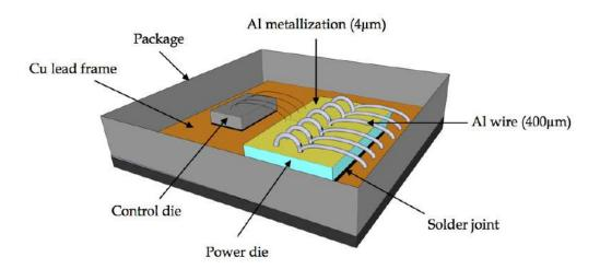
Figure 16: Schematic representation of a LFET1T-like smart MOSFET power device.
