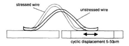
Figure 20: Bonding wire subjected to cyclic mechanical stress applied by lateral displacement of one bonding area relatively to the other in Ramminger et al. experiments [Ramoo].
