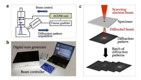
Figure 70: Automated Crystal Orientation Mapping (ACOM).
