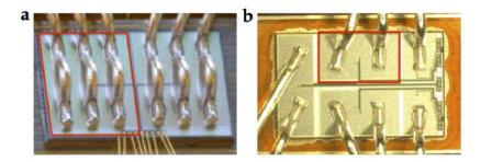
Figure 27: Localization of the MOSFET sector under accelerated aging test (red rectangle) in a (a) LFET1T 45V (SPD06) and (b) LFET1T 65V (T07D17) power device.
