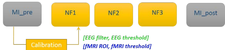
Figure 45 – The experimental protocol consisted of 5 EEG-fMRI runs: a preliminary motor imagery run without NF (MI_pre) used for calibration, three NF runs (NF1, NF2, NF3), and a post motor imagery run without NF (MI_post). Each run consisted of a block design alternating 8 times 20s of rest and 20s of task.
