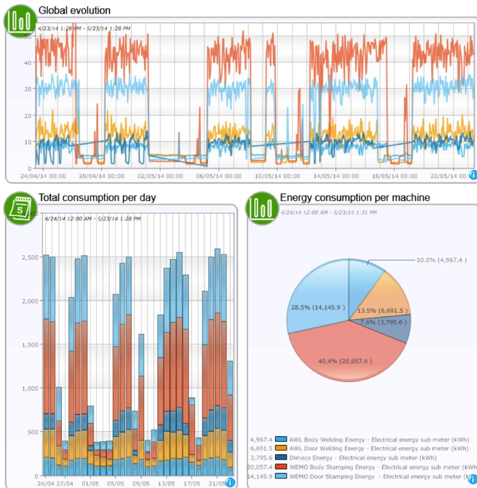
FIGURE 3.3 – Energy Operation dashboard example.
