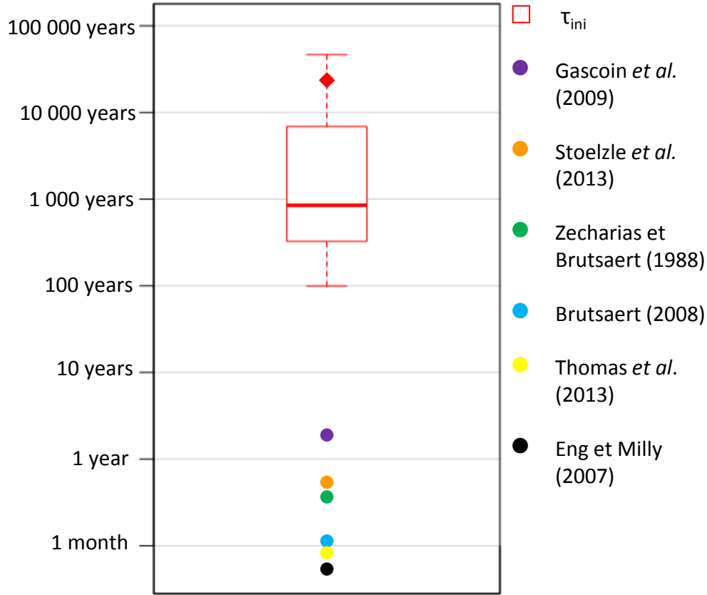
Figure 1.4 – Estimated base flow time constant ( \tau_{ini} ) estimated at 0.5^\circ resolution with HydroSHEDS and GLHYMPS data. The bottom and top of the box-plot represent first and third quartiles, the middle bar gives the median, and red diamond indicates the mean value. Whiskers show the 10th and 90th percentiles. Points represent mean values from the literature for the simple approach (linear reservoir).
