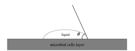
**Fig. 2.2** Schematic illustration of a sessile-drop contact angle system (adapted from Kwok and Neumann (1999)).
