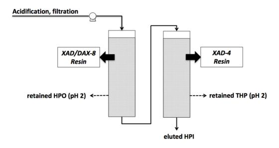
Fig. 2.5 Classical hydrophobic/hydrophilic fractionation by XAD/DAX resins.
