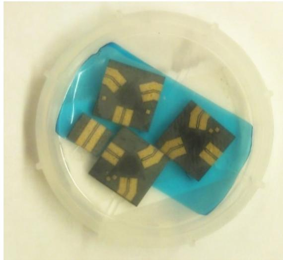
**Figure 4.29:** Prototypes of the ferrite LTCC circulator
