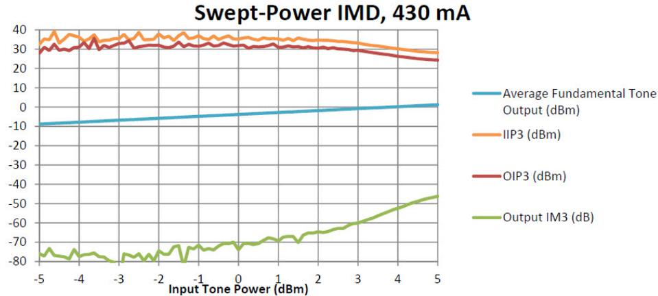
Figure 4.42: Swept-Power IMD Test when current  $I=430$  mA
