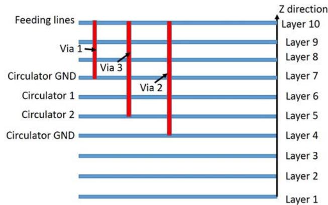
**Figure 4.49b:** Ferrite LTCC layers configuration
