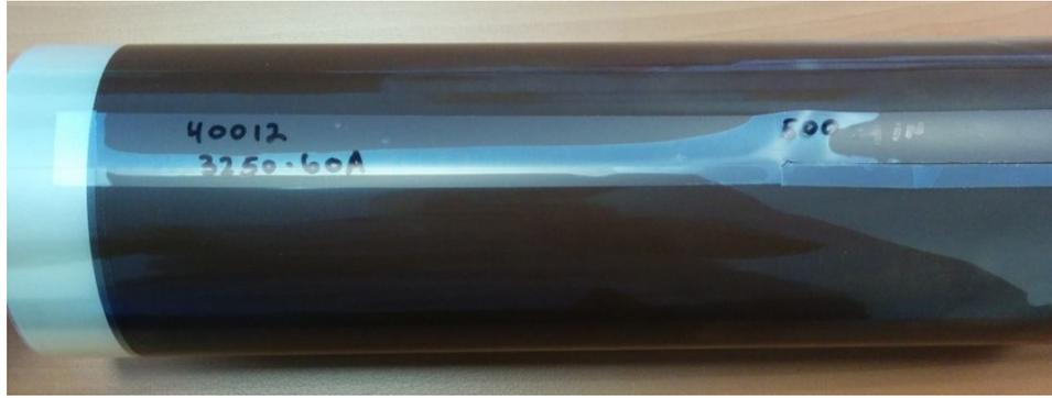
**Figure 3.13:** Photo of ESL 40012 ferrite tape ('green' tape)
