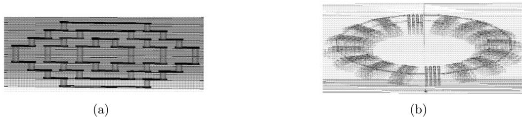
**Figure 3.14:** LTCC (a) solenoid transformer unit cell cross section and (b) toroid transformer tilted front view [15]
