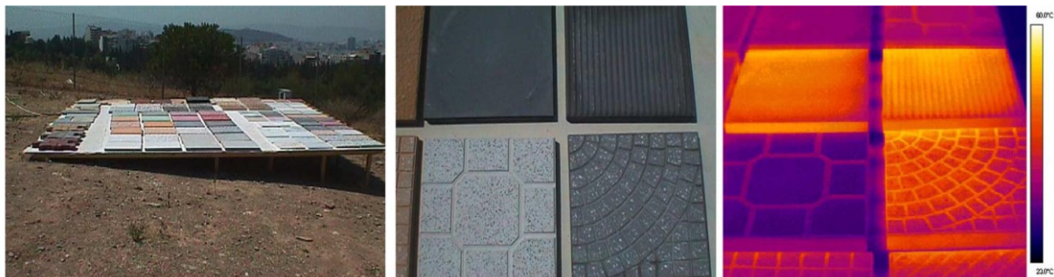
Figure 3. 3: The site of the experimental campaign with the modulated platform | Visible and infrared image of selected building materials
