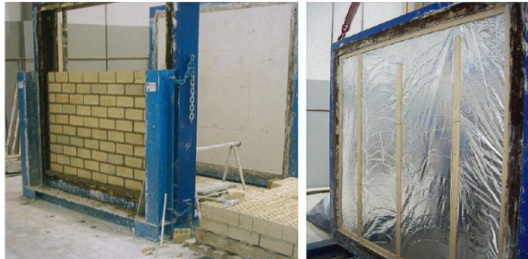
Figure 1. 26: Non insulated wakk and wall insulated with the radiant barrier Source: (Escudero et al., 2013)
