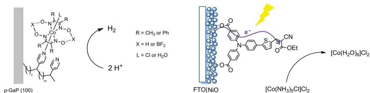
**Figure I.36.** Hybrid inorganic SC-cobaloxime photocathode for HER (left)<sup>139b, 139c, 141</sup> and a push-pull organic dye attached to NiO in a *p*-type photocathode approach (right).<sup>140</sup>
