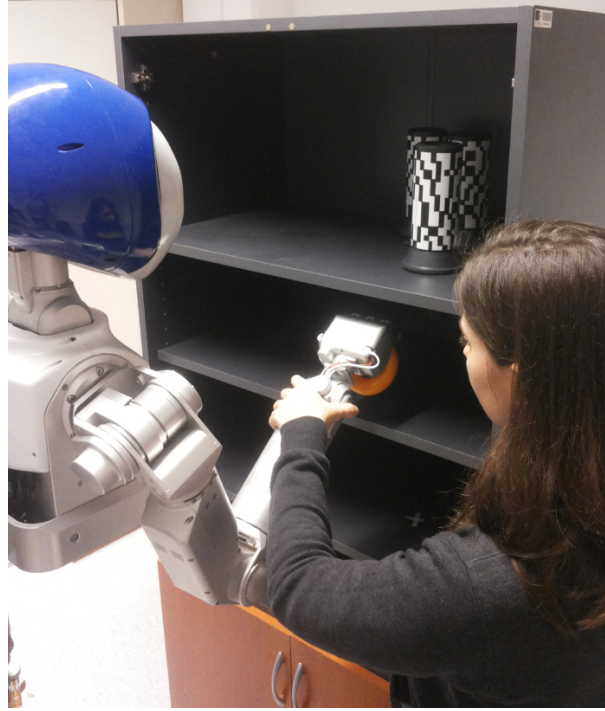
Figure 2.3: Image taken from the experiment conducted with the Meka robot at ENSTA-ParisTech (section 6.1). The task consisted in using virtual guides assistance to facilitate the placement of objects in a cupboard with shelves while avoiding collisions with them. Within the virtual guide formalization, it is important to distinguish between three participators: 1) the human operator, who exerts forces on the robot end-effector 2) the robot 3) the virtual mechanism, which constrains the movement of the robot.
