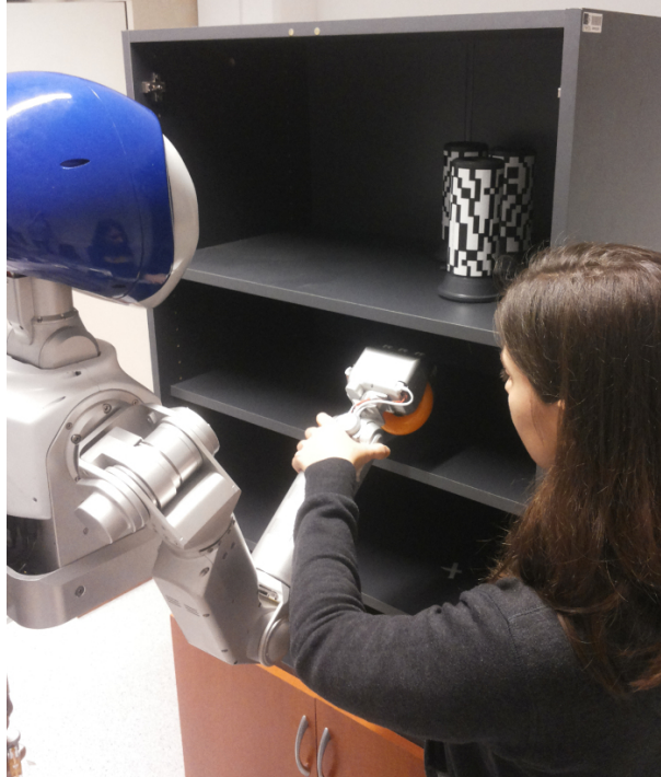
Figure 6.2: The task with meka consisted in using virtual guides assistance to facilitate the placement of objects in a cupboard with shelves.
