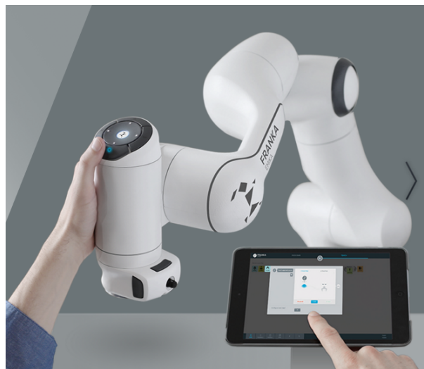
Figure 1.2: Franka robot. In recent years a lot of effort have been made to improve human-machine interaction. New devices such as smart phones, tablets and augmented reality devices make easier to interact with a robot.
