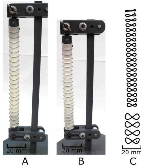
FIGURE 5.4 – Experimental setup inserted in the microtomograph to obtain SG modules geometry in stretched (A) and tension-free (B) configurations. Example of stent centrelines extracted from microtomography scan images (C).
