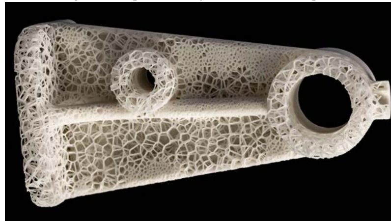
(c) Model printed on a ZCorp 450.
