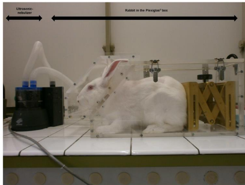
Fig 1. Rabbit exposed to an aerosol administered in a closed Plexiglas box using an ultrasonic-nebulizer (SYST'AM, LS290). The box was conceived to allow the head of the rabbit to be maintained in front of the aerosol particles and drops cloud generated by the nebulizer. Aerosol sessions were performed 15–20 min daily from day 26 to day 28 either with ovalbumin (OVA rabbits) or with saline (control rabbits).
