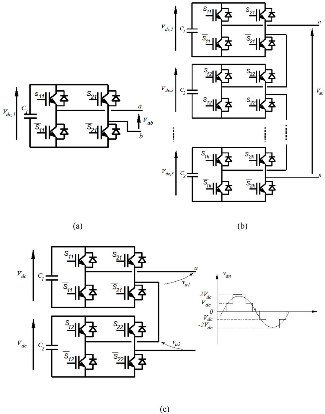
Fig. 1.9: Cascaded H-bridge (CHB) multilevel converter description:
