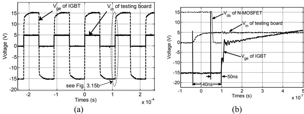
Fig. 3.17.: Validation results for a signal transmission function ( $ep_1 = 0.5mm$ ):
