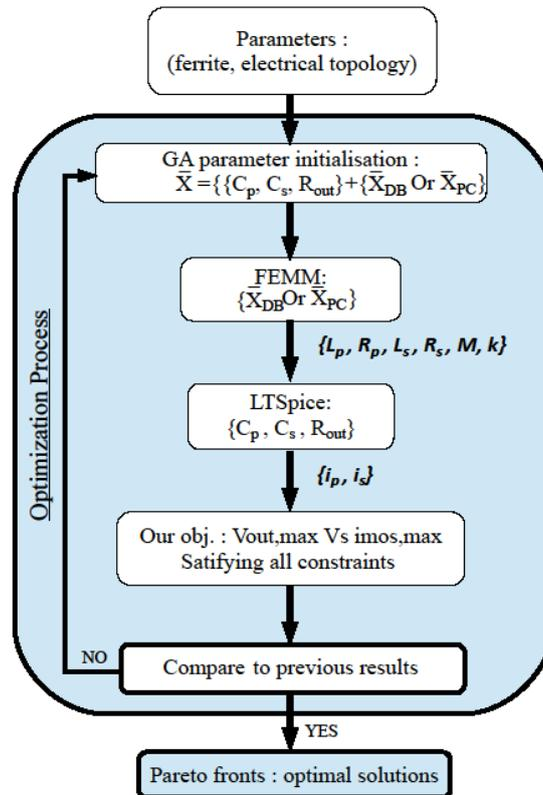
Fig. 2.10.: Genetic algorithm (GA) flowchart for overall system optimization based on FEMM<sup>TM</sup> and LTSpice<sup>TM</sup> softwares.
