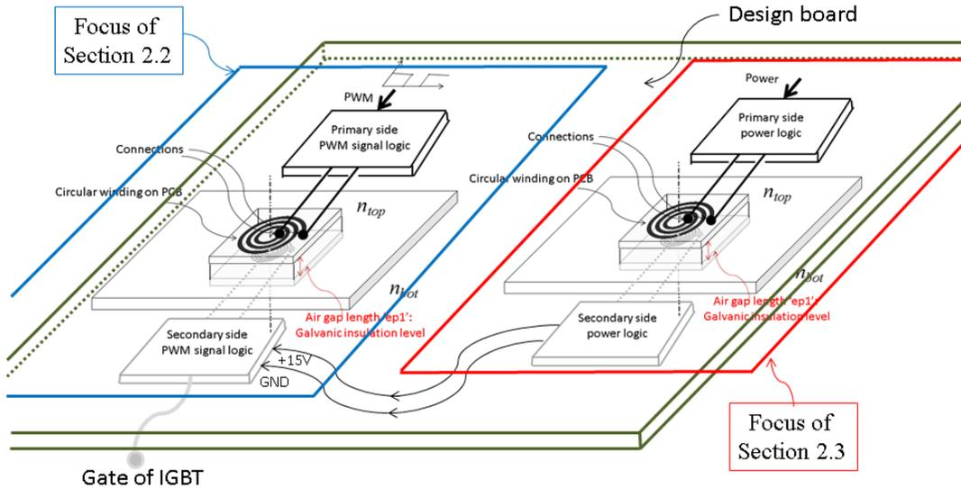
Fig. 2.15.: Example of a design board for a single channel IGBT gate driver: a signal transmission function and a power transmission function with two insulation transformers.
