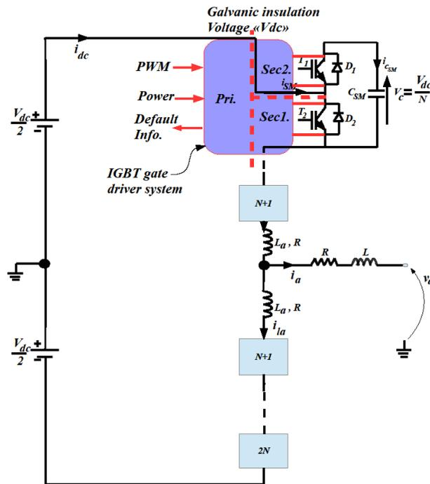
Fig. 1.27: Synopsis of IGBT gate drivers: proposed IGBT gate drivers for one SM with determined galvanic insulation voltage level ( $V_{dc}$ )
