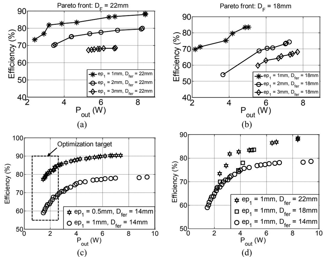
Fig. 2.21.: Optimization results for power transmission IGBT gate drivers:
