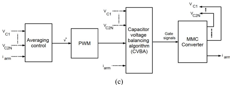
Fig. 1.14: Summarizes of internal control of MMC converter:
