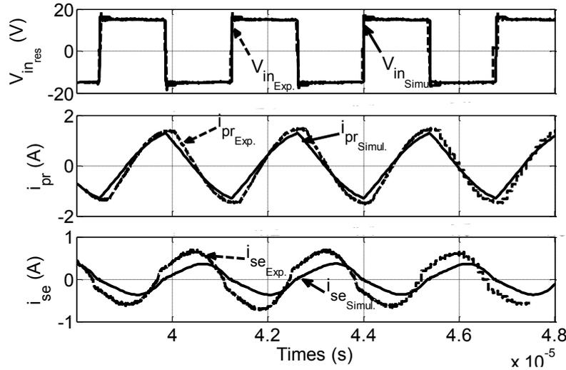
Fig. 3.19.: Validation results for a power transmission function ( $ep_1 = 1mm$ ): the comparison of  $V_{in,power}$ ,  $i_{pr}$  and  $i_{se}$  between the simulation and the experimental results
