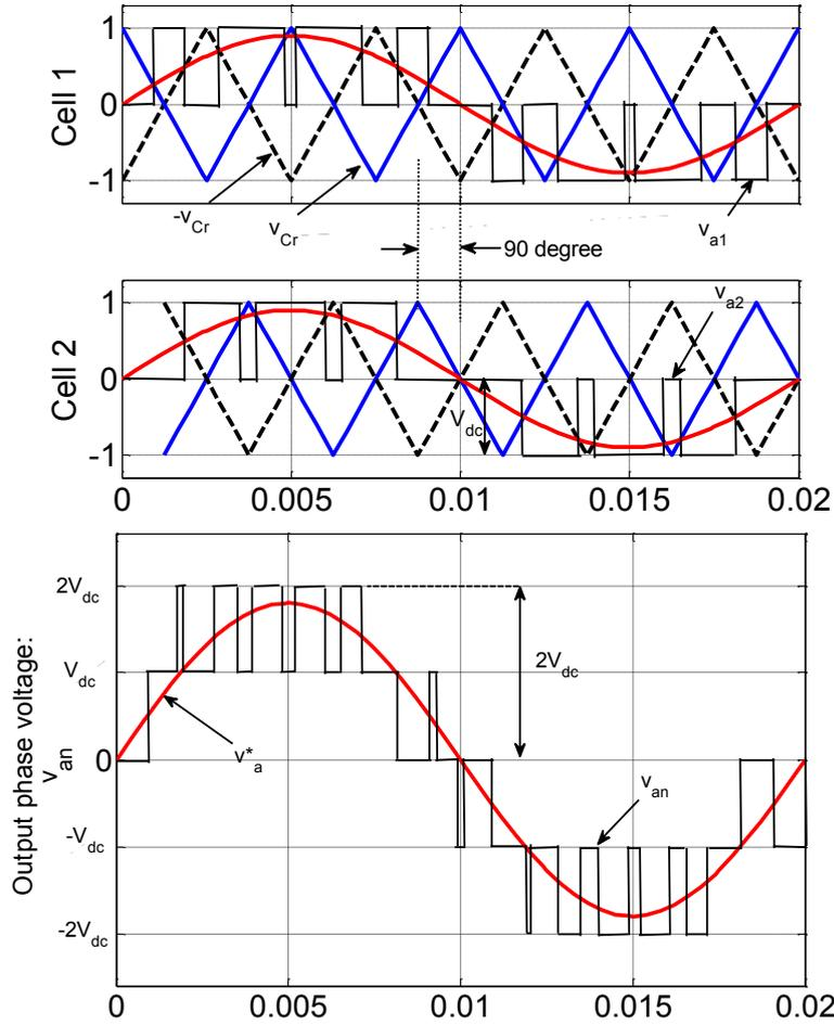
Fig. 1.10: Two-cell five-level CHB (5L-CHB) PS-PWM waveform generation
