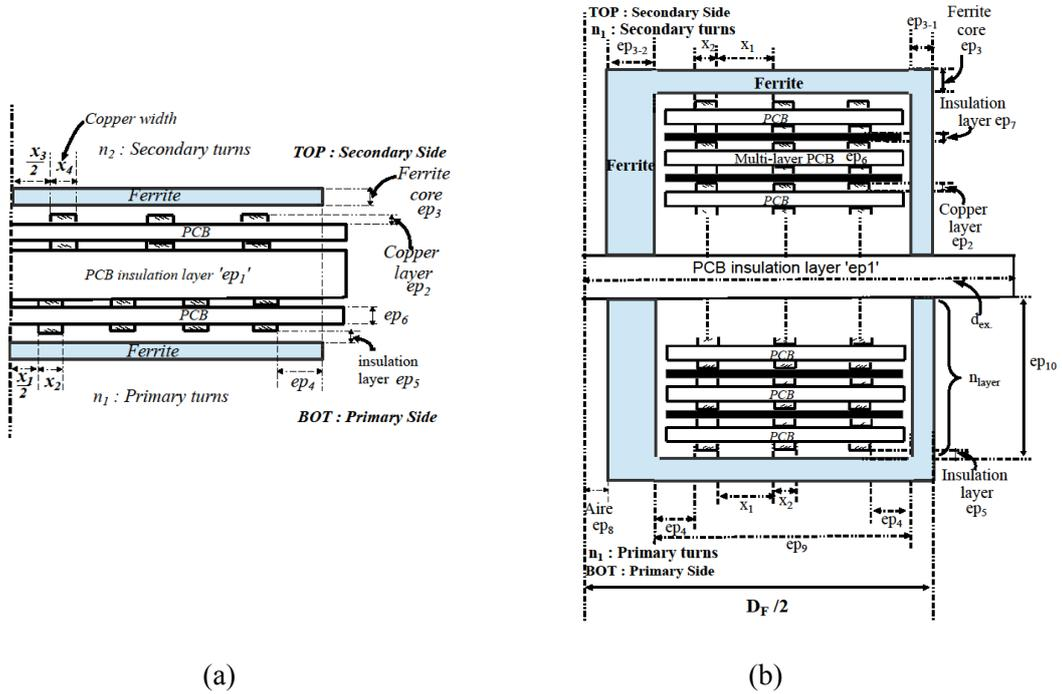
Fig. 2.9.: Transformer geometries:
