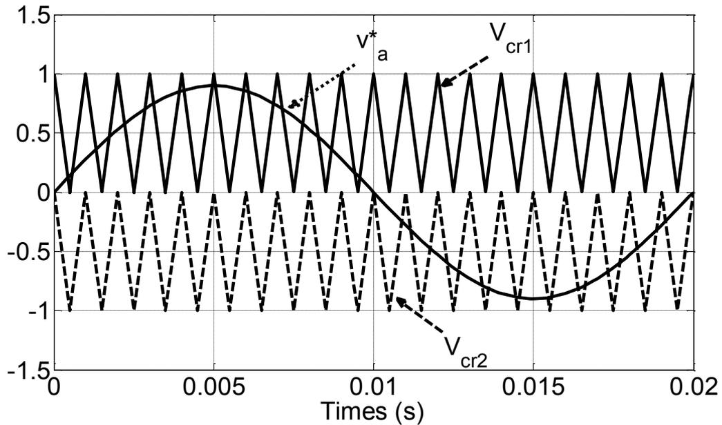
Fig. 1.4: Example of phase-disposition (level-shift) modulation for 3L-NPC converter
