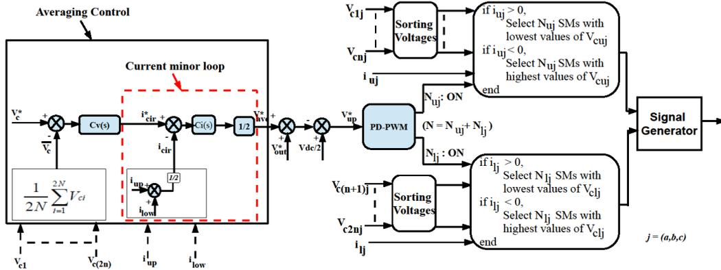
Fig. 1.18: Completed internal control of MMC converter
