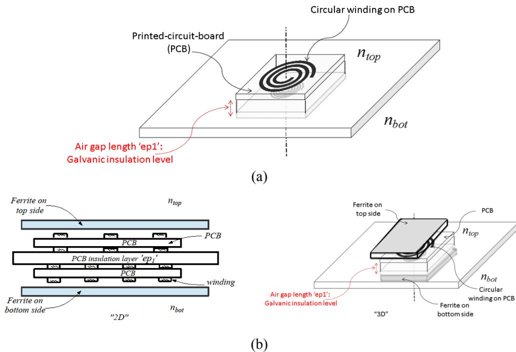
Fig. 2.2.: Compact planar transformer:
