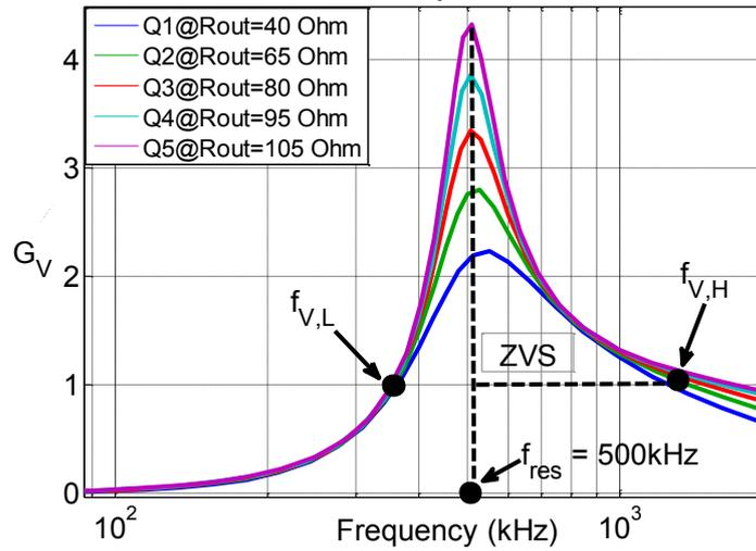
Fig. 2.18.: Magnitude analysis of voltage transfer ratio  $G_v$
