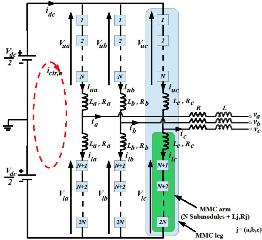
Fig. 1.12: Three-phase modular multilevel converter (3p-MMC)
