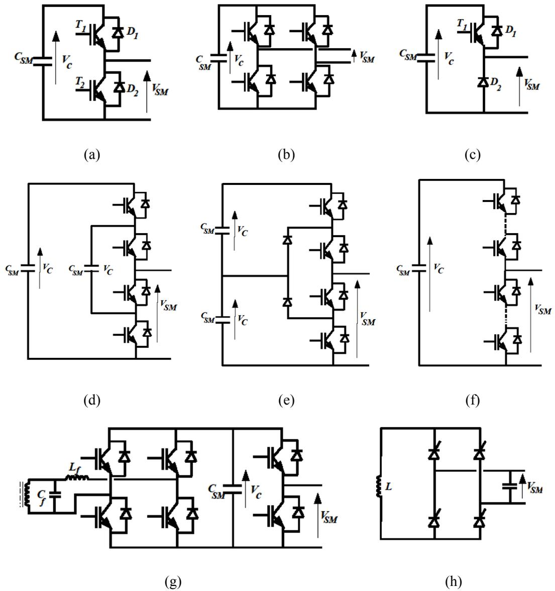
Fig. 1.13: Various sub-module topologies for MMC converter:
