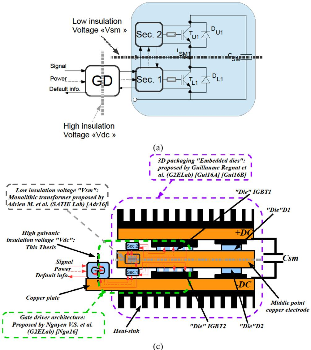
Fig. 3.23: 3D packaging of active power modules for SM:
