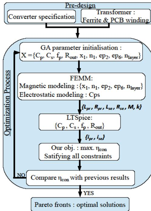
Fig. 2.20.: Optimization flowchart with genetic algorithm (GA) code in a MATLAB<sup>TM</sup> script.
