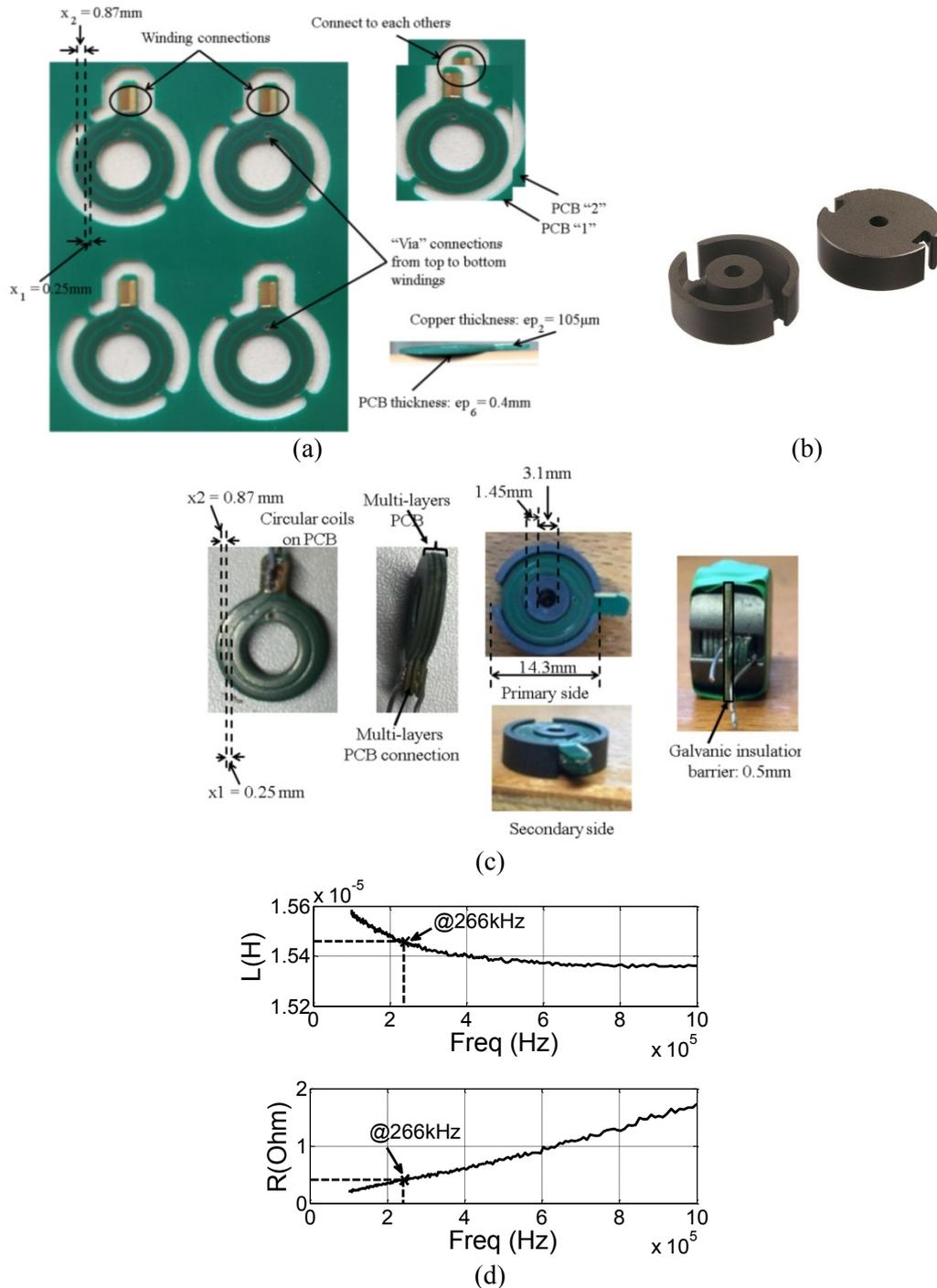
Fig. 3.2.: Optimal pot core planar transformer set up:
