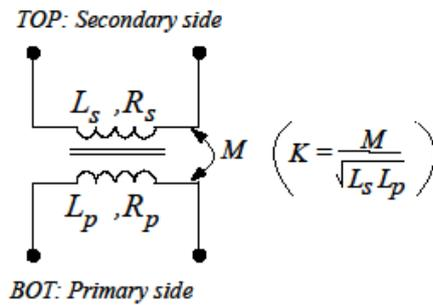
Fig. 2.5.: Pot core transformer modeling considerations:
