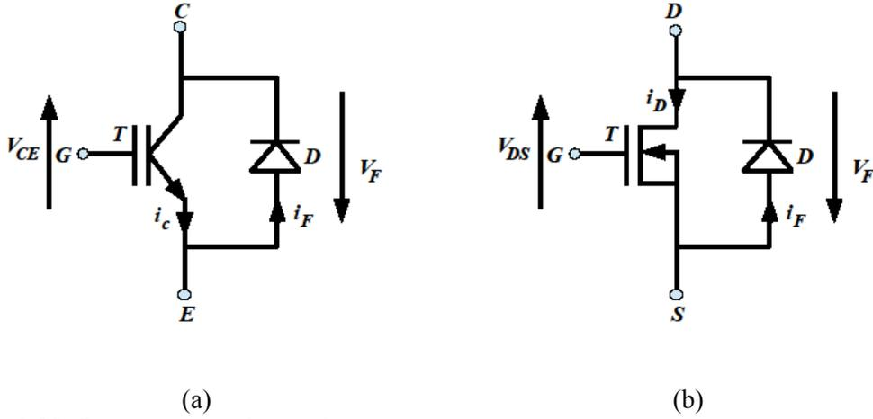
Fig. 1.20: Power semiconductor devices:
