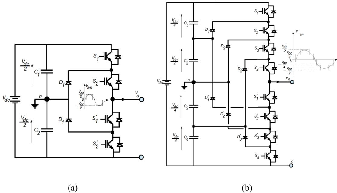
Fig. 1.3: Neutral-point-clamped multilevel converters:
