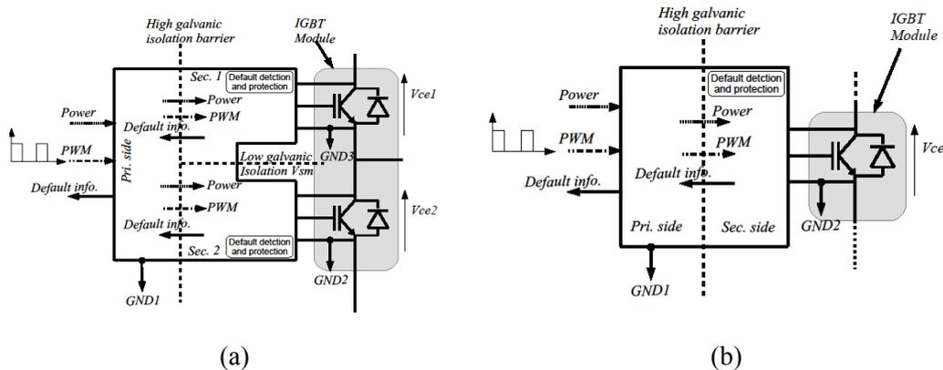
Fig. 2.7.: Synopsis of IGBT gate drivers system:
