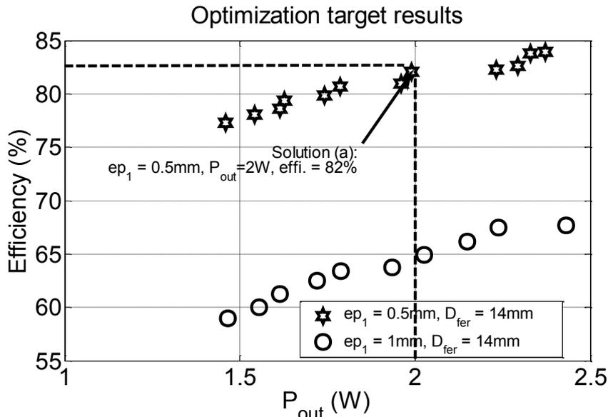
Fig. 3.1: Optimization target results for power transmission
