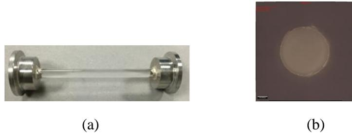
Figure 6.2: (a) Glass microtube glued to KF16 socket flanges;
