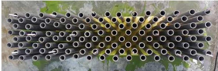
Figure 3: Arrangement of the medium diameter cylinders (viewed from above).
