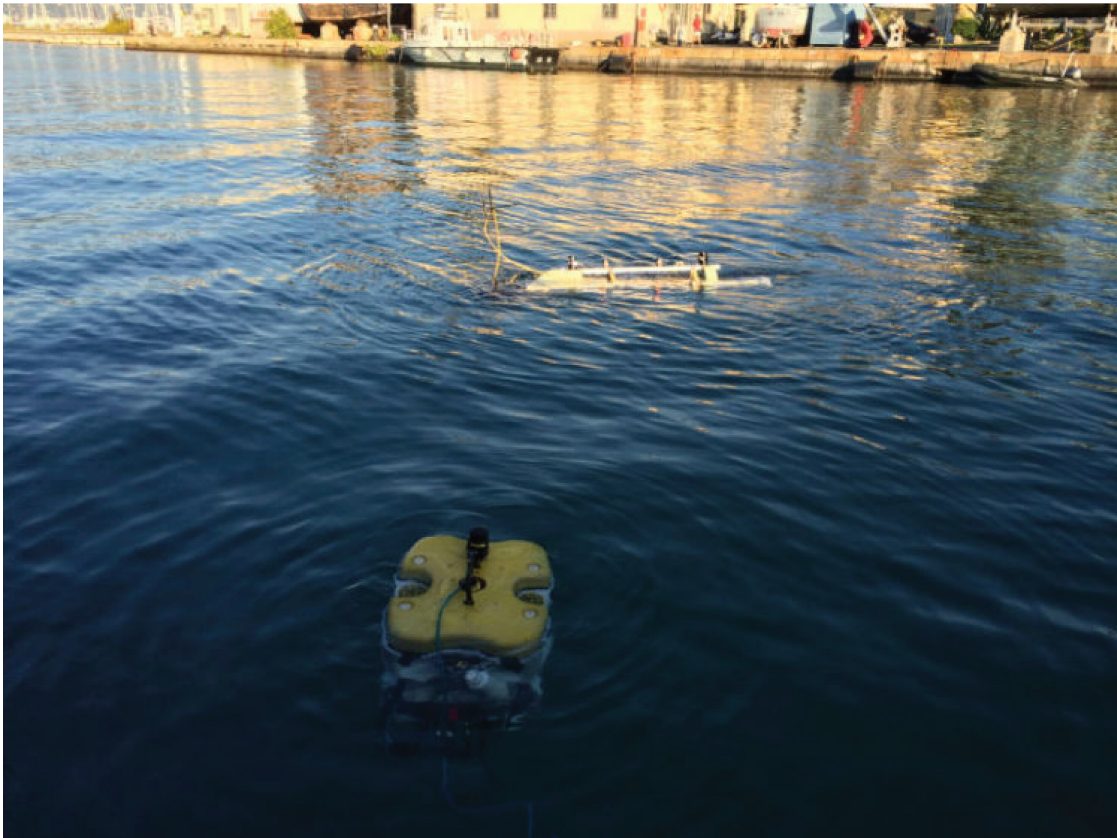
Figure 6-2: An improved AUV version of the CISCREA robot that equipped with fully autonomous sensors, such as sonar, underwater cameras, INS/electro-gyros, depth meter and other self-navigate and control unit
