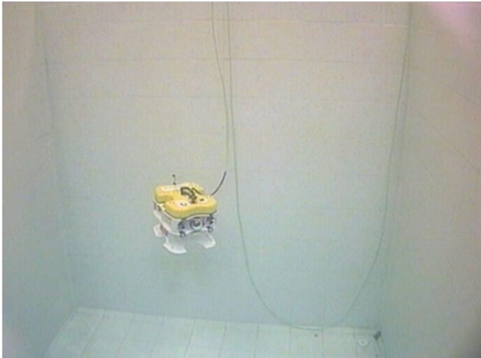
Figure 4-9: CISCREA AUV captured by an underwater camera moving in the heave direction
