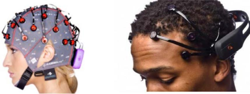
Figure 1.2: Left: g-tec EEG headset, with 32 g.LADYbird active electrodes. Right: Emotiv EPOC low-cost EEG Headset, using dry electrodes <sup>4</sup>
