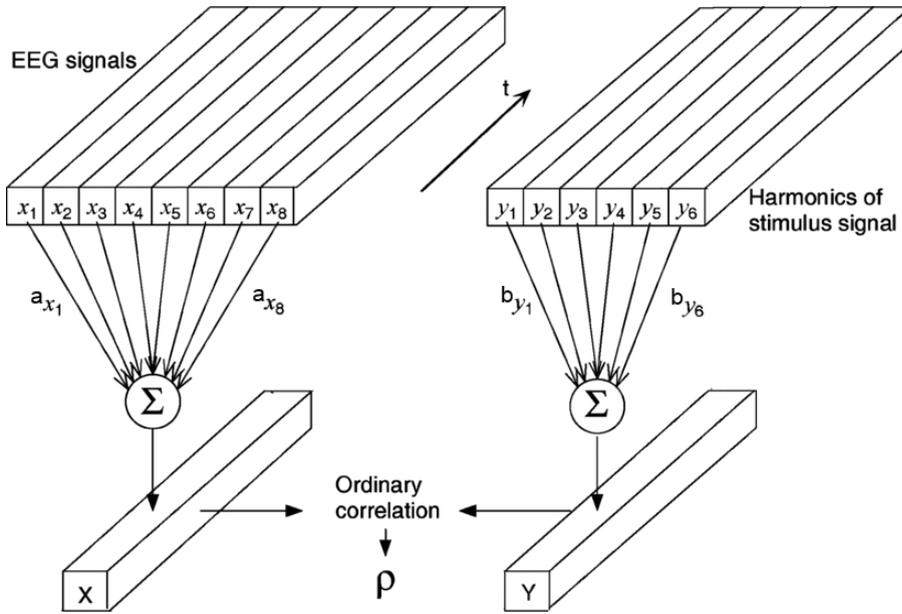
Figure A.1: CCA use for EEG signal analysis [Friman et al., 2001]. The signals  $x_1, x_2$ , etc. is compared to the reference signals  $y_1, y_2$ , etc. (typically the harmonics of the stimulus signal for SSVEP classification), producing a single correlation measure  $p$ .
