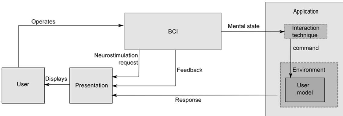
Figure 2.7: **Passive BCI:** The user does not send an explicit command, but the application can construct a model of the user based on his or her mental state
