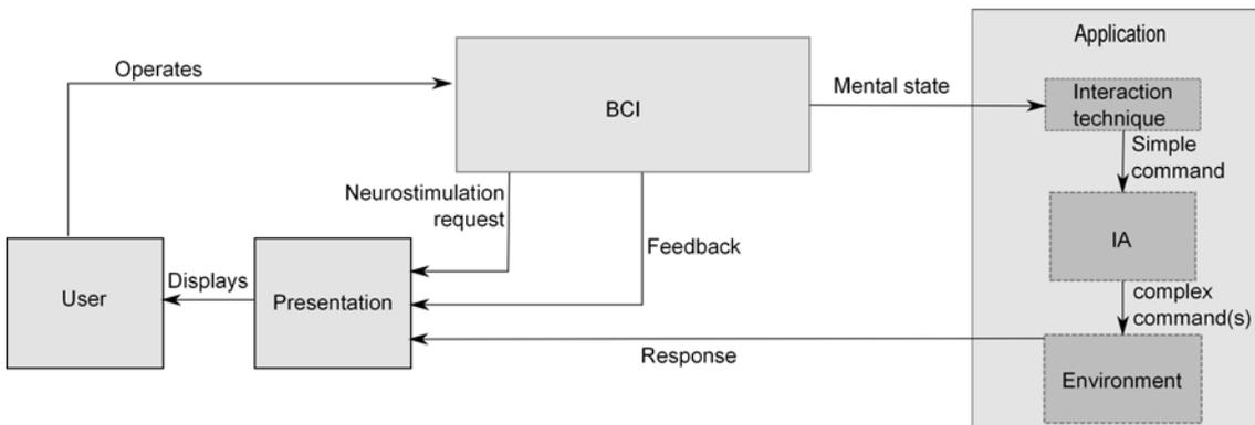
Figure 2.8: **Shared control:** a unique command is analyzed and transformed into a high-level command that may be automatically deconstructed into a series of low-level commands.
