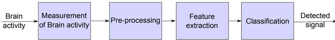
Figure 1.1: General architecture of signal processing for BCIs.
