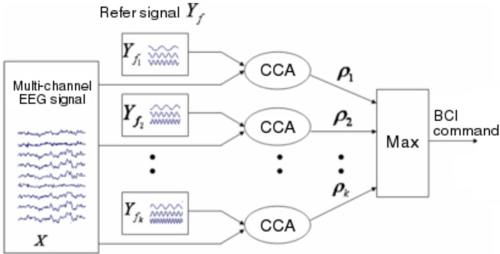
Figure A.2: Description of CCA-based pipeline for segmentation-paced classification, with with  $k$  targets, as described by [Bin et al., 2009]
