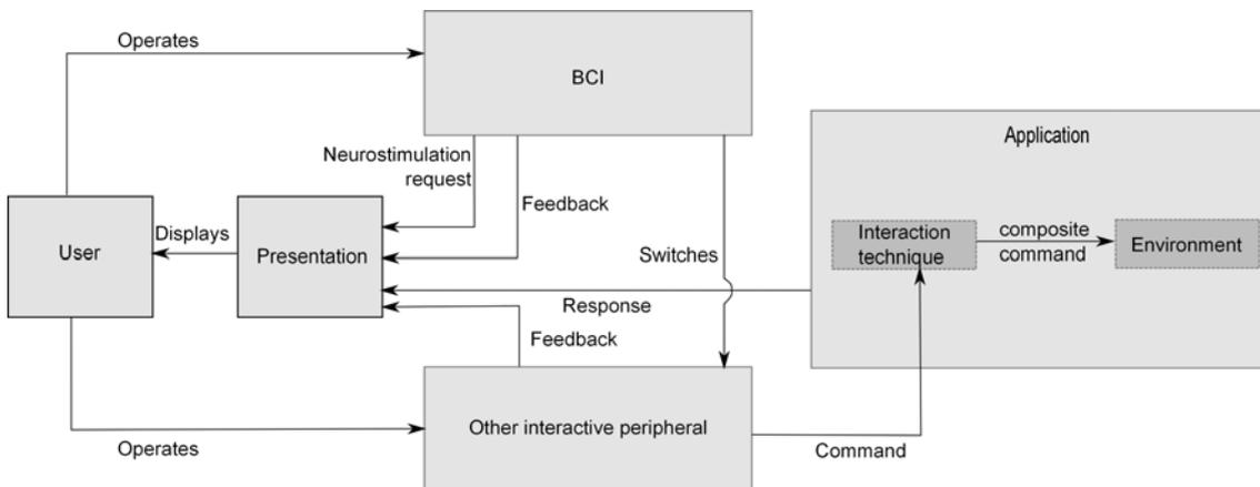
Figure 2.6: **Brain Switch**: The BCI is used to turn ON or OFF another interaction device, possibly another BCI. The same effect can be obtained in a more classical way if the application uses the BCI input to control the other interaction device.
