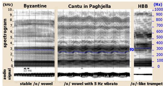
Figure 8 Three vocalic /o/ samples of different style singing voice (Byzantine, Cantu in Paghjella, HBB). Spectrograms (10kHz band in black on the left) and  $f_0$  curves (in blue on the right) are shown in the upper panel, corresponding acoustic waveforms in the lower one.
