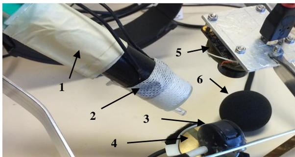
Figure 5 Sensor synchronization experimental setup test. 1) Syringe, 2) Piezo, 3) EGG sensor, 4) US transducer, 5) Camera, 6) Microphone
