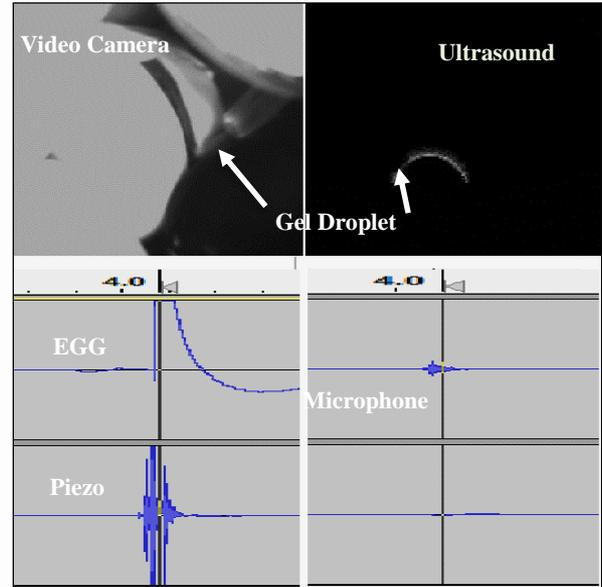
Figure 6 Top left, arrow indicates gel droplet ejected from tip of syringe; top right, arrow indicates arrival point of droplet on ultrasound probe; bottom left and right, time waveforms of EGG, Piezo, and microphone, signals, see discussion in text
