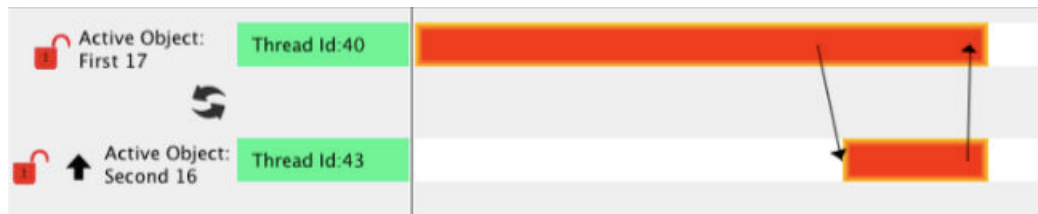
Figure 5.5 – Representation of a deadlock by the debugger tool for multiactive objects.
