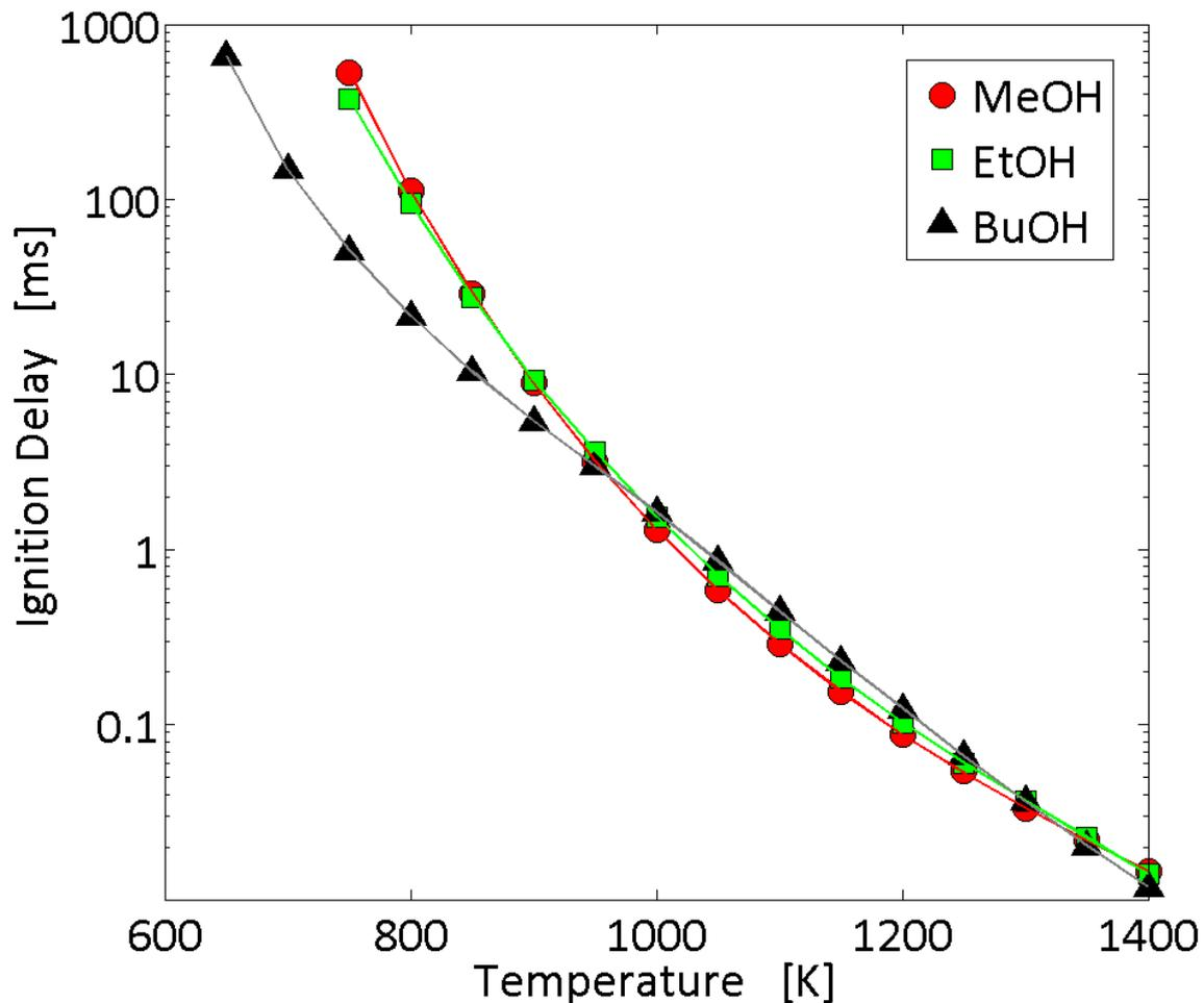
**Figure 116.** Ignition delays computed as a function of the temperature for the three alcohol fuels selected under a pressure of 35 bar and an equivalence ratio of 0.3. Symbols represent the results obtained in the case of the scheme without the ozone sub-mechanism and dashed lines the results with the ozone sub-mechanism.
