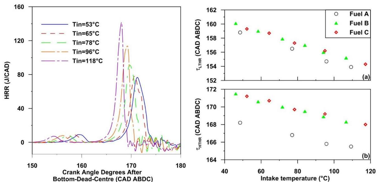
**Figure 19.** Effect of the intake temperature on heat release rate for TRF24 as fuel (on the left) and effect of the intake temperature on combustion timing (on the right). Results on the top correspond to the cool flame and those on the bottom to the main flame. Fuels A, B and C represent *n*-heptane, PRF25 and TRF24, respectively [33].
