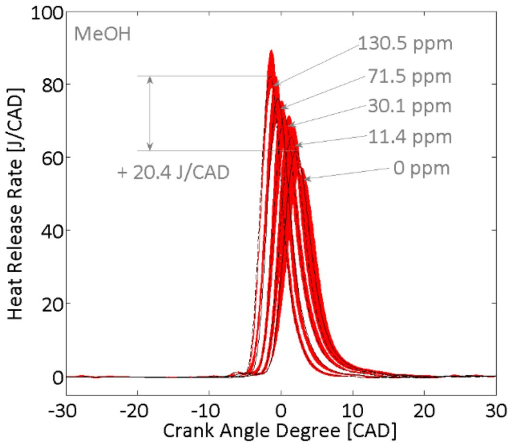
**Figure 110. B.** Heat release rate traces as a function of the ozone seeded for MeOH as fuel. Black curves correspond to the average of 100 cycles recorded and gray areas represent the variation of the same 100 cycles (the upper and the lower limits obtained).
