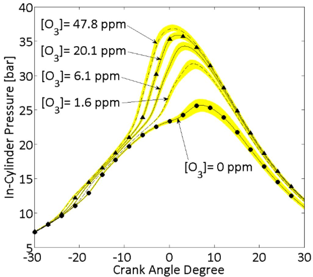
**Figure 51. A.** In-cylinder pressure evolutions as a function of the ozone concentration injected in the intake of the engine for *n*-heptane/PRFO as fuel.
