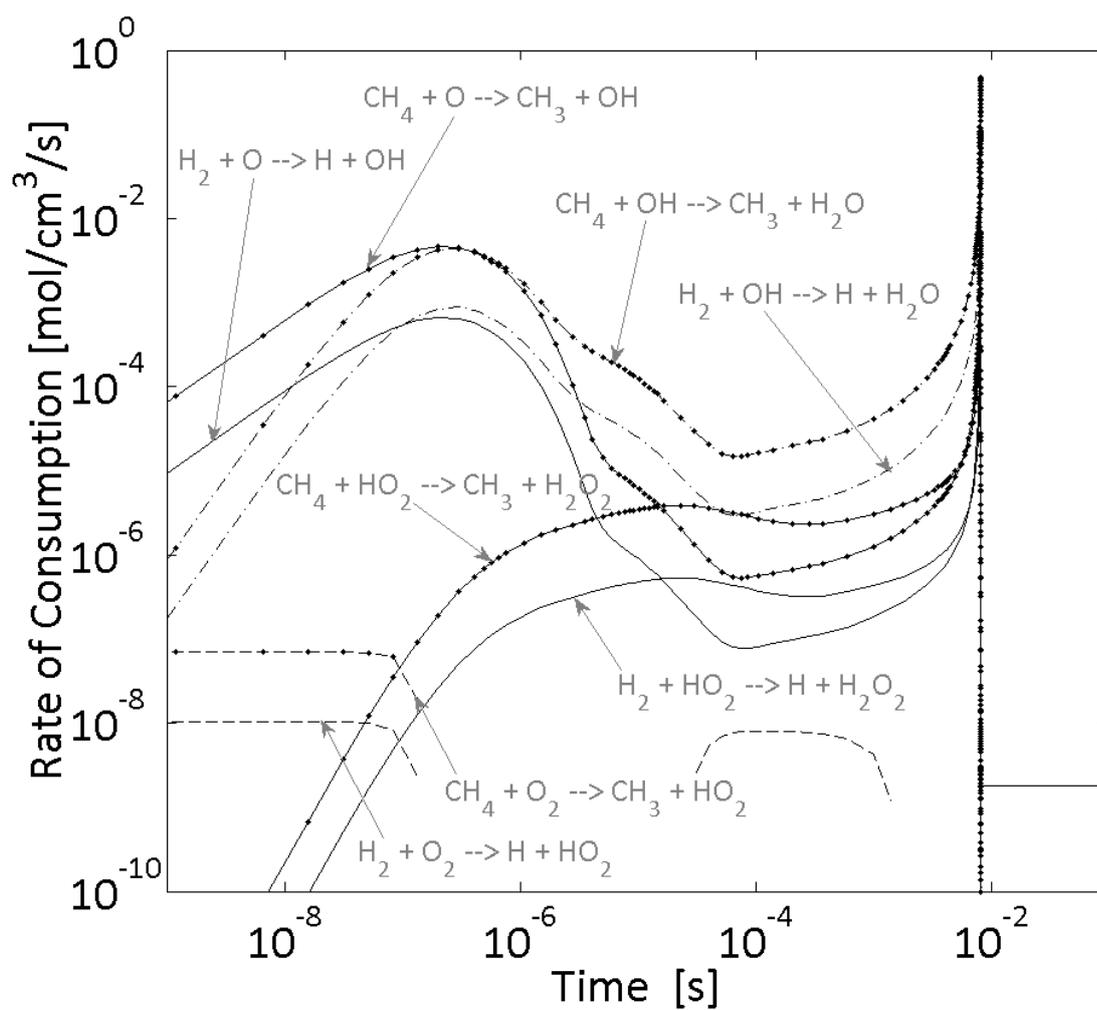
**Figure 108. D.** Rate of consumption for a mixture of methane and hydrogen (80/20) with 10 ppm of ozone.
