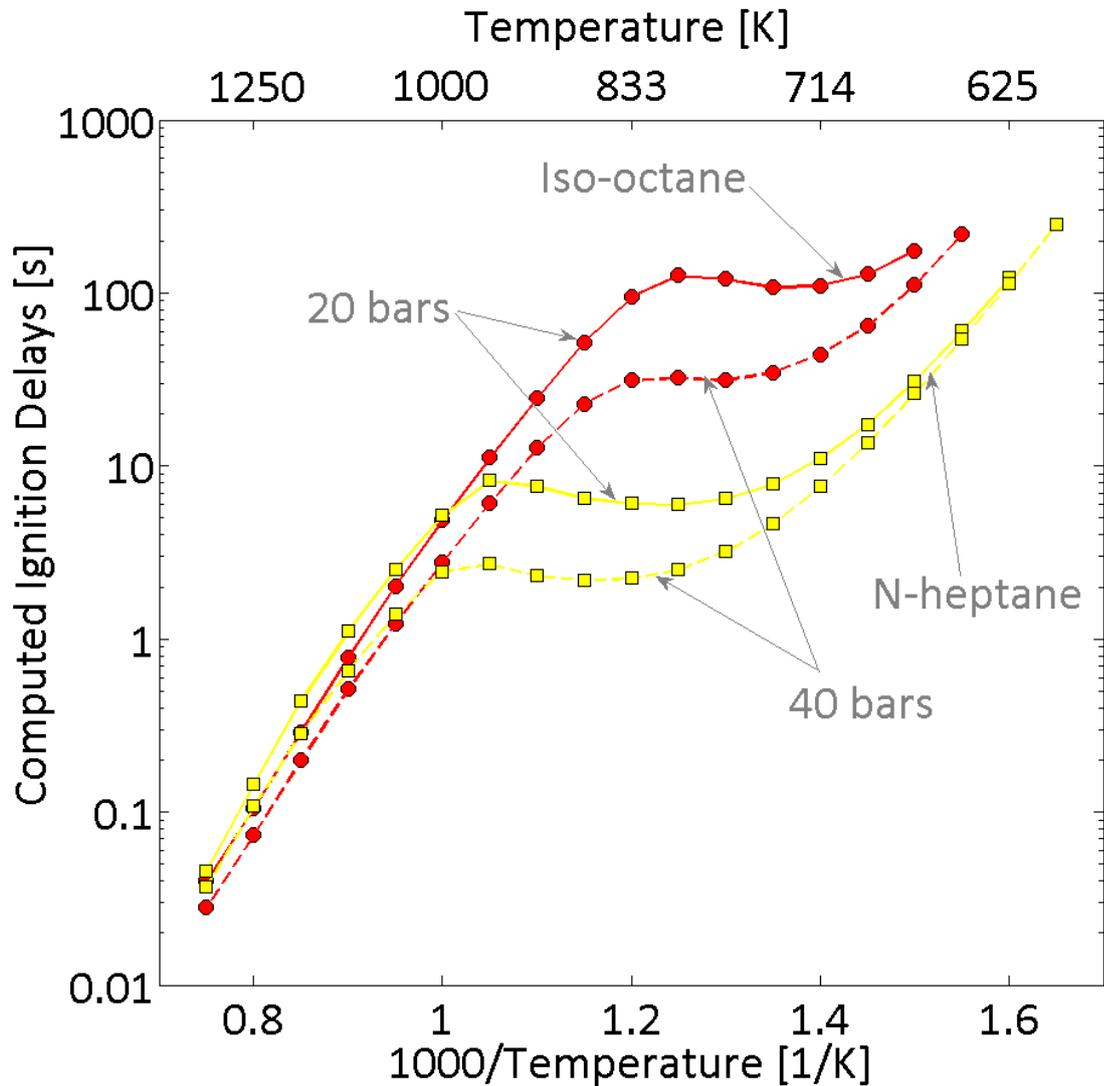
**Figure 55.** Computed ignition delays as a function of the inverse temperature for an equivalence ratio of 0.3, two initial pressure (20 bar in filled symbols and 40 bar in open symbols) and two fuels (squares for n-heptane and circles for isooctane). Symbols correspond to computed ignition delays results with the ozone submechanism and lines represent results without.
