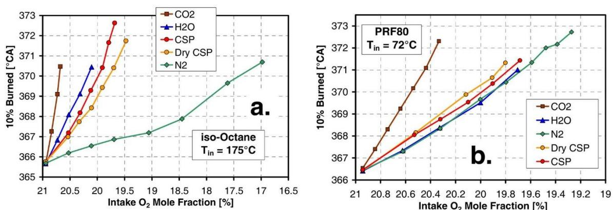
**Figure 30.** Effect of the main components of the EGR on CA10 for isooctane (on the left) and PRF80 (on the right) as fuel. CSP corresponds to the Complete Stoichiometric Products and is therefore composed of CO<sub>2</sub>, H<sub>2</sub>O and N<sub>2</sub>. Dry CSP corresponds to CSP without H<sub>2</sub>O [104].
