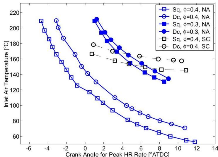
**Figure 27.** Intake air temperature versus combustion timing for two different piston geometries (Square: Sq and Disc: Dc). NA corresponds to Naturally Aspirated and SC to Supercharged [80].
