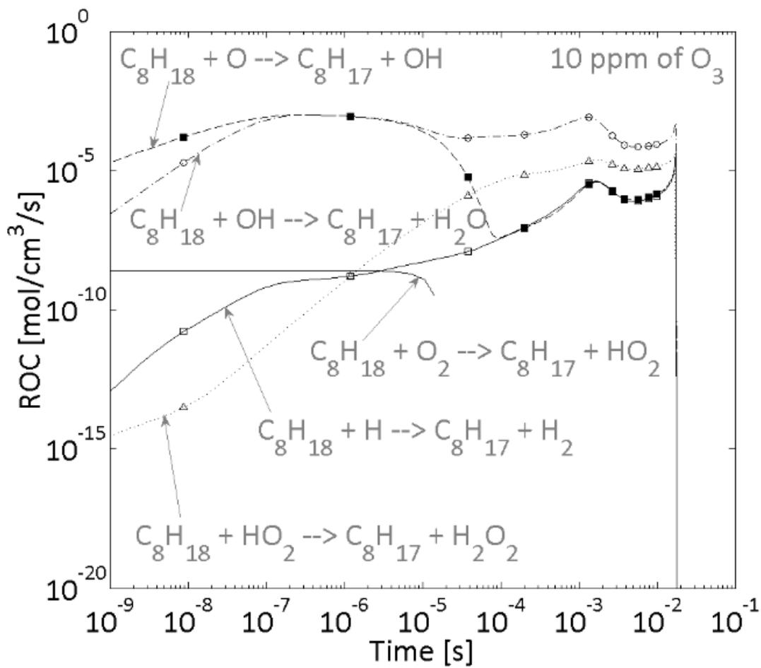
**Figure 58. D.** Reaction pathway analysis from rates of consumption for isooctane (PRF100) at an initial temperature of 800 K, initial pressure of 50 bar, an equivalence ratio of 0.3 and with 10 ppm of ozone.
