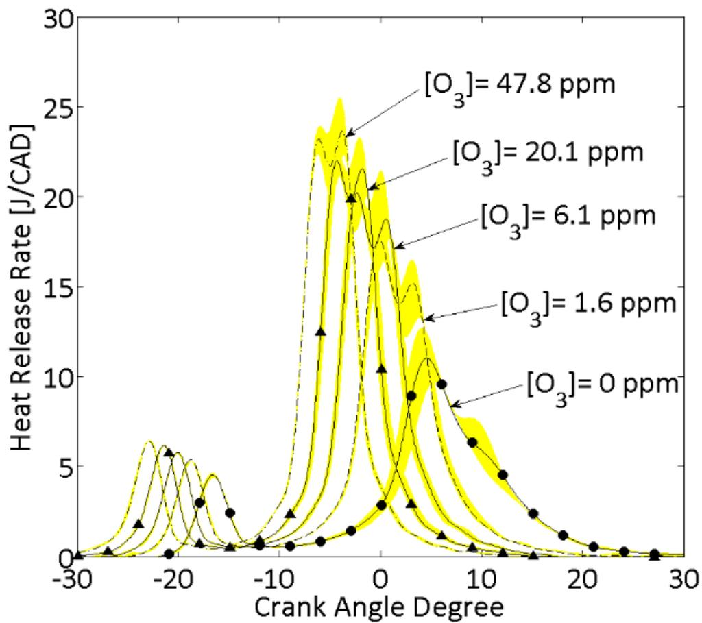
**Figure 51. B.** Heat release rate evolutions as a function of the ozone concentration injected in the intake of the engine for *n*-heptane/PRFO as fuel.
