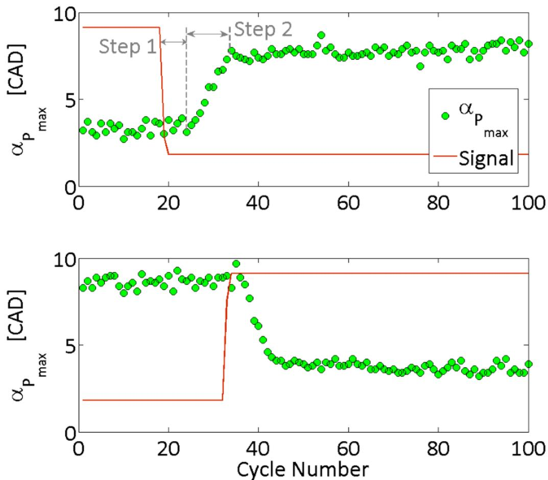
**Figure 86.** Cycle-to-cycle variations for an increase and a decrease of the combustion phasing. Dots correspond to the maximum pressure phasing at each cycle and lines correspond to the signal on the ozone generator. Step 1 and step 2 correspond to the transitional time.
