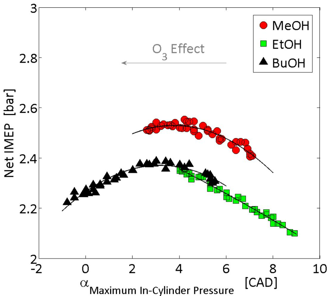
**Figure 114.** Net indicated mean effective pressure as a function of the maximum in-cylinder pressure and the ozone seeded for the three alcohol fuels selected. Symbols represent experiments and dashed lines the evolutions.
