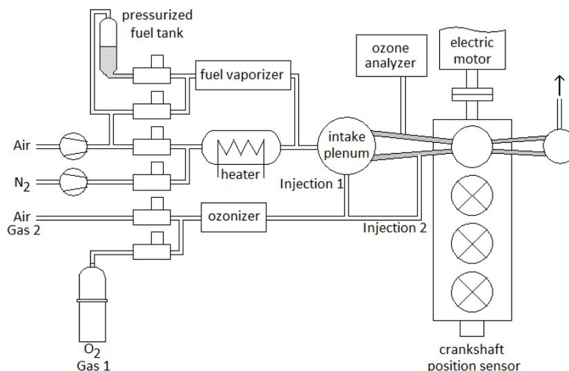
**Figure 75.** Scheme of the experimental setup for the application case. The ozone generator may be supplied either by pure oxygen or air and the ozone produced can be injected either inside the plenum or into one of the intake pipes.
