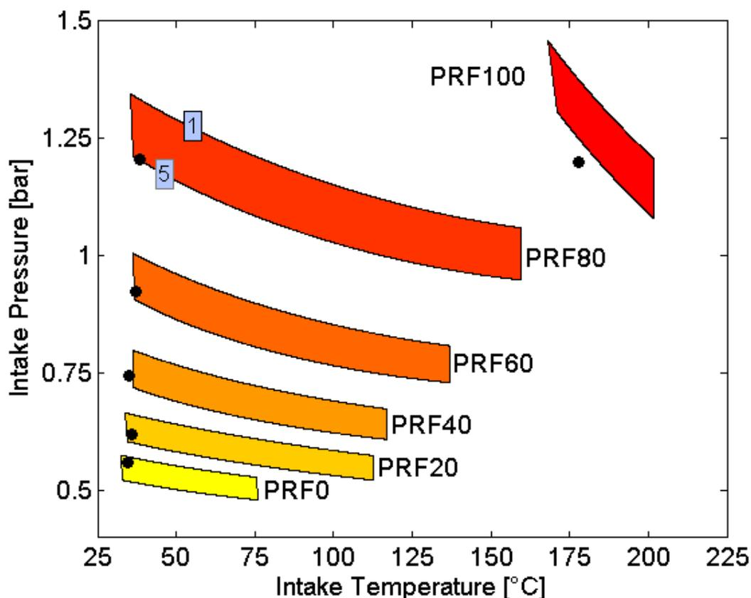
**Figure 50.** Optimal combustion areas for each PRFs selected as a function of the intake pressure and the intake temperature of the engine for an equivalence ratio of 0.3 and a rotation speed of 1500 rpm. 1 and 5 correspond to the iso-CA50 limits. Black points correspond to the conditions selected to examine the effect of ozone.
