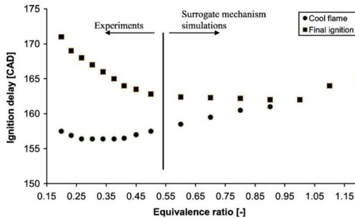
**Figure 22.** Ignition delays for *n*-heptane as fuel as a function of the equivalence ratio at a compression ratio of 10 and an intake temperature of 70 °C. Results for equivalence ratios up to 0.55 correspond to experimental results and upper than 0.55 come from computations [35].
