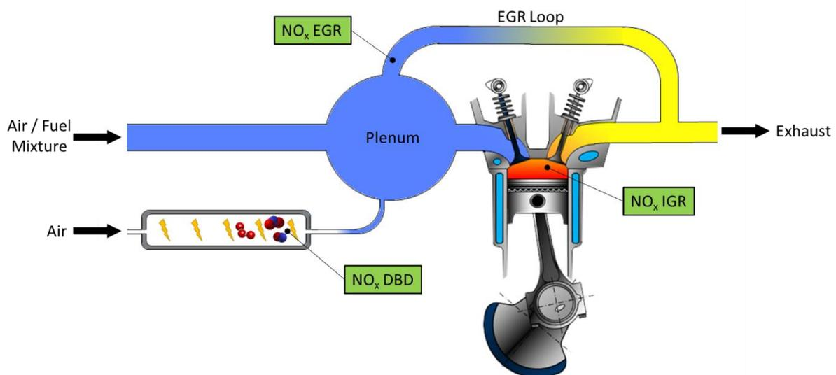
**Figure 63.** Scheme of the different sources of NO<sub>x</sub> into an engine using an ozone generator.
