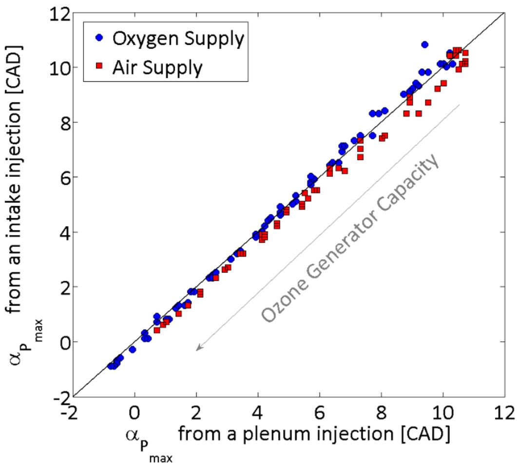
**Figure 78.** Effect of the ozone generator capacity on the maximum cylinder pressure for the two different injection positions, for the two different gases supplying the ozone generator (neat oxygen and dry air) and for the three intake temperatures selected (100 °C, 150 °C and 200 °C).
