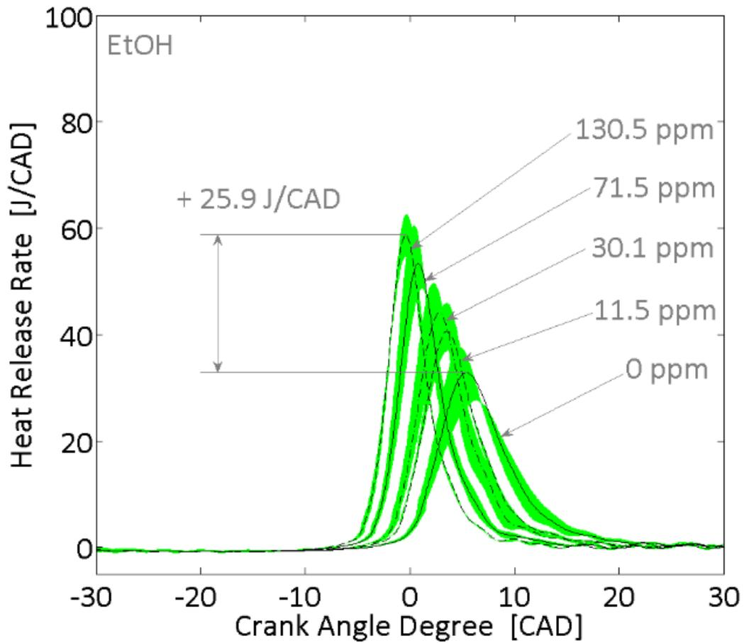
**Figure 110. D.** Heat release rate traces as a function of the ozone seeded for EtOH as fuel. Black curves correspond to the average of 100 cycles recorded and gray areas represent the variation of the same 100 cycles (the upper and the lower limits obtained).
