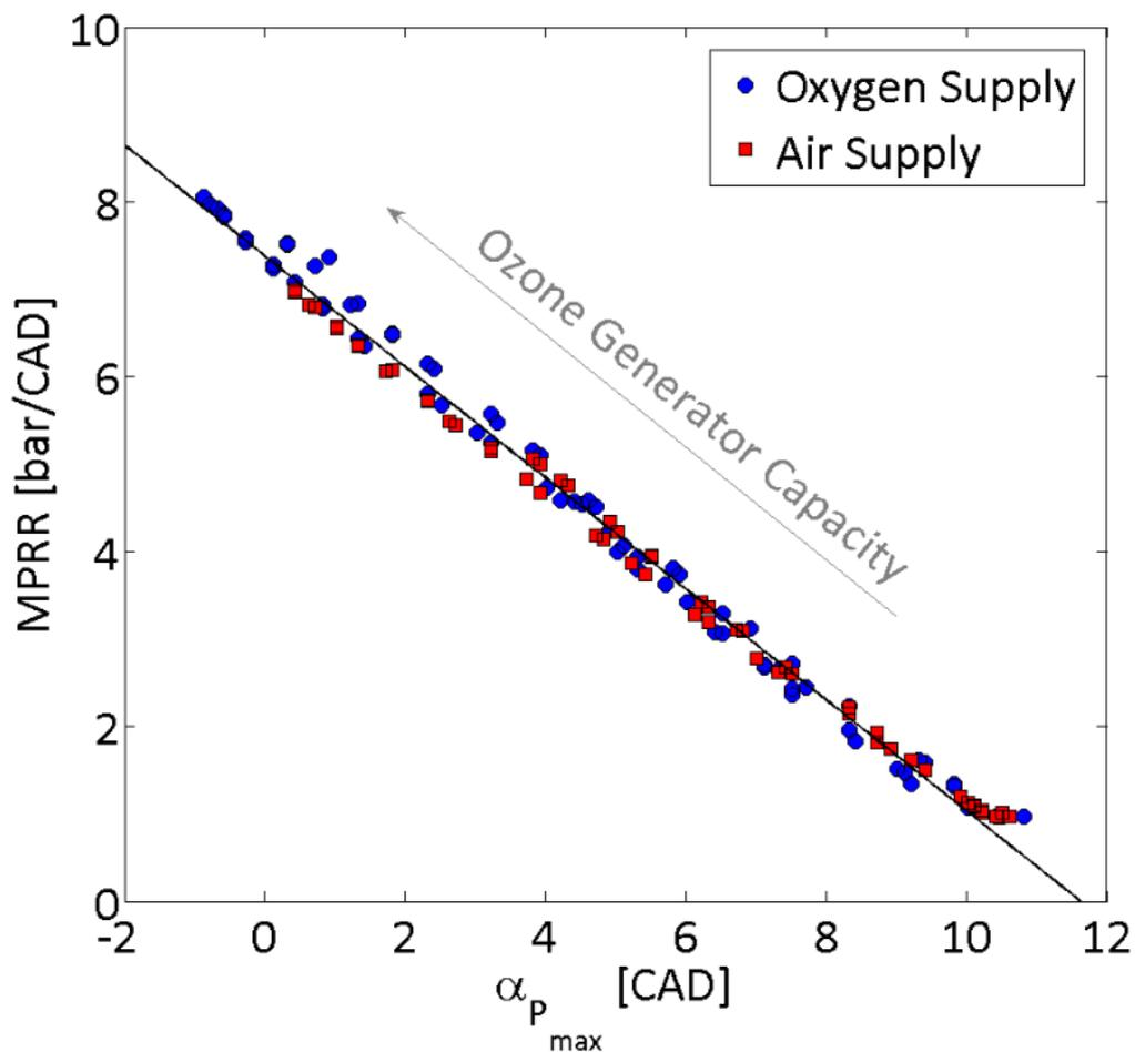
**Figure 81.** Maximum pressure rise rate as a function of the maximum pressure phasing for both types of gas supply, an injection inside the intake of the engine and the three intake temperatures selected.
