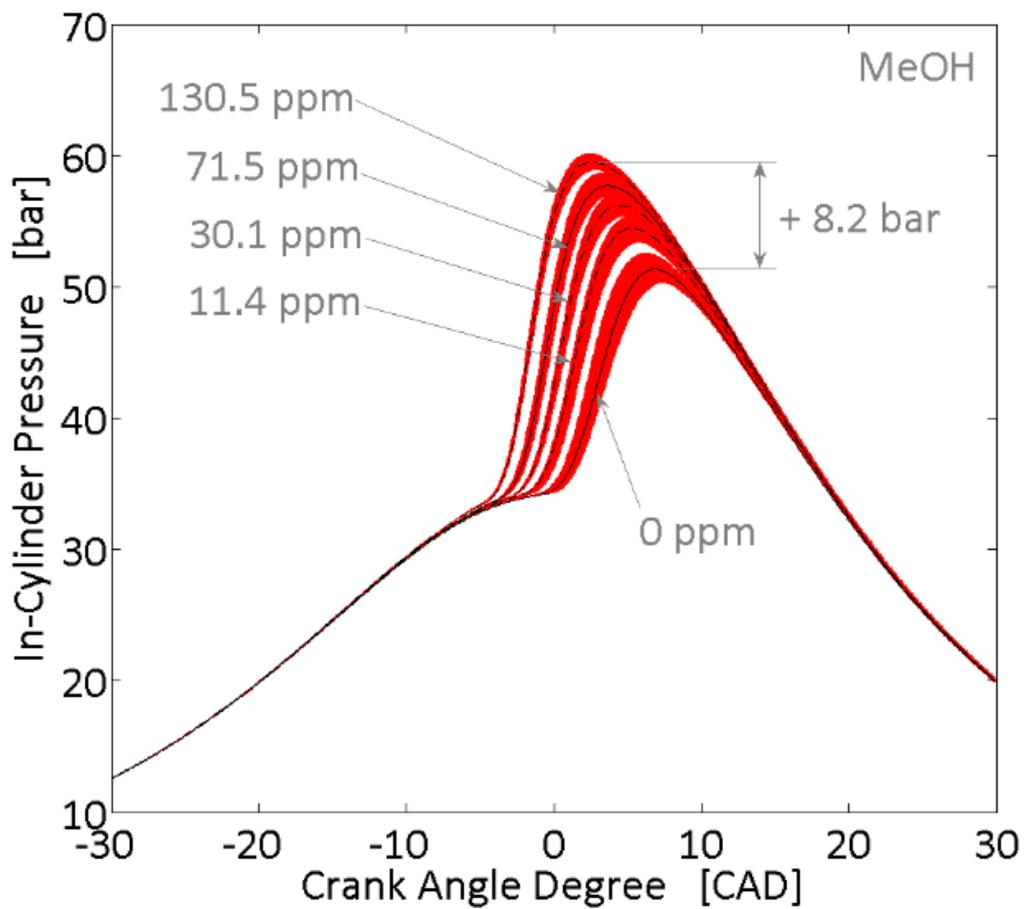
**Figure 110. A.** In-cylinder pressure traces as a function of the ozone seeded for MeOH as fuel. Black curves correspond to the average of 100 cycles recorded and gray areas represent the variation of the same 100 cycles (the upper and the lower limits obtained).
