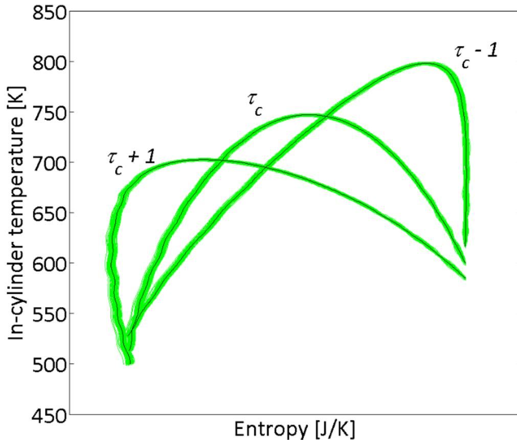
**Figure 41.** Temperature-Entropy diagram under various compression ratios. A wrong compression ratio shifts the shape of the diagram either towards the left or towards the right. This results in no thermodynamic senses while a good compression ratio allows obtaining the symmetry desired.
