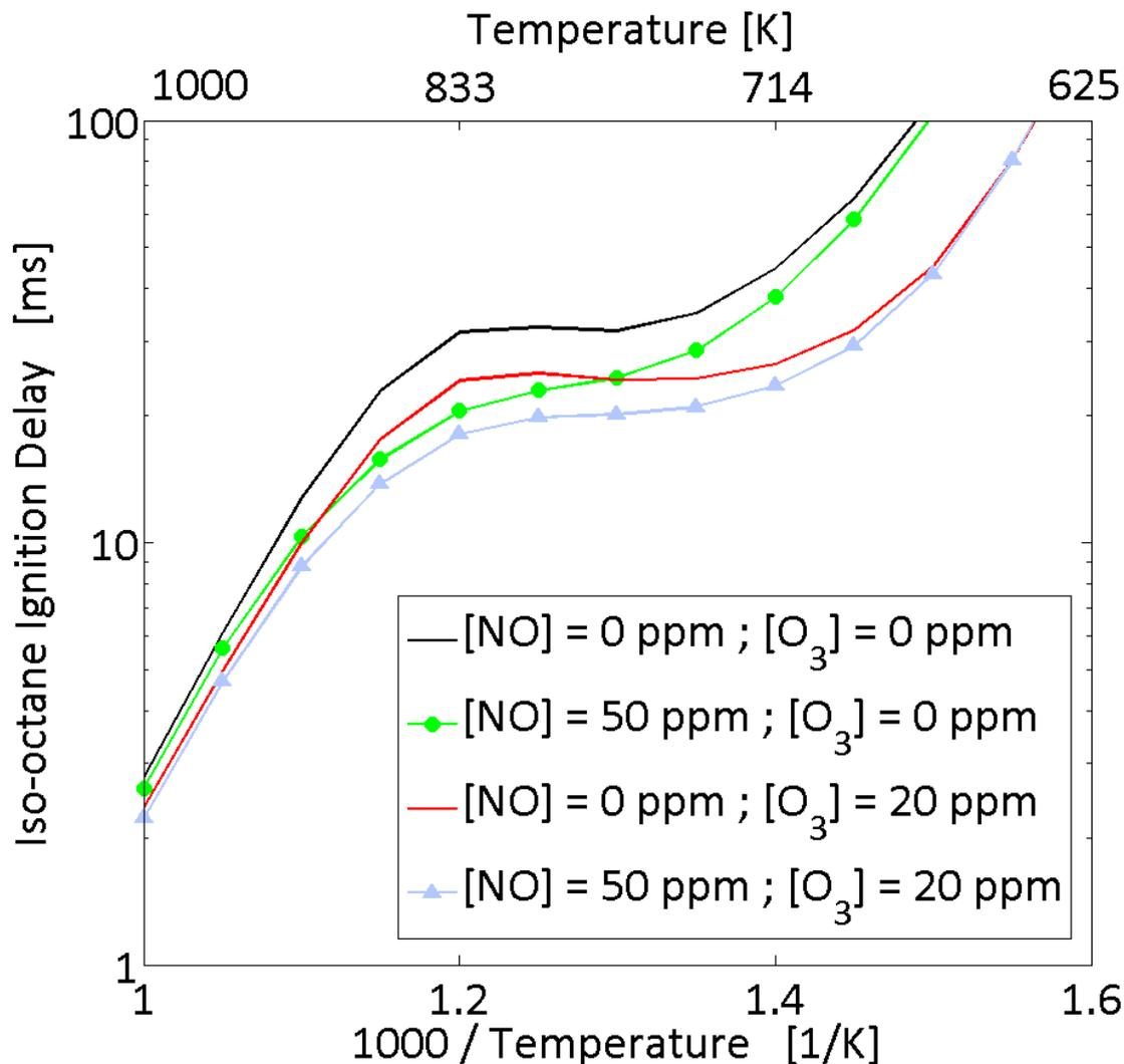
**Figure 70.** Ignition delays computed over a large temperature range in the case without any seeding, when nitric oxide is seeded alone, when ozone is seeded alone and when both oxidizing chemical species are together present.
