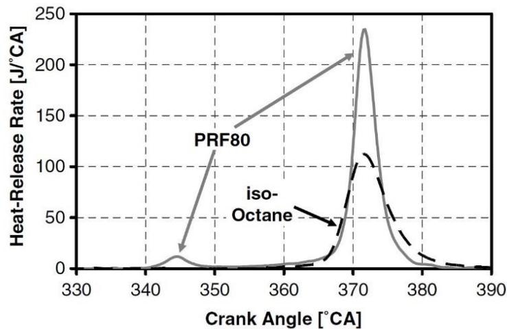
**Figure 18.** Heat release rate traces for iso-octane and PRF80 (80% iso-octane and 20% n-heptane) [27]. Iso-octane combustion is in single stage while PRF80 is in two stages. The first stage between 340 and 350 °CA corresponds to the low temperature regime or cool flame. The area from 350 to 360 °CA is related to the negative temperature coefficient (NTC) regime and after 360, the peaks corresponds to the main combustion.
