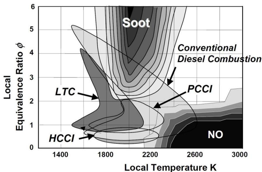
**Figure 16.** Equivalence ratio - Local temperature diagram from Kitamura et al. [18] and the location of Conventional Diesel Combustion and some of the most advanced combustion modes encountered into the literature [19].
