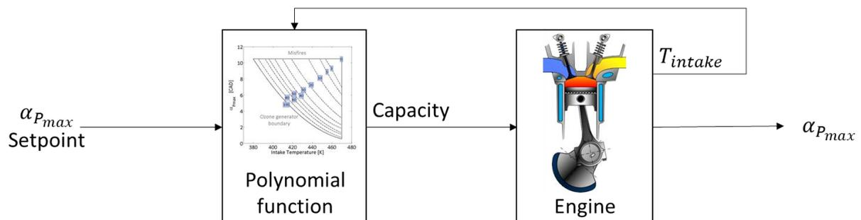
**Figure 87.** Scheme of the open-loop control.
