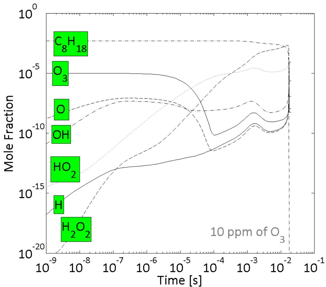
**Figure 58. C.** Mole fractions of the main radicals and the fuel for isooctane (PRF100) at an initial temperature of 800 K, initial pressure of 50 bar, an equivalence ratio of 0.3 and with 10 ppm of ozone.
