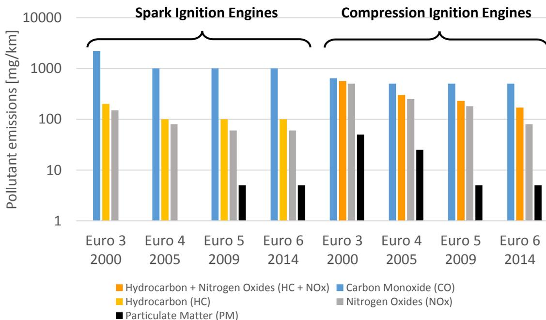
**Figure 14.** Evolutions of the pollutant requirements for light duty vehicles with Spark Ignition engines (on the left) and with Compression Ignition engines (on the right) [8]. Note: particles appear for Spark Ignition engines from the Euro 5 pollutant standard with the development of the stratified direct injection.
