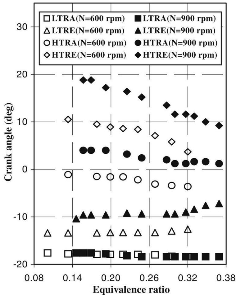
**Figure 26.** Effect of the engine speed and the equivalence ratio on the ignitions and the ends of both cool and main combustion stages for iso-butane as fuel [79]. LTRA corresponds to the Low Temperature Reaction Appearance, LTRE to the Low Temperature Reaction End, HTRA to the High Temperature Reaction Appearance and HTRE to the High Temperature Reaction End.
