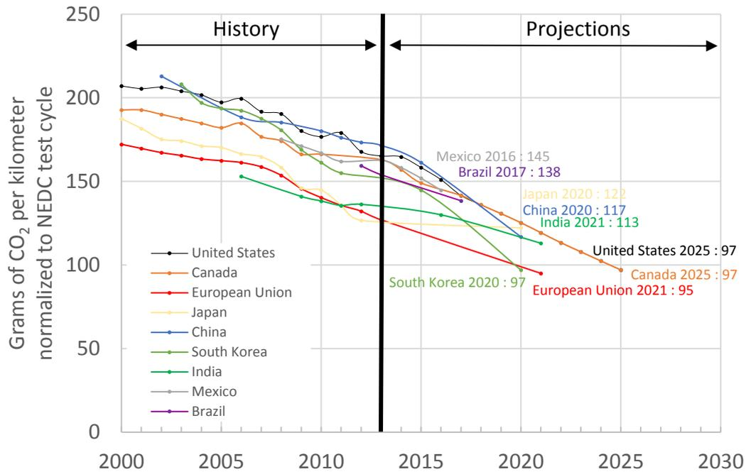
**Figure 13.** Forecasts of the CO<sub>2</sub> production per kilometer for light duty vehicles in reference to the NEDC cycle [7].
