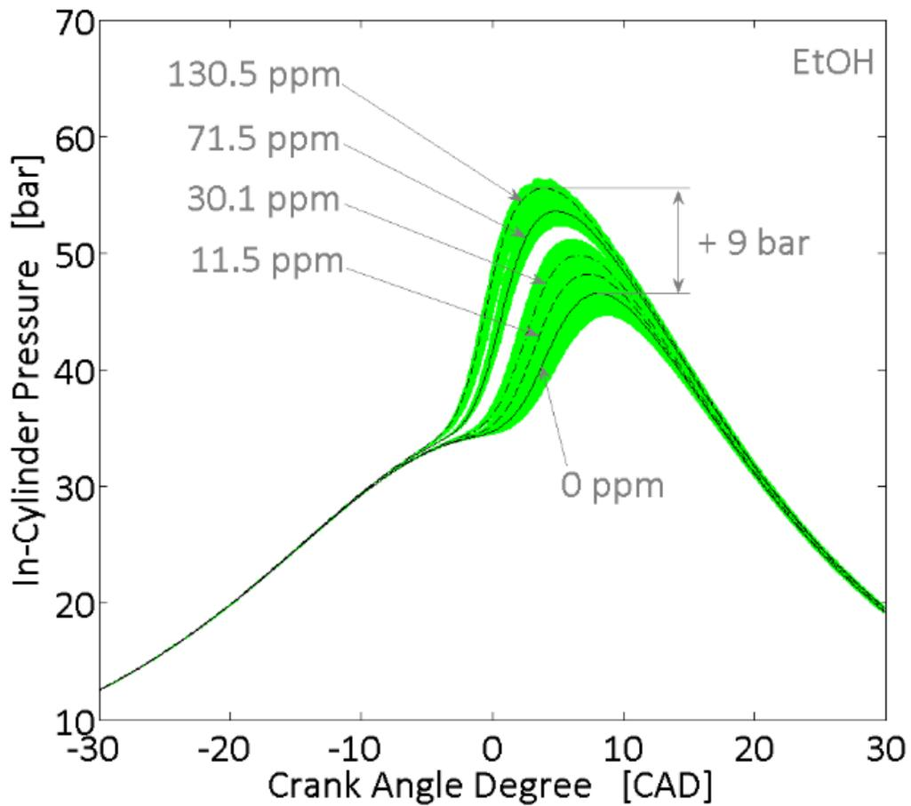
**Figure 110. C.** In-cylinder pressure traces as a function of the ozone seeded for EtOH as fuel. Black curves correspond to the average of 100 cycles recorded and gray areas represent the variation of the same 100 cycles (the upper and the lower limits obtained).
