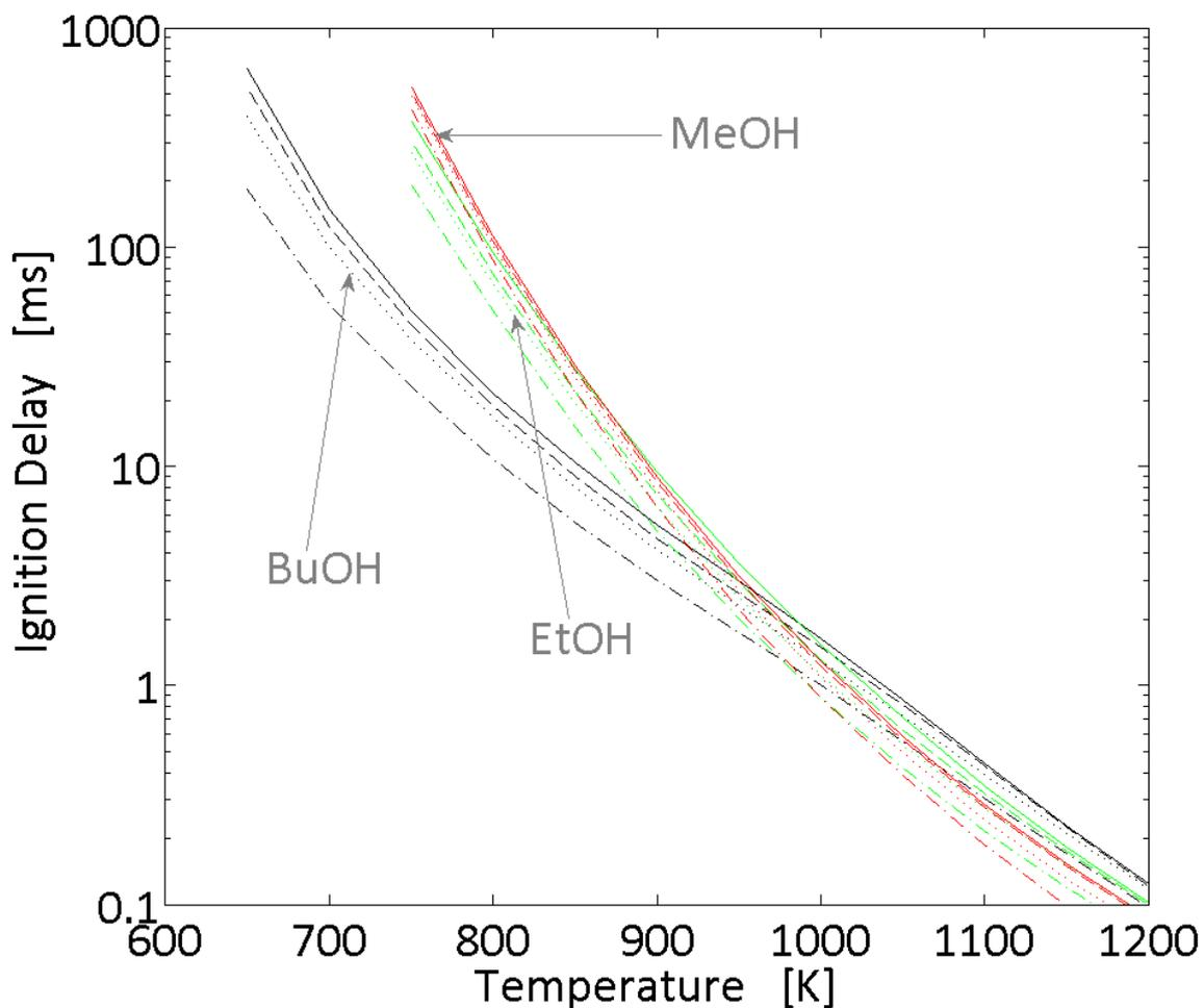
**Figure 117.** Ignition delays computed as a function of the temperature and the ozone concentration for the three alcohol fuels studied, for a pressure of 35 bar and an equivalence ratio of 0.3. Solid lines correspond to a concentration of 0 ppm, dashed lines to a concentration of 1 ppm, dotted lines to a concentration of 10 ppm and dash-dot lines to a concentration of 100 ppm.
