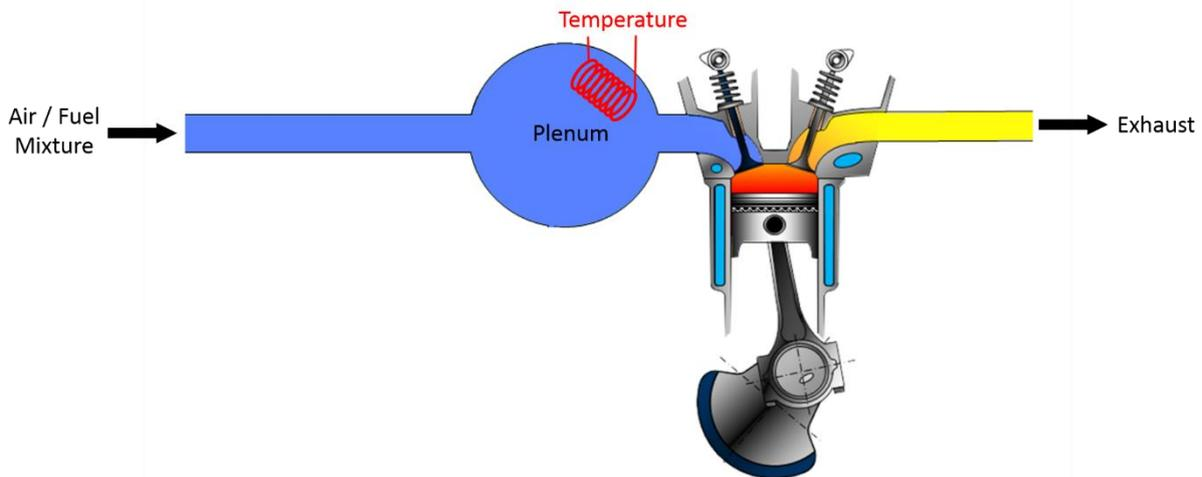
**Figure 36.** Scheme of the experimental setup in its normal configuration.
