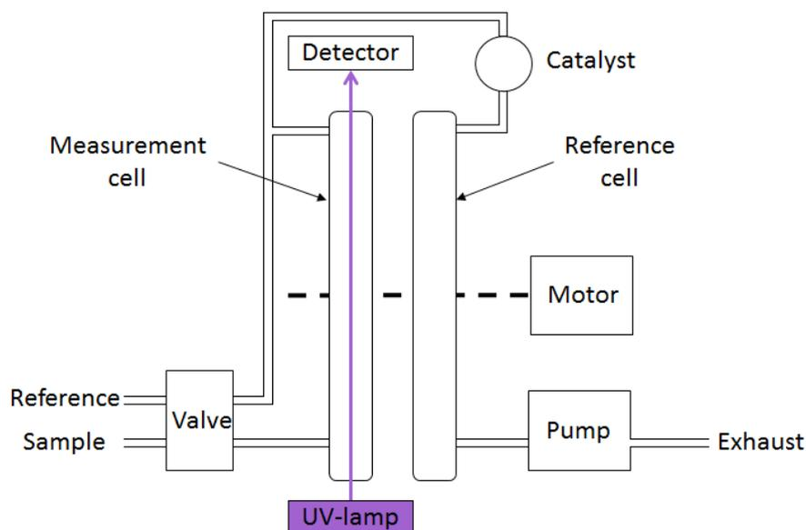
**Figure 38.** Scheme of the ozone analyzer used.
