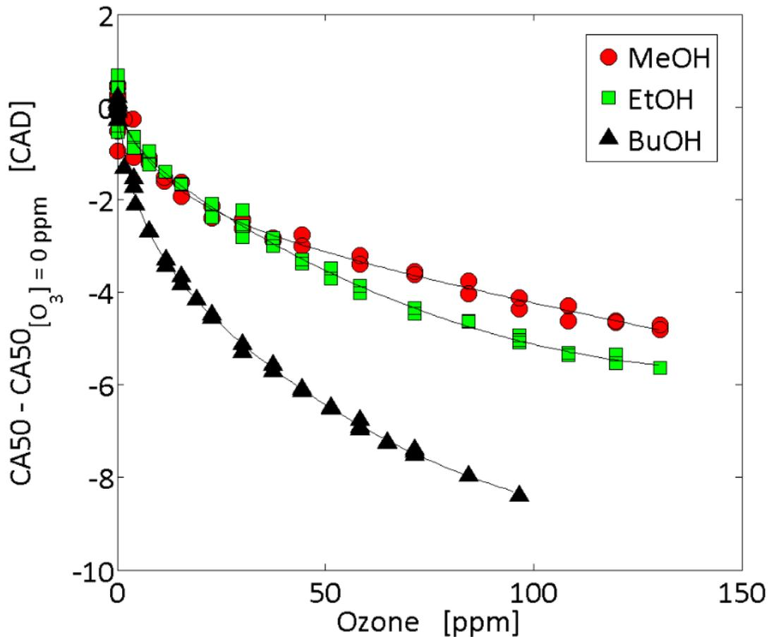
**Figure 112.** Effect of ozone on the shift of the CA50 with respect to the CA50 without ozone for the three alcohol fuels selected. Symbols correspond to the experiments and dashed lines to the trends.
