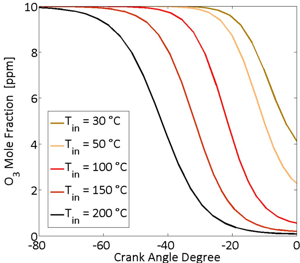
**Figure 56.** Computed ozone mole fraction during the compression stroke of an engine as a function of the crank angle degree under temperatures from 30 °C to 200 °C at a constant pressure of 1 bar.
