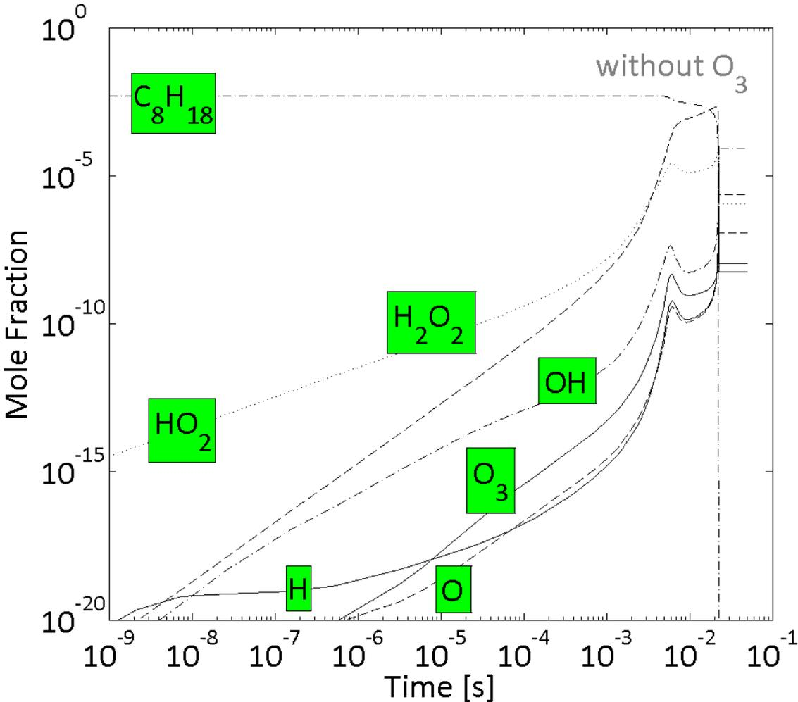
**Figure 58. A.** Mole fractions of the main radicals and the fuel for isooctane (PRF100) at an initial temperature of 800 K, initial pressure of 50 bar, an equivalence ratio of 0.3 and without ozone.
