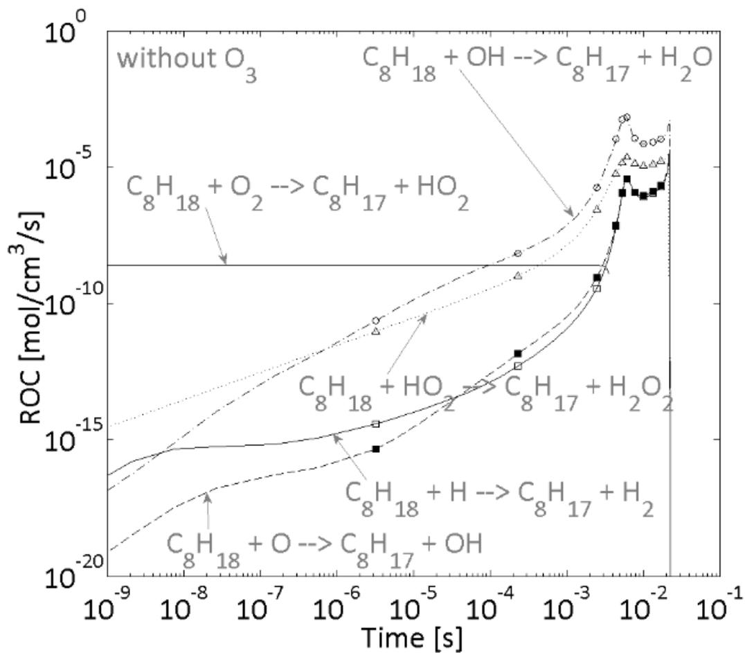
**Figure 58. B.** Reaction pathway analysis from rates of consumption for isooctane (PRF100) at an initial temperature of 800 K, initial pressure of 50 bar, an equivalence ratio of 0.3 and without ozone.
