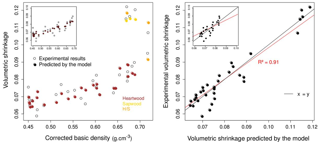
**Fig 6. Relationship between total volumetric shrinkage and corrected specific density in sapwood, heartwood and mixed samples.** Empty circles and full circles represent experimental results and predictions from the model m3 respectively. On the top-left corner is presented the heartwood-subsampling predictions using model m3\_h.
