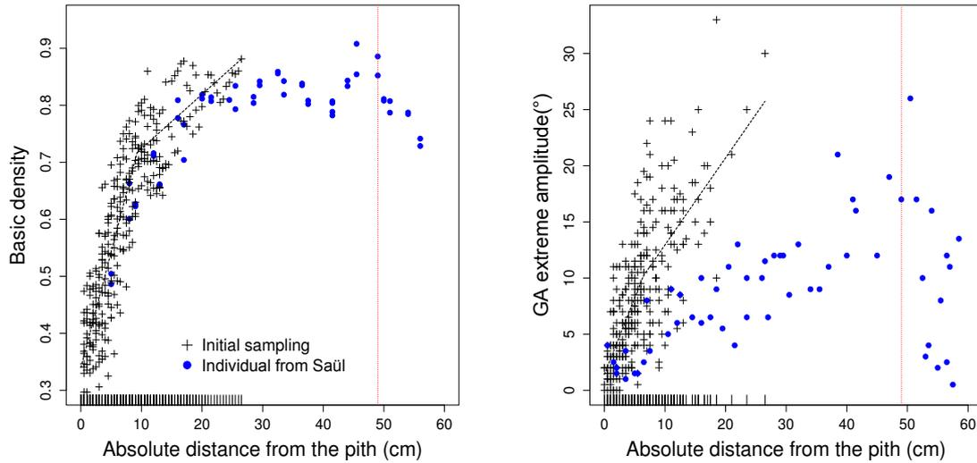
**Figure 7: Variation in IG extreme amplitude ( $^{\circ}$ ) and Wood Specific Gravity (BD) with absolute distance to the pith (cm). Black crosses correspond to the results from the original dataset and blue dots correspond to the measures obtained with the extra individual sampled in Saül.**
