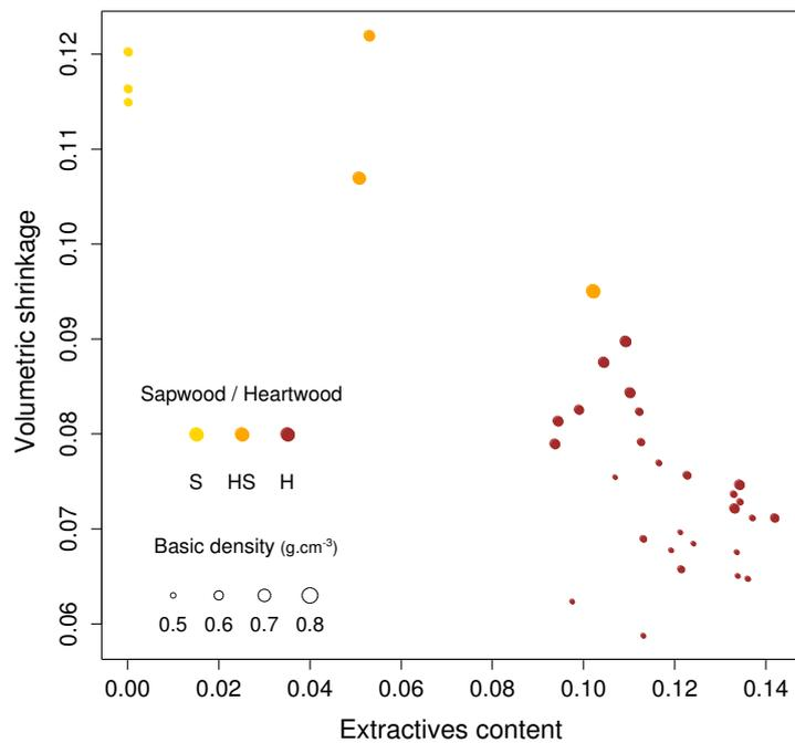
**Fig 4.** Effect of extractive content on the total volumetric shrinkage for one individual of *B. guianensis*. Basic density is represented by the thickness of the circles and colours correspond to different wood types.
