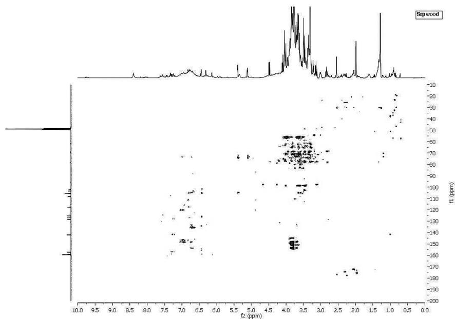
S5 Fig. HMBC NMR spectra of *B. guianensis* sapwood
