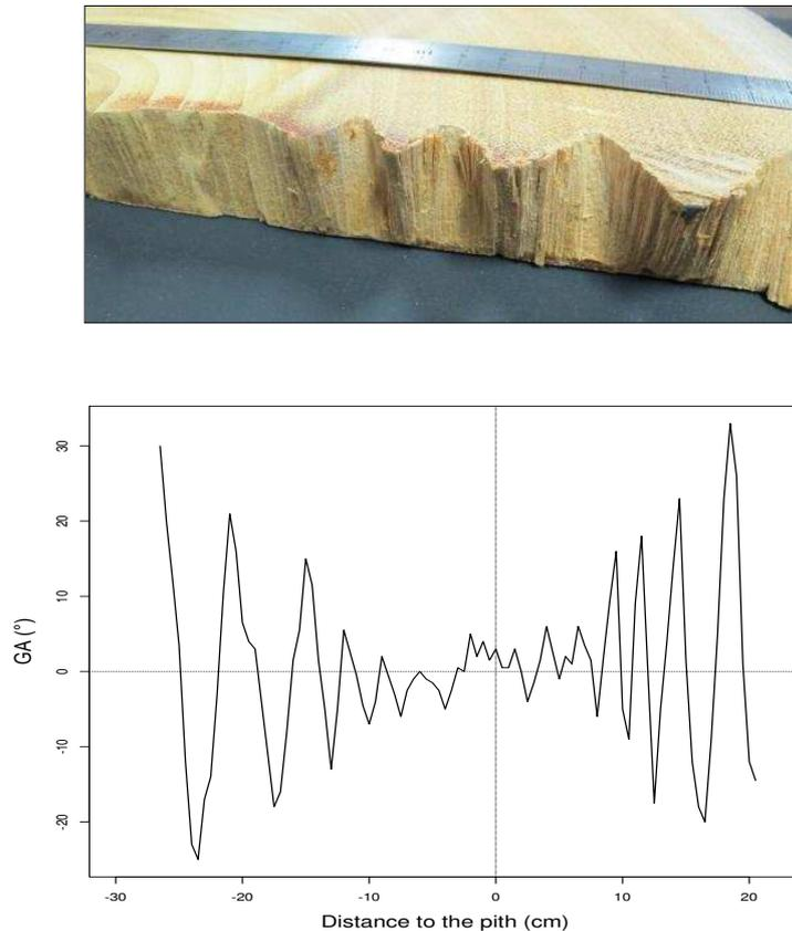
**Figure 5: Example of IG variations within a diametrical plank. Here are the results observed for the bigger tree of the sampling, the individual 9. The corresponding ring used for these measured is represented above the graph. IG amplitudes are increasing with distance from the pith and there are the same numbers of period in each side of the pith.**
