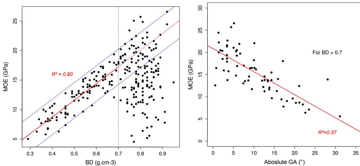
**Figure 8: Variations of Modulus of Elasticity (MOE) with Wood Specific Gravity (BD). The linear model applied on samples on which BD is under 0.7 is represented in red ( $R^2=0.80$ ). The continuity of this model for denser samples is represented with a red dotted line. Blue dotted lines represent the interval of prediction.**
