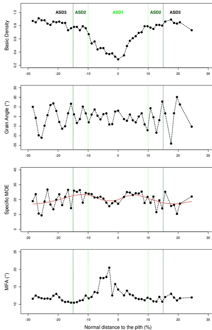
**Figure 10: Variations in BD, IG, MOE, Specific MOE and MFA with the absolute distance from the pith (%) for the individual 9 in *B. guianensis*. The two stages of development mentioned in the discussion are represented by the black dotted lines and correspond to a radial distance from the pith of 9.2 cm. The red line on specific MOE profile indicates the mobile average on four points.**
