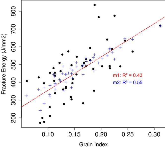
**Figure 9:** Variation of Rupture Energy from tenacity test on the Grain Index measured on split samples. The red dotted line represents the simple linear model (m1) and the blue crosses represent the predicted values given by the multi linear mode using Grain Index and MOE as parameters. R squared value are reported on the figure for each model (in red: m1; in blue: m2)
