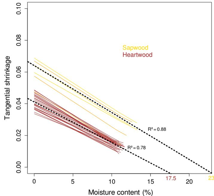
**Fig 2. Relationship between tangential shrinkage and moisture content (MC) for sapwood and heartwood subsampling of *B. guianensis* used for chemical extractions (N = 33).** Yellow and brown lines respectively correspond to sapwood and heartwood measures and black dashed lines indicate the mean values calculated for each subsampling.
