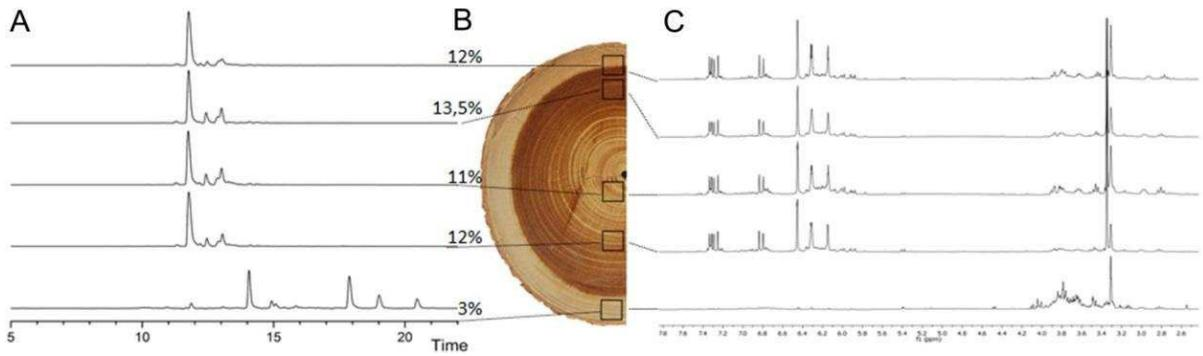
**Fig 3.** Stacked view of HPLC chromatograms (A), <sup>1</sup>H NMR spectra of heartwood and sapwood extractives (C) and corresponding extraction yield (B).
