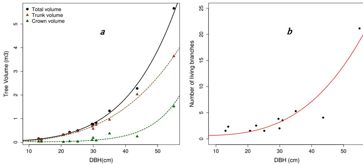
**Figure 3: a) Contribution of trunk (brown triangles) and crown (green triangles) volumes to the total volume (black circles) as a function of the Diameter at Breast Height (DBH). b) Increase of the number of living branches with DBH.**
