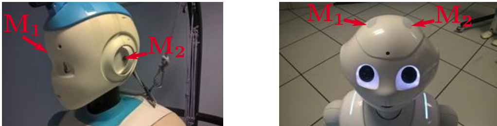
Figure 6.2: Auditory system of Romeo and Pepper
