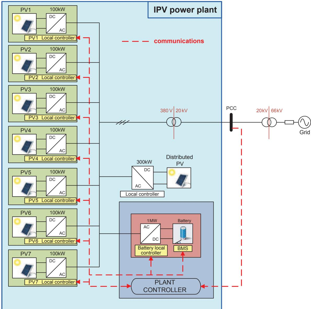
Figure 2.4: Configuration of the IPV power plant (in operation between 2012 and 2013).
