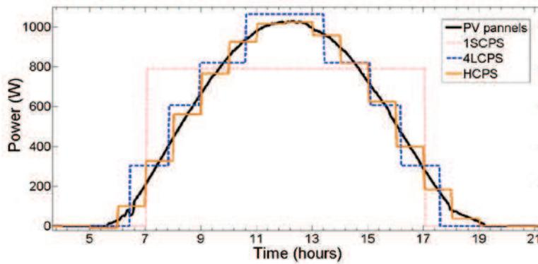
Figure 1.14: Real PV power production pattern and different power commitment according to different EMS configurations [23].
