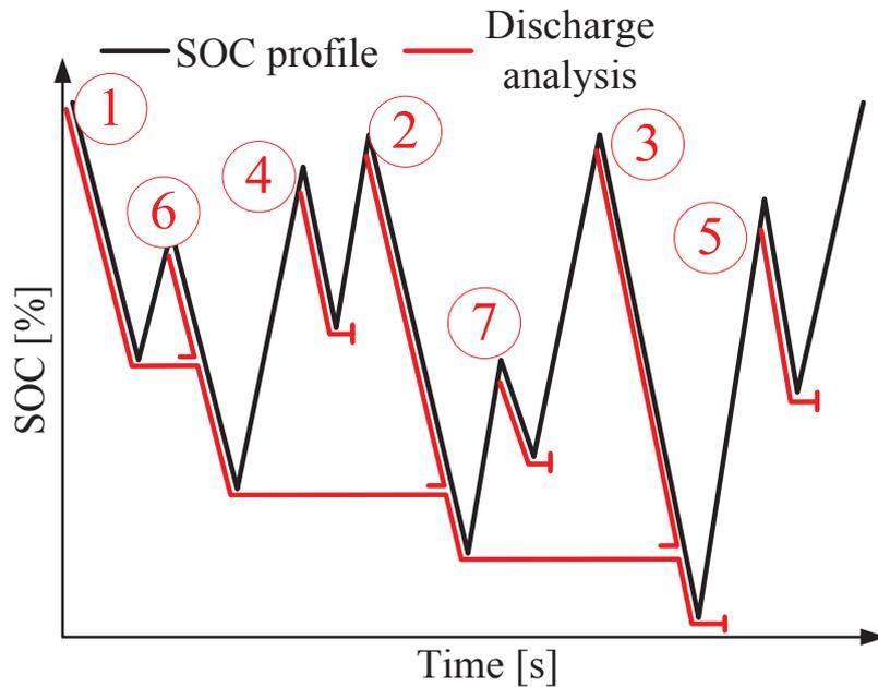
Figure 2.12: First step of *Rainflow* cycling counting algorithm (discharge analysis).
