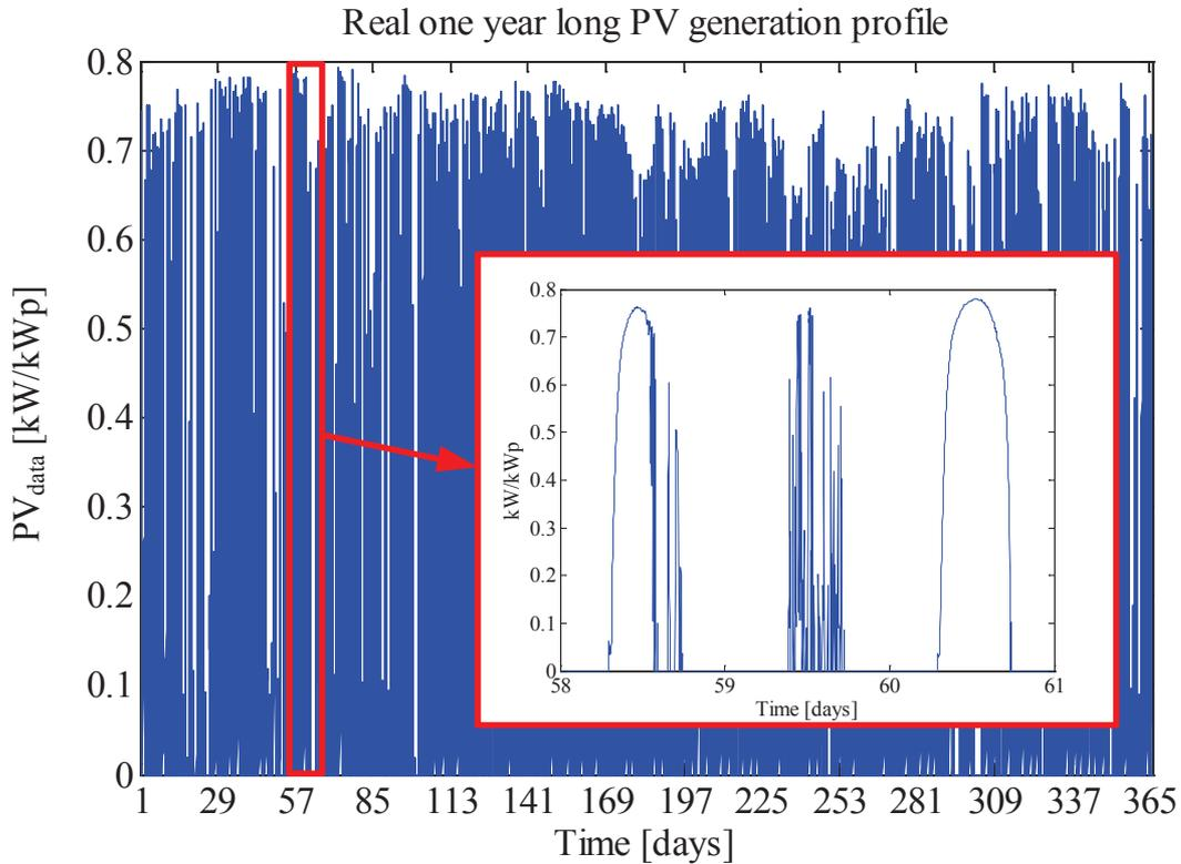
Figure 2.9: Real one year long PV generation profile with a three days detail [26].
