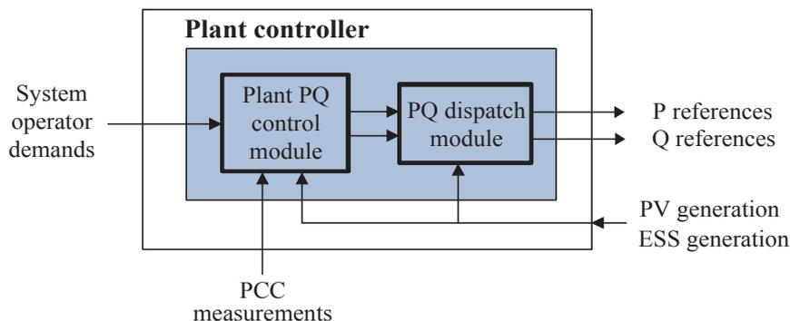
Figure 2.6: Internal control blocks of the plant controller [14].
