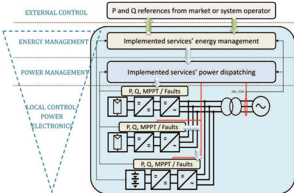
Figure 1.9: Representation of the hierarchical control structure on the IPV application.
