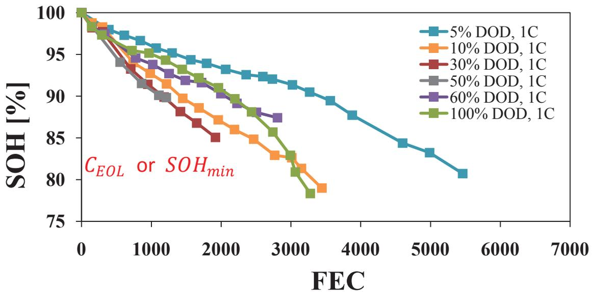
Figure 2.10: Example of cycling ageing for six different DOD [140].
