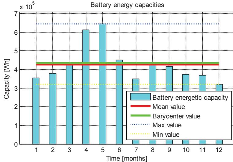
Figure 4.7: Design stage ESS sizing optimization results: battery energy capacity values.
