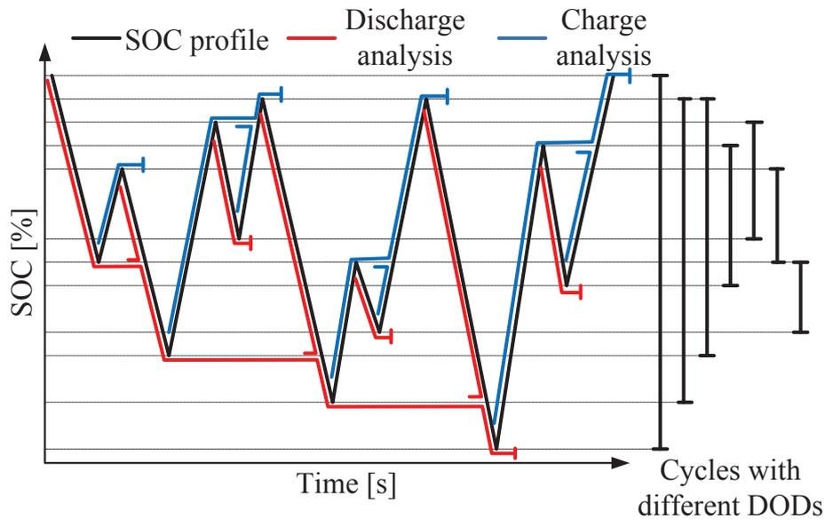
Figure 2.14: Third step of *Rainflow* cycling counting algorithm (matching process).
