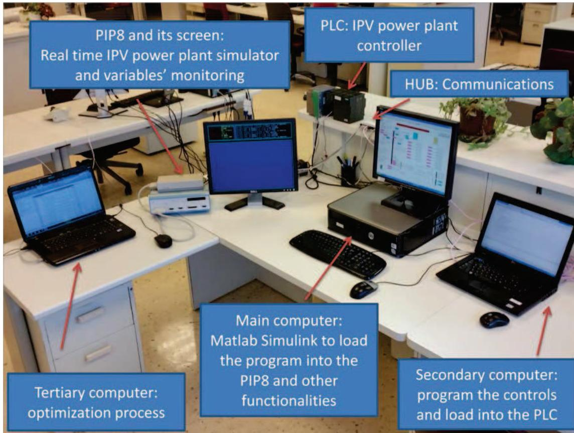
Figure 5.1: Real time validation platform picture.
