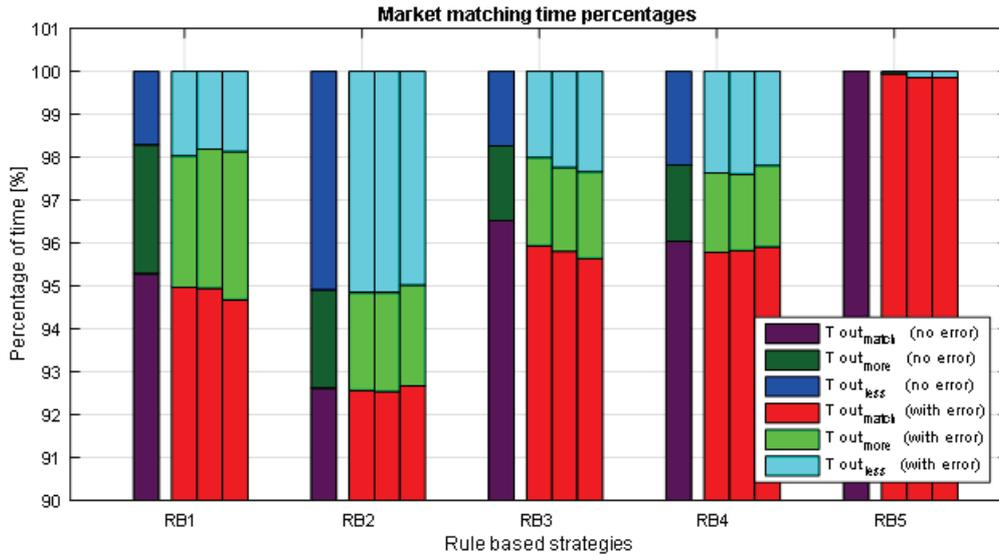
Figure 3.6: Results of market matching time percentages of the whole year simulation with (with error) and without prediction errors (no error).
