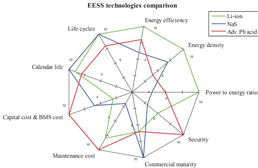
Figure 2.1: Spider chart of relevant BESS technologies comparison.
