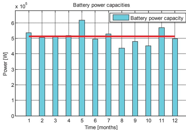
Figure 4.6: Design stage ESS sizing optimization results: battery power capacity values.
