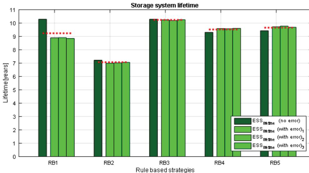
Figure 3.7: Results of storage system lifetime of the whole year simulation with (with error) and without prediction errors (no error).
