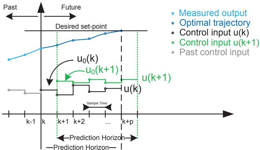
Figure 3.10: MPC operation summary diagram.
