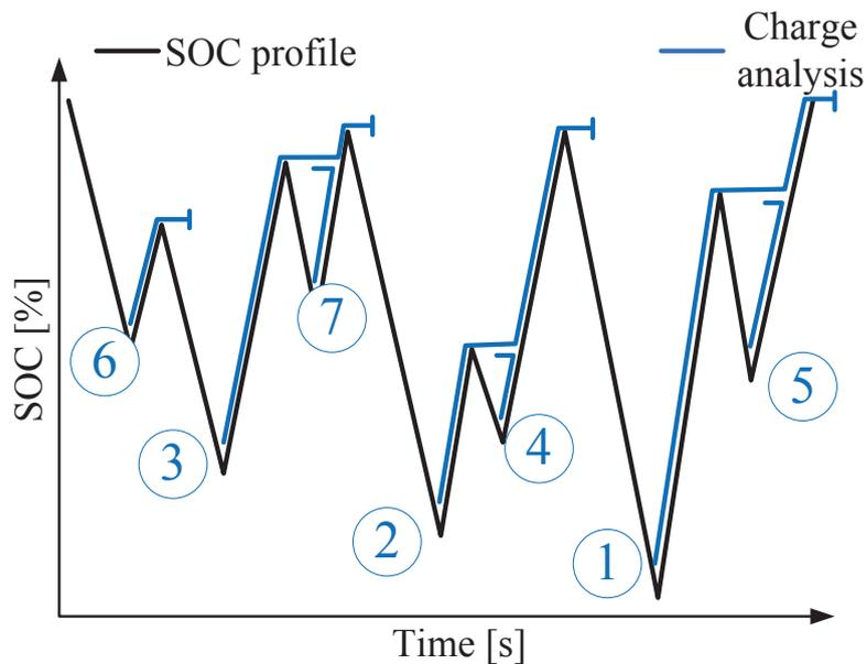
Figure 2.13: Second step of *Rainflow* cycling counting algorithm (charge analysis).
