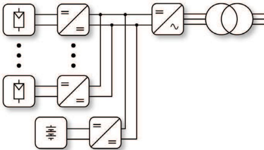
Figure 1.5: Power architecture of IPV power plant with the centralized storage connected in DC.
