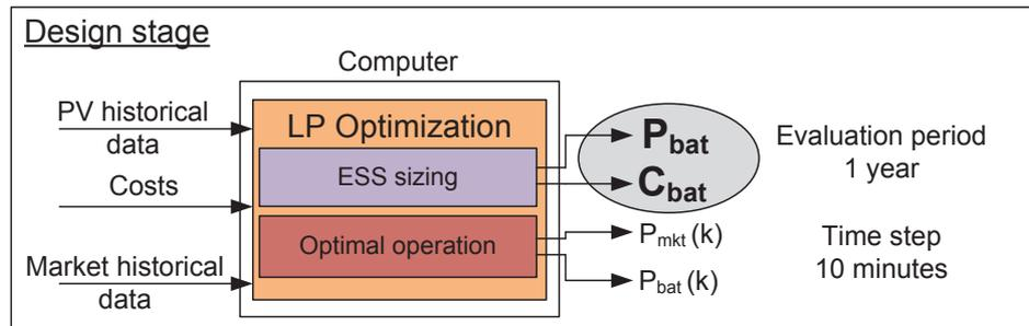
Figure 4.4: Design Stage of the process where the optimal sizing of the ESS is obtained.
