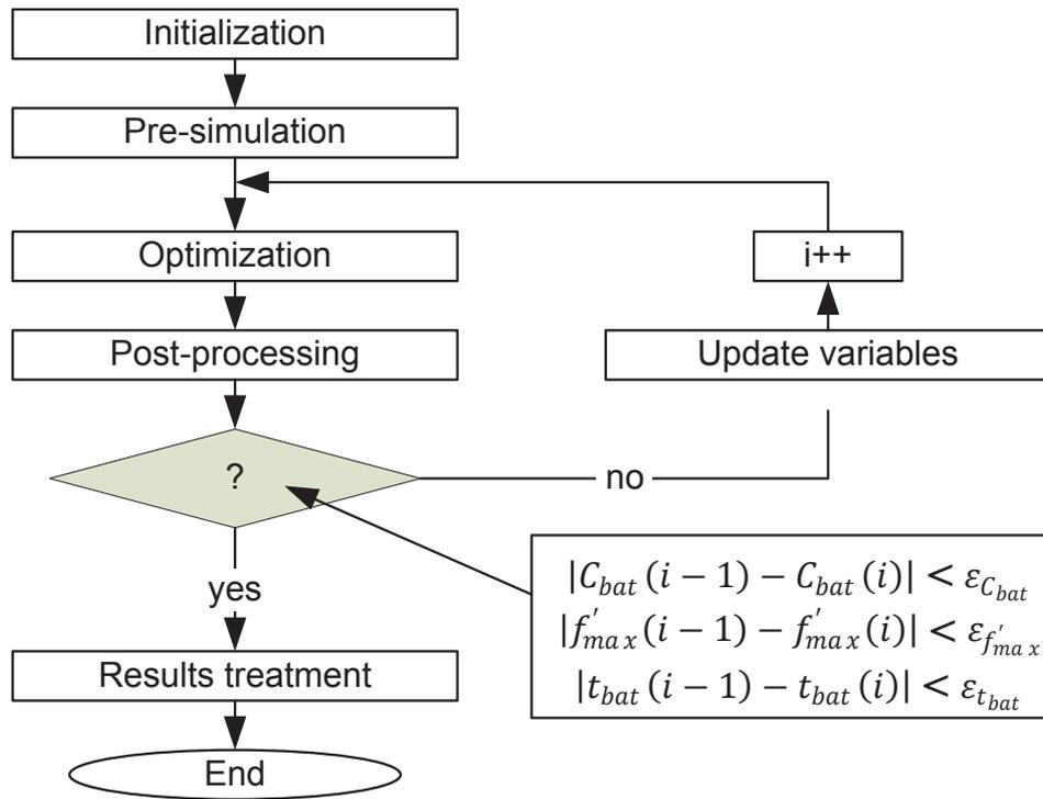
Figure 4.3: Complete simulation execution flowchart.
