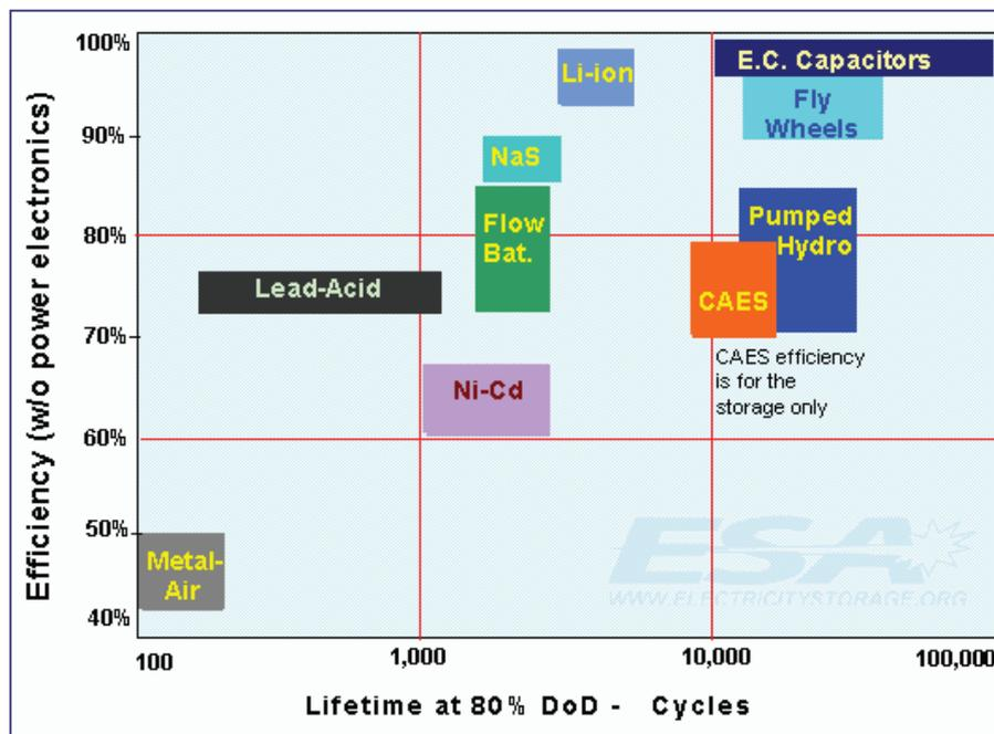
Figure 1.13: Energy storage technologies' efficiency versus their lifetime [60].
