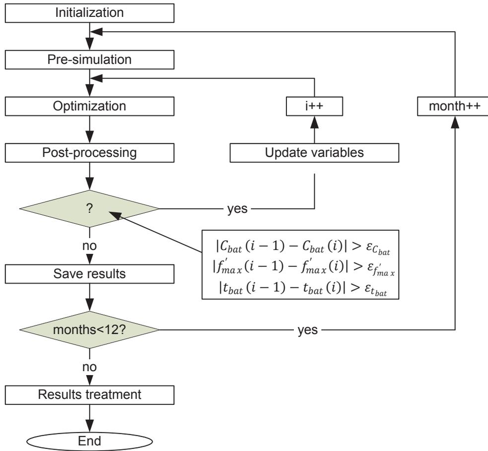
Figure 4.5: Design Stage of the process where the optimal sizing is determined.
