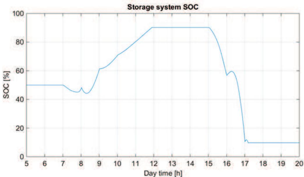
Figure 5.5: Storage system SOC variation corresponding to a sunny day operation based on RB control strategy.
