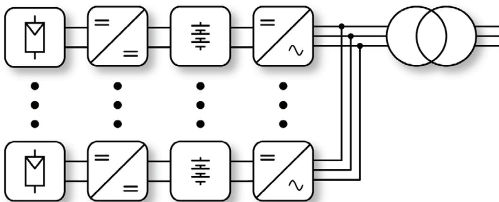
Figure 1.6: Power architecture of IPV power plant with distributed storage.
