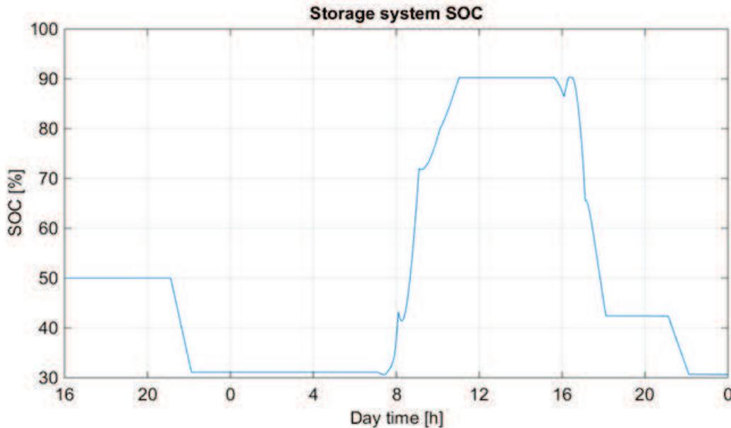
Figure 5.14: Storage system SOC variation corresponding to a sunny day operation based on the optimal control strategy.
