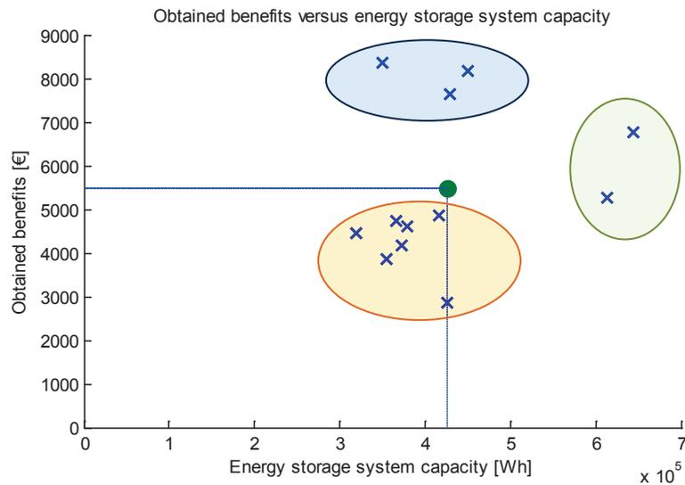
Figure 4.10: Design stage ESS sizing optimization results: obtained benefits versus capacity values.
