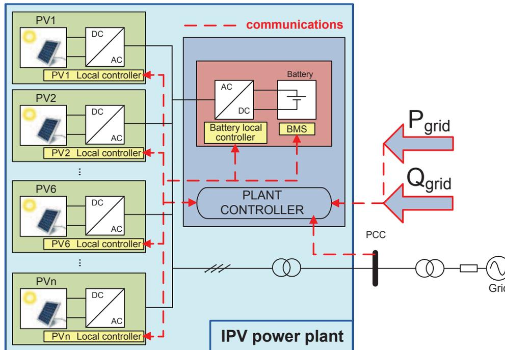
Figure 1.7: IPV power plant overview with the controllers and their communications.
