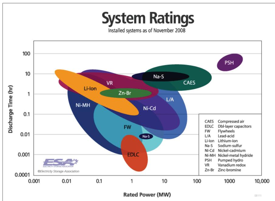
Figure 1.12: Energy storage technologies discharge time versus their rated power [60].
