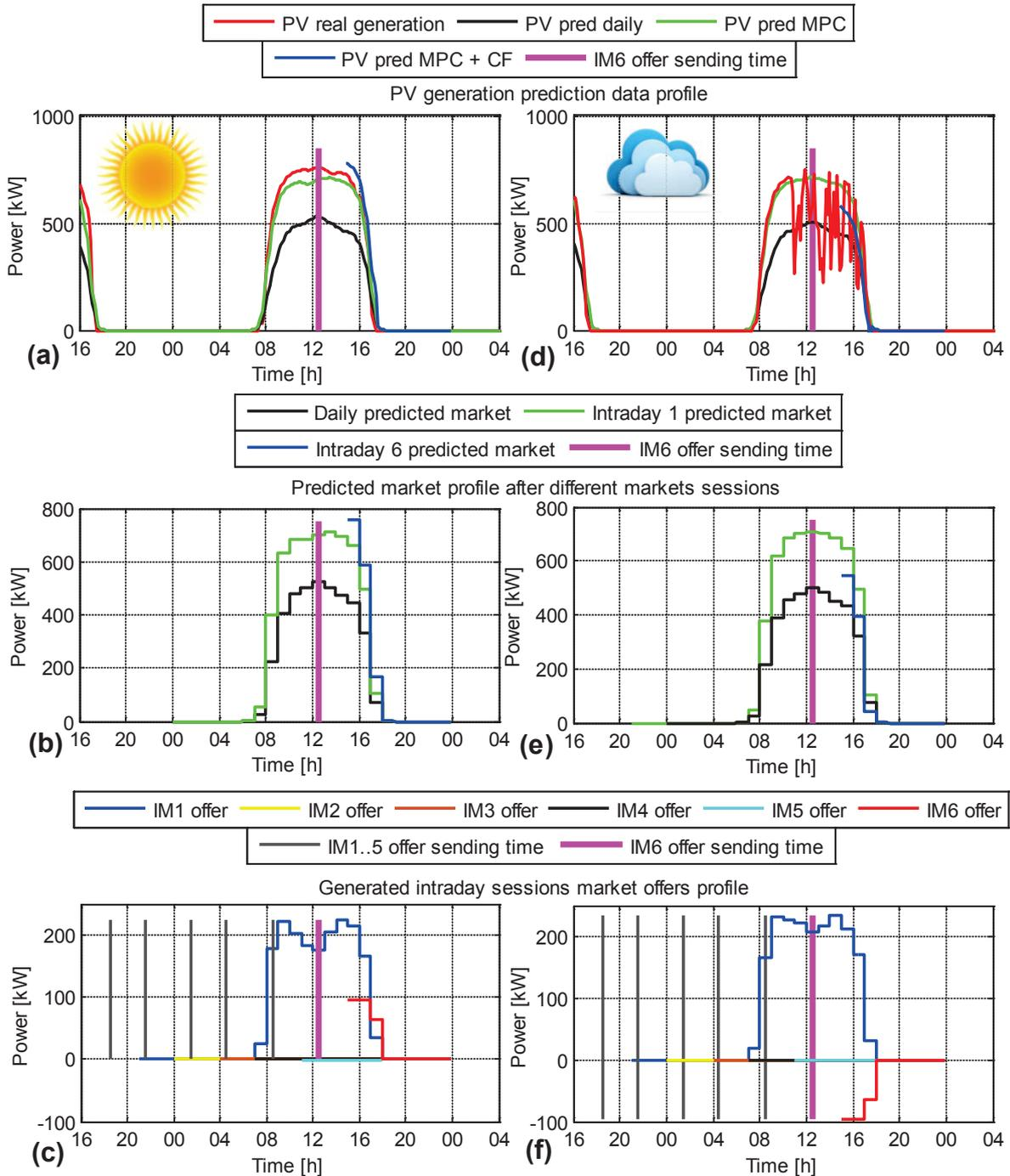
Figure 3.12: Online operation results for a sunny day (a, b and c) and for a cloudy day (d, e and f). a and d: PV generation predictions and real generation; b and e: predicted market profiles; c and f: intraday offers calculated by the MPC.
