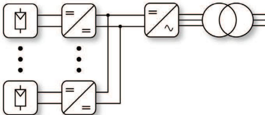
Figure 1.2: PV power plant with the modules connected in DC [32].
