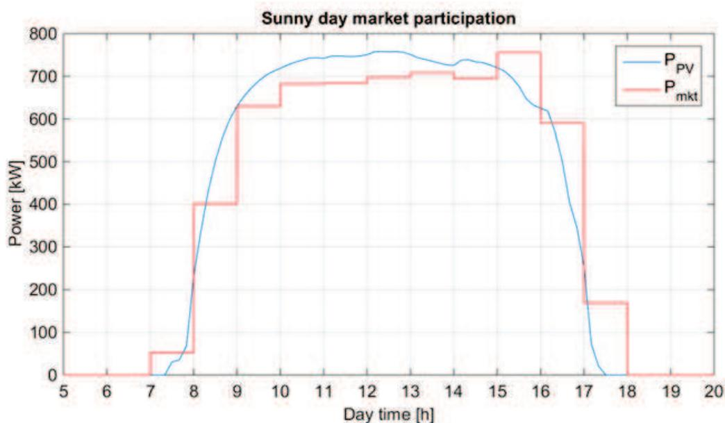
Figure 5.3: Market cleared and the PV generation inputs of the validation for a sunny day.
