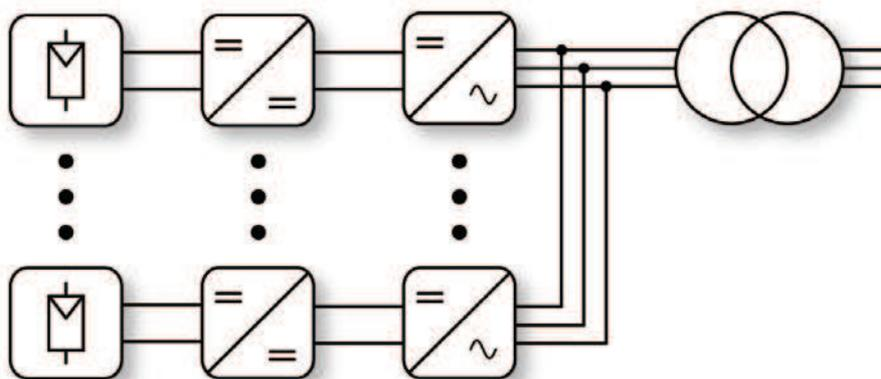
Figure 1.3: PV power plant with the modules connected in AC [14].
