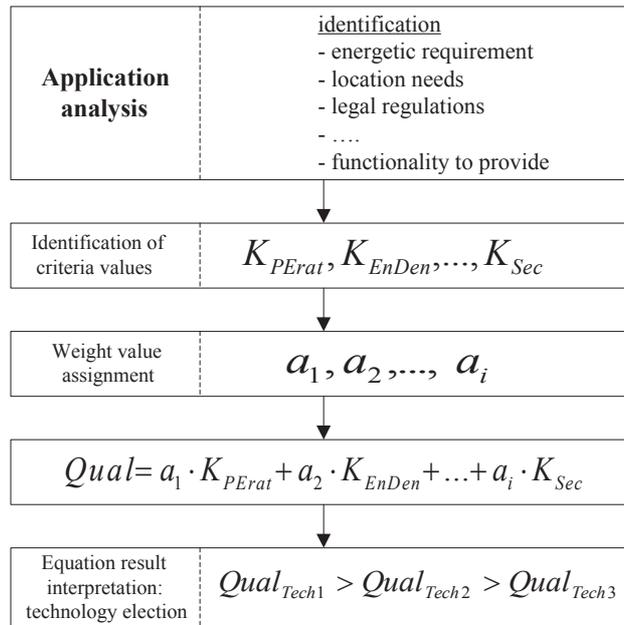
Figure 2.2: BES technologies selection methodology flowchart.
