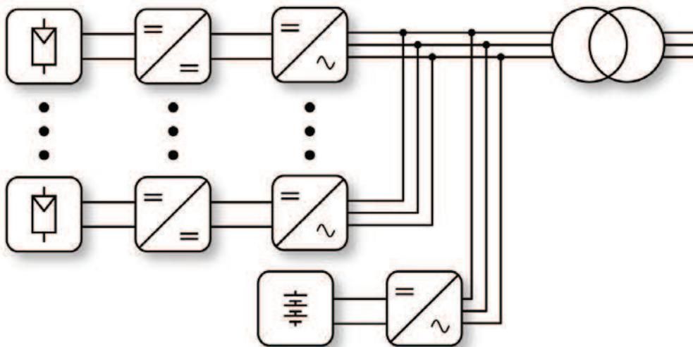
Figure 1.4: Power architecture of IPV power plant with the centralized storage connected in AC [14].
