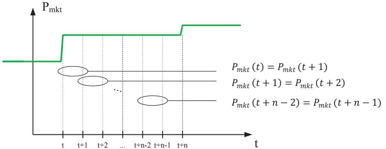
Figure 4.2: Firming service to participate in markets and the corresponding equations to model this operation mode.
