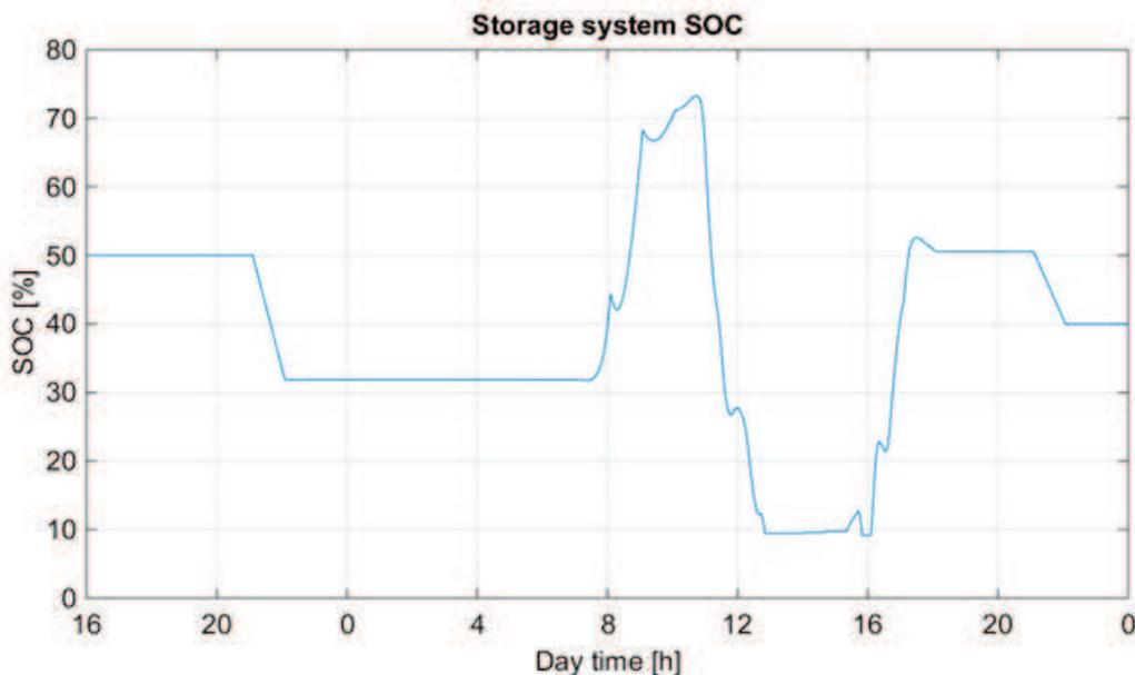
Figure 5.18: Storage system SOC variation corresponding to a cloudy day operation based on the optimal control strategy.
