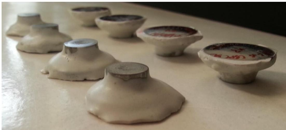
*Figure III.2. Photograph of the modified coin-cells.*
