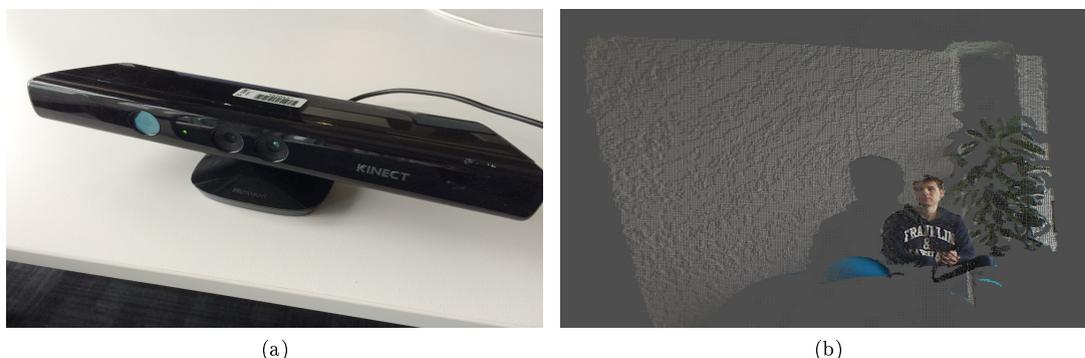
FIGURE 2.12 – (a) The Microsoft<sup>®</sup> Kinect<sup>™</sup> is an example of depth sensor that uses a structured light approach. (b) The point cloud provided by this sensor crosses the depth image with the RGB one.
