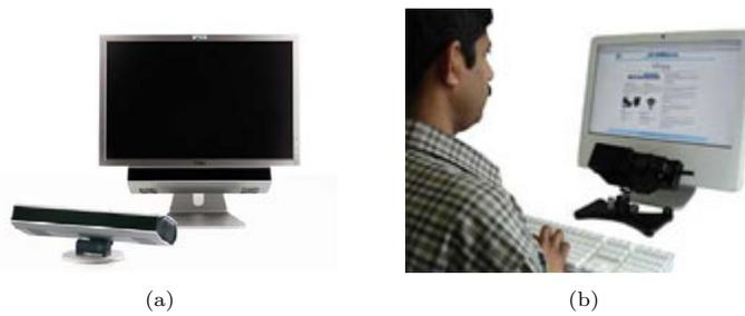
Figure 3.2: Two eye-tracking apparatus used in our experiments. (a) SMI<sup>©</sup> iView X<sup>TM</sup> RED, (b) Eye Link 1000 Remote/Head Free
