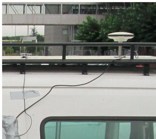
Figure 40 The U-blox antenna (left) and the NovAtel SPAN antenna (right)
