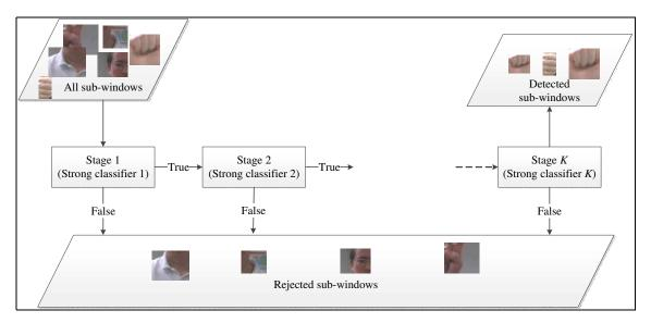
Figure 3.21 – The cascade of classifiers structure
