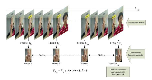
Figure 5.10 – System deployment: making decision.
