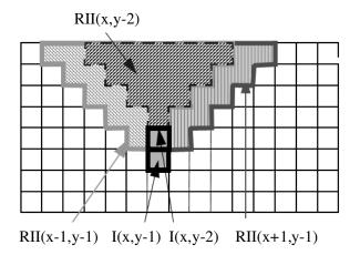
Figure 3.11 – Calculation scheme for  $45^{\circ}$  rotated integral image.
