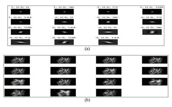
Figure 2.3 - (a) Kernel response with different scales and orientations. (b) Gabor filter response of a typical hand gesture [32]
