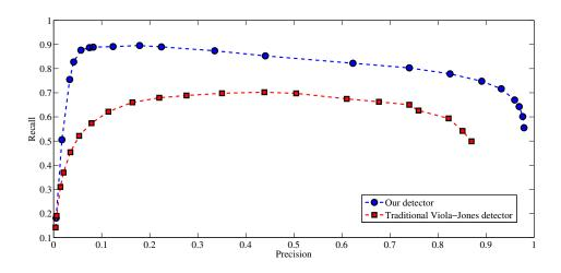
Figure 3.34 – Precision-Recall curves for comparison between our detector and traditional Viola-Jones detector.
