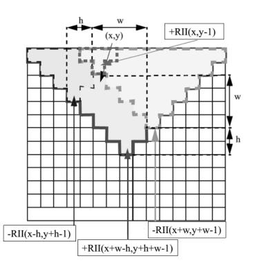
Figure 3.12 – Calculation scheme for sum of  $45^{\circ}$  rotated rectangle.
