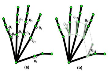
Figure 2.11 – An illustration of (a) the joint angles, and (b) the angle differences between fingers used in [20].
