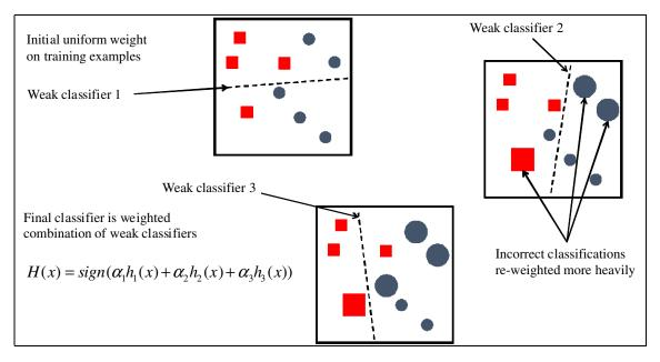
Figure 3.19 – Illustration of AdaBoost algorithm with number of weak classifiers M = 3.
