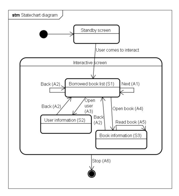
Figure 5.4 – The state chart diagram of the system
