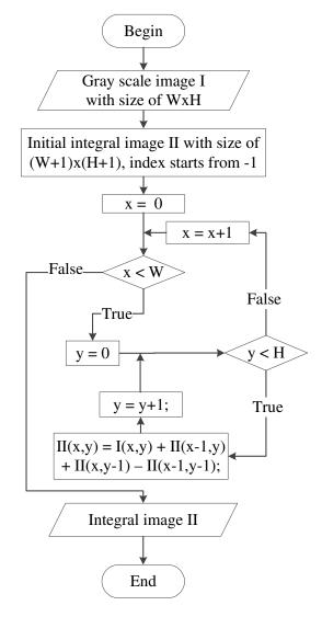
Figure 3.8 – Diagram of computation integral image.
