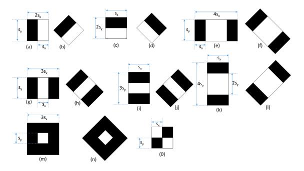
Figure 3.4 – The extended set of Haar-like features [51] used in our system.
