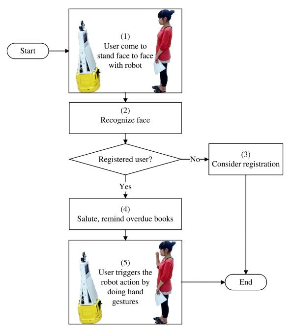
Figure 5.3 – The activity diagram of the system
