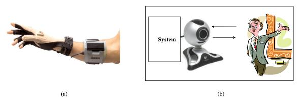
Figure 1.1 – Two main approaches for hand gesture interaction. (a) The Data-Glove based approach (An example of the Data Glove: The CyberGlove from the Immersion Corporation [1]). (b) Vision Based approach.
