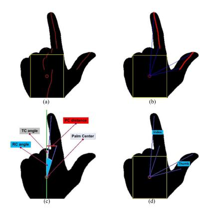
Figure 2.12 – Hand representation used in [82]. (a) Local maxima of horizontal distance transform; (b) Root and fingertips points; (c) RC, TC angles and distance from the palm center; (d) Raised fingers classification.
