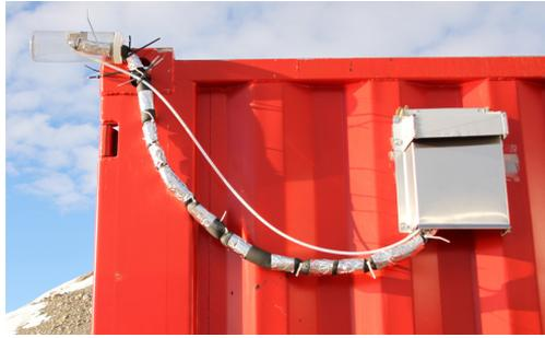
Figure 7.5: The inlet for atmospheric air during the measurement campaign. The coated tubing was heated to 50°C and thermally insulated. A plastic cover around the inlet avoided perturbations because of snow fall
