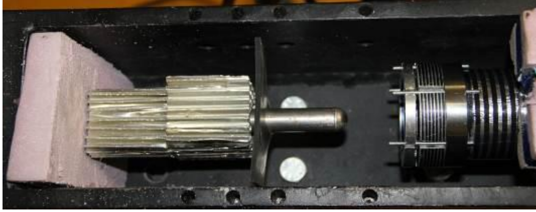
Figure 5.2 Projectile and Hopkinson pressure bar and experimental setup
