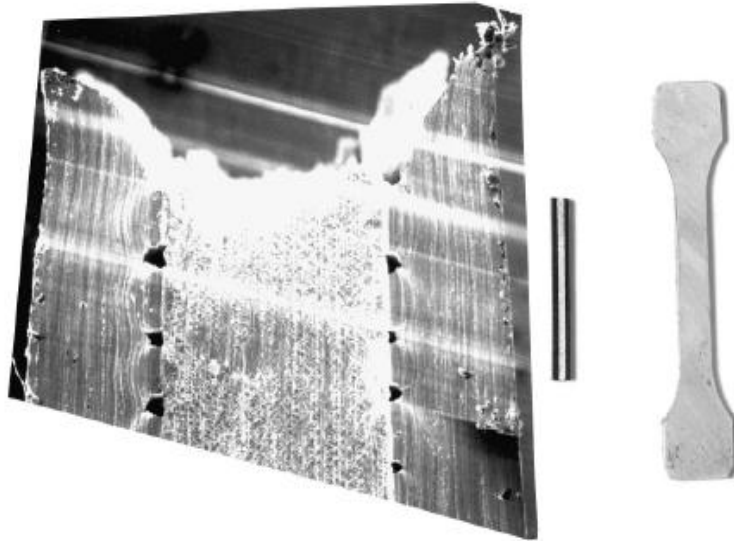
Figure 1.7 A specimen section of three-layer graded laminate sheet: 304ss/UHCS/304ss [24]
