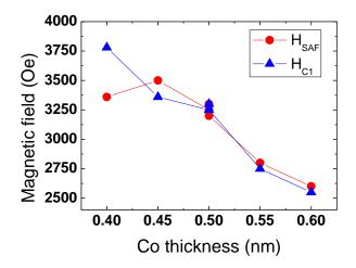
Figure II-18: Variation of the coupling field  $H_{SAF}$  and the coercive field  $H_{C1}$  of the bottom multilayer as a function of Co thickness in the Co/Pt multilayers.
