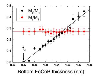
Figure IV-7: Normalized magnetizations  $M_b/M_1$  and  $M_t/M_1$  as functions of bottom FeCoB thickness for junctions consisting of SAF<sub>1</sub>/MgO/FeCoBx/Ta0.2/Ru0.5/FeCoB1.1/MgO.
