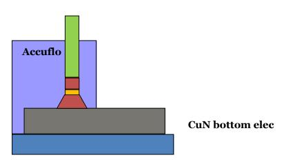
Figure V-12: Thinning down of the Accuflo to a thickness around 90-130 nm in order to free the top part of the Ta pillar.
