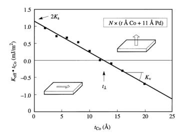
Figure I-2: Example of a plot of K<sub>eff</sub>.t as a function of t for Co/Pd multilayers [Joh-96].
