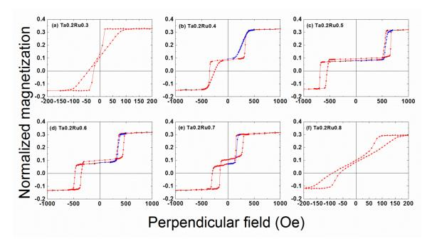
Figure IV-3: Magnetic loops measured by VSM with perpendicular applied field for samples with standard bottom SAF reference and a composite FeCoB1.4/Ta0.2Rux/FeCoB1.1 storage layer. Values of x are: (a) 0.3 (b) 0.4 (c) 0.5 (d) 0.6 (e) 0.7 (f) 0.8 nm. Only zooms on the storage layers are shown.
