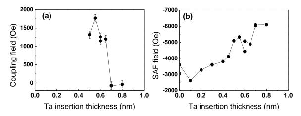
Figure II-8: Evolution of (a) the coupling field of the FeCoB layer and (b) the SAF field as a function of Ta insertion thickness.
