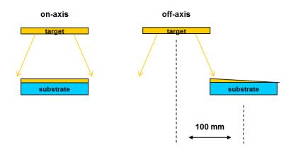
Figure I-11: Schematic representation of the two possible geometries in our deposition tool.
