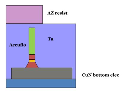
Figure V-10: Deposition of the positive AZ resist and optical lithography to define an insulating zone around the pillar.
