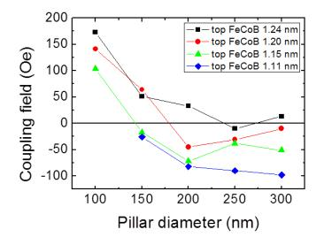
Figure V-17: Coupling field acting on the storage layer as a function of pillar diameter for different thicknesses of the top FeCoB layer.
