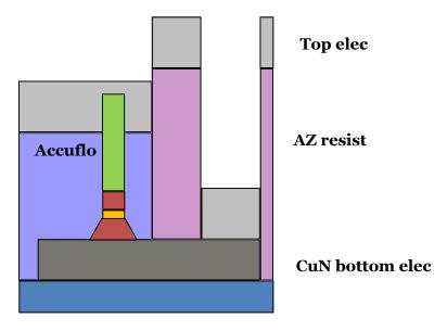
Figure V-14: Deposition of the Cr/Al metallic contacts by evaporation to create the top electrode.
