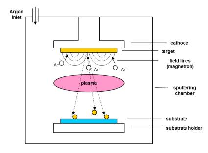
Figure I-9: Schematic representation of a sputtering chamber.
