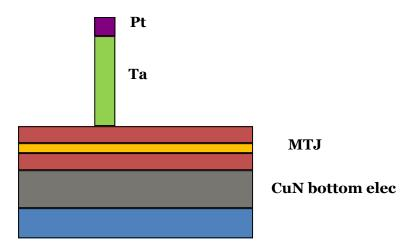
Figure V-5: Reactive ion etching of the Ta hard mask. The parts under the Pt are protected.
