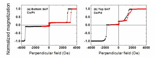
Figure III-20: Comparison of the magnetic loops of two junctions with (a) a bottom Co/Pt SAF reference (b) a top Co/Pd SAF reference.
