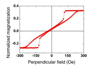
Figure III-2: Minor loop performed on the free layer by VSM with a perpendicular applied field for a sample with a FeCoB1.5/Tao.3/FeCoB1.5/MgO storage layer.
