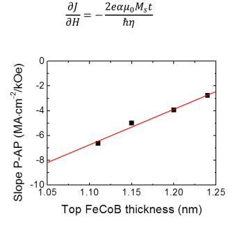
Figure V-20: Slope of the P-AP transition as a function of top FeCoB thickness for 150 nm pillars.
