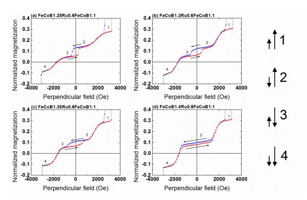
Figure IV-10: Magnetic cycles of  $SAF_1/MgO/FeCoBx/Ru0.6/FeCoB1.1/MgO/Pt2$  structures measured by VSM with perpendicular applied field. 4 different thicknesses of bottom FeCoB are shown: (a) 1.25 (b) 1.3 (c) 1.35 and (d) 1.4 nm. The magnetic configurations labelled 1 to 4 on the graphs are schematically represented on the right.
