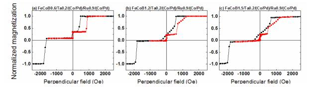
Figure III-15: Magnetic cycles measured by VSM with perpendicular applied field for junctions having varying thickness of FeCoB in the top SAF reference, Ta3/FeCoB1.2/MgO/FeCoBx/Ta0.2/(Co0.3/Pd1.2)<sub>4</sub>/Co0.3/Rux/(Co0.3Pd1.2)<sub>8</sub>/Co0.3/Pd2. (a) x=0.6 nm (b) x=1.2 nm (c) x=1.5 nm.
