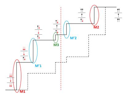
Figure III-22: Schematic representation of the major loop of a double junction. The black line corresponds to the descending branch coming from positive field saturation while the black dotted line shows the ascending branch. The red dotted line symbolizes H=0.
