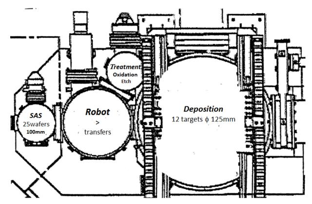
Figure I-10: Plan of the Actemium deposition tool showing the organization of the different chambers.
