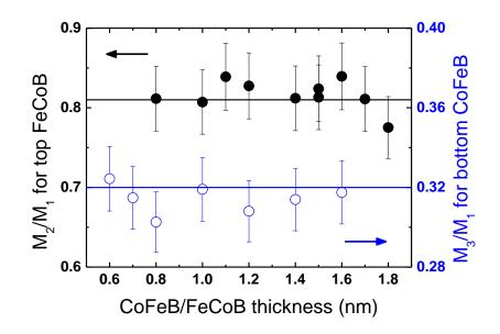
Figure II-29: Magnetization ratio of the constant magnetic contributions  $M_2/M_1$  as a function of top FeCoB thickness, filled black circles, left-hand scale, and  $M_3/M_1$  as a function of bottom CoFeB thickness, open blue circles, right-hand scale. Horizontal lines correspond to the theoretical values, 0.81 and 0.32, respectively.
