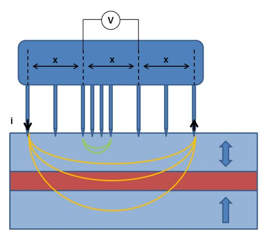
Figure I-16: Schematic representation of the CIPT technique.
