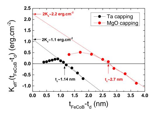
Figure III-5: Variation of  $K_{\rm eff}$  t as a function of effective thickness for top FeCoB electrodes capped with Ta or MgO.
