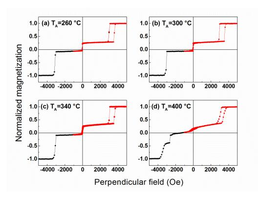
Figure II-23: Magnetic loops measured by VSM with perpendicular applied field for standard perpendicular junctions with Coo.5/Pto.25 multilayers in the bottom SAF. Three different annealing temperatures are presented: (a)  $260 \degree C$  (b)  $300 \degree C$  (c)  $340 \degree C$  and (d)  $400 \degree C$ .
