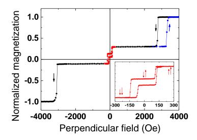
Figure IV-1: Magnetic loop measured by VSM with perpendicular applied field for a junction with bottom SAF reference and a top SAF storage layer made of FeCoB1.2/Tao.8/FeCoB1.2/MgO.
