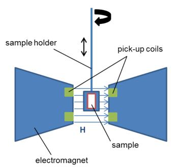
Figure I-12: Working principle of a VSM.
