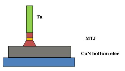
Figure V-8: Ion beam etching of the bottom electrode down to the substrate. The part protected by the resist is not etched. The resist is afterwards removed.
