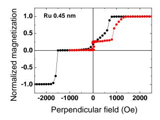
Figure III-14: Magnetic cycle measured by VSM with perpendicular applied field for a junction with top Co/Pd SAF reference, a Ru spacer of 0.45 nm and a bottom free layer of 1.2 nm of FeCoB. A minor loop is performed by saturating the system in a negative field of -1000 Oe and increasing it towards positive field saturation (red dots).
