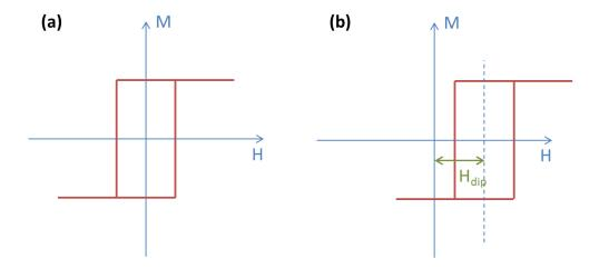
Figure II-11: Schematic representation of the magnetic loop of the storage layer in the case of (a) no dipolar coupling and (b) a dipolar coupling.  $H_{dip}$  corresponds to the amplitude of the shift of the hysteresis loop.
