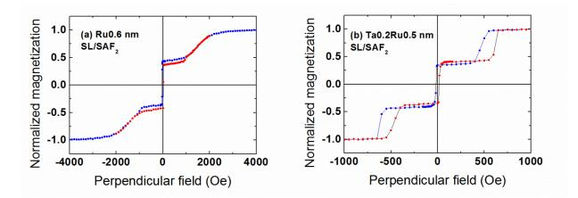
Figure IV-17: Magnetic cycles measured by VSM with perpendicular applied field for single junctions with a bottom storage layer SL=Ta3/FeCoB1.2 and a top reference that is either (a) FeCoB1.4/Ru0.6/FeCoB1.1/MgO or (b) FeCoB1.4/Ta0.2/Ru0.5/FeCoB1.1/MgO.
