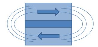
Figure II-12: Schematic representation of a planar SAF.
