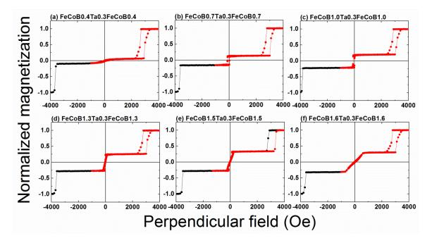
Figure III-1: Magnetic loops measured by VSM with perpendicular applied field for samples with a bottom SAF reference and varying thickness of FeCoB in the top electrode capped with MgO. The total FeCoB thickness goes from 0.8 (a) to 3.2 nm (f).
