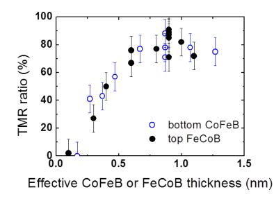
Figure II-32: TMR ratio as a function of bottom CoFeB (blue open circles) and top FeCoB (black filled circles) thicknesses, respectively, after subtraction of their corresponding dead layer thicknesses.
