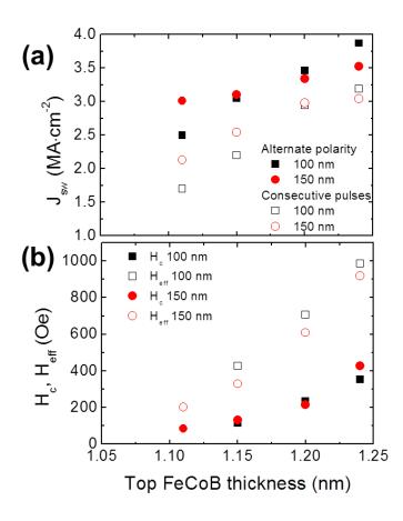
Figure V-18: (a) Critical current density  $J_{sw}$  for STT switching as a function of top FeCoB thickness. Results are shown for two pillar sizes, 100 nm (squares) and 150 nm (circles) and for the two measurement techniques, alternate polarity (solid symbols) and consecutive pulses (open symbols). (b) Coercive field  $H_c$  (solid symbols) and anisotropy field  $H_{eff}$  (open symbols) as a function of top FeCoB thickness.
