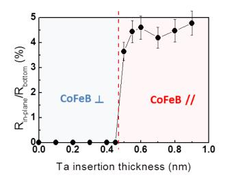
Figure II-4: Relative Hall contribution of the in-plane component of the bottom electrode as a function of Ta insertion thickness.
