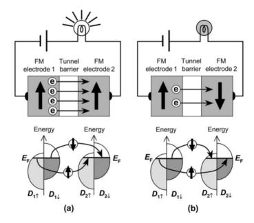
Figure I-4: Schematic representation of the tunnel magnetoresistance effect for (a) parallel configuration of the magnetizations (b) antiparallel configuration of the magnetizations [Yua-07].
