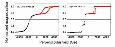
Figure III-11: Magnetic cycles measured by VSM with perpendicular applied field for SAF composed of (a) Ta3/(Co0.5/Pt0.25)<sub>3</sub>/Co0.5/Ru0.9/(Co0.5/Pt0.25)<sub>5</sub>/Co0.5/Pt2 and (b) Ta3/(Co0.3/Pd1.2)<sub>3</sub>/Co0.3/Ru0.9/(Co0.3/Pd1.2)<sub>5</sub>/Co0.3/Pd2. Minor loops are included in red.
