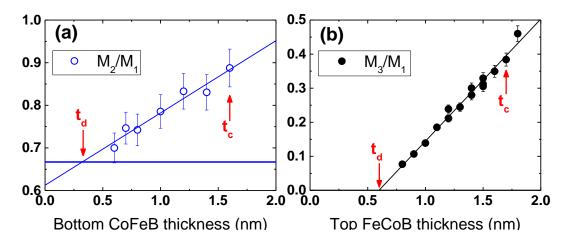
Figure II-27: Magnetization ratio  $M_2/M_1$  as a function of bottom CoFeB thickness (a) and  $M_3/M_1$  as a function of top FeCoB thickness (b). The horizontal line on the left graph corresponds to the ratio  $M_2/M_1$  for zero CoFeB thickness, that is to say 2/3.
