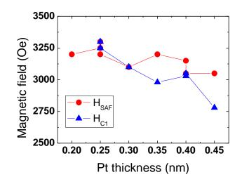
Figure II-20: Variation of the coupling field  $H_{SAF}$  and the coercive field  $H_{C1}$  of the bottom multilayer as a function of Pt thickness in the Co/Pt multilayers.
