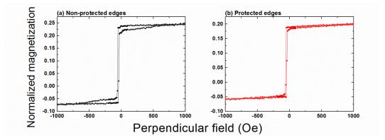
Figure I-14: Magnetic loops measured by VSM with perpendicular applied field on standard magnetic tunnel junctions with (a) non-protected or (b) protected edges.
