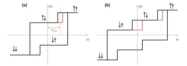
Figure II-14: Schematic hysteresis loops of a SAF in the case where (a) the RKKY coupling energy is smaller than the Zeeman and anisotropy contributions (b) the opposite situation. We add in red minor loops.
