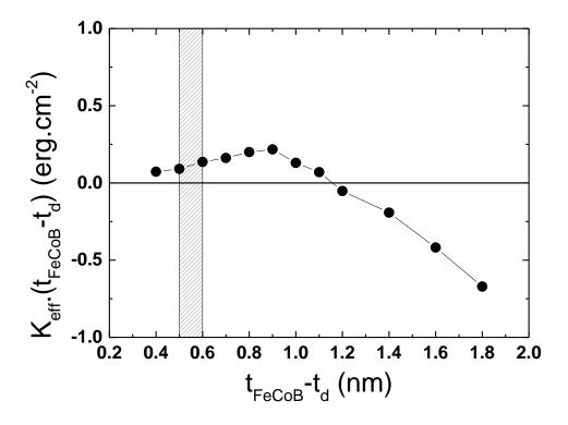
Figure V-19: Variation of the K<sub>eff</sub>t product as a function of effective thickness for top FeCoB layers capped with Ta. The dashed region corresponds to the thickness range present on our patterned sample.
