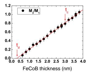
Figure III-3: Magnetization of the FeCoB storage layer with a 0.3 nm Ta insertion as a function of its nominal thickness for junctions with a bottom SAF reference and an MgO capping.  $t_c$  and  $t_d$  stand for dead layer and critical thicknesses, respectively. The magnetization  $M_3$  of the storage layer is normalized to the magnetization  $M_1$  of the bottom part of the SAF (internal reference).
