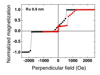
Figure III-12: Magnetic cycle measured by VSM with perpendicular applied field for a junction with top Co/Pd SAF reference, a Ru spacer of 0.9 nm and a bottom free layer of 1.2 nm of FeCoB. A minor loop is performed by saturating the system in a negative field of -1000 Oe and increasing it towards positive field saturation (red dots).
