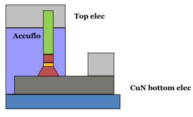
Figure V-15: Final lift-off of the resist.
