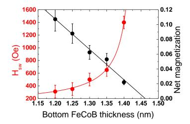
Figure IV-11: Switching field  $H_{sw}$  of the additional transition (in red) and net magnetization normalized to  $M_1$  (in black) as a function of the bottom FeCoB thickness for SAF<sub>1</sub>/MgO/FeCoBx/Ruo.6/FeCoB1.1/MgO/Pt2 magnetic tunnel junctions.
