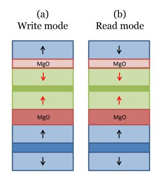
Figure IV-15: Schematic representation of the write (a) and read (b) modes in the case of double junctions with the following structure:  $SAF_1/MgO/SAF_3/MgO/SL$ , SL standing for the soft control layer.
