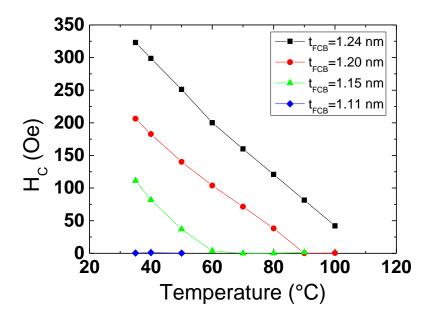
Figure V-21: Variation of the coercive field  $H_{\rm c}$  as a function of the temperature for 100 nm pillars with varying thickness of the top FeCoB storage layer.
