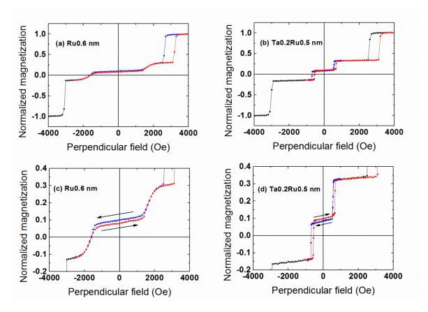
Figure IV-9: Magnetic cycles measured by VSM with perpendicular applied field for samples composed of SAF<sub>1</sub>/MgO/FeCoB1.4/spacer/FeCoB1.1/MgO/Pt2. The spacer is either Ru0.6 (a, c) or Ta0.2/Ru0.5 (b, d). Curves (c) and (d) are zooms of the top SAF.
