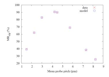
Figure I-17: Example of the evolution of the  $MR_{cip}$  as a function of the probe distance for a standard planar junction. The curve includes both the experimental data points and the fit of the CIPT tool.
