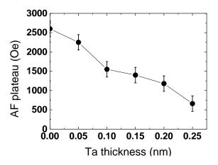
Figure IV-6: Variation of the width of the antiparallel plateau as a function of Ta insertion thickness for junctions made of  $SAF_1/MgO/FeCoB1.4/Tax/Ruy/FeCoB1.1/MgO$ . y is adjusted to keep the maximum coupling amplitude.
