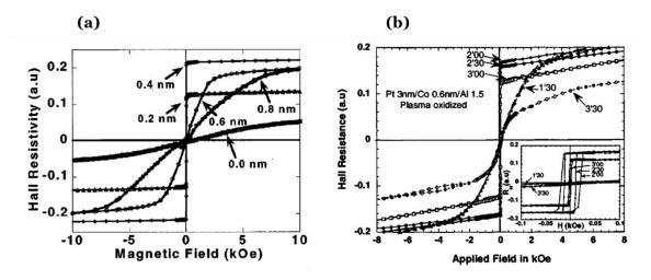
Figure I-1: Hall resistance as a function of perpendicular applied field for (a) Pt<sub>3</sub>/CoFeo.6/AlOx samples naturally oxidized in air with varying thicknesses of Al [Mon-02] (b) Pt<sub>3</sub>/Coo.6/AlOx samples plasma oxidized with different oxidation times [Rod-03].
