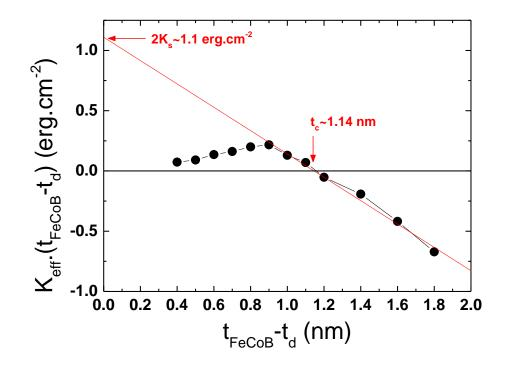
Figure II-30: Variation of  $K_{eff}$  as a function of effective thickness for top FeCoB electrodes capped with Ta.
