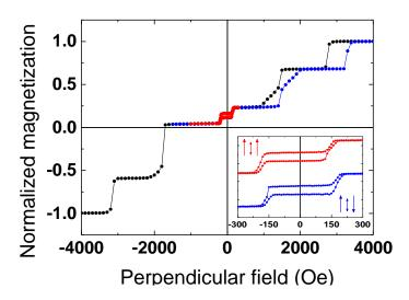
Figure IV-13: Magnetic cycle measured by VSM with perpendicular applied field for a double junction with  $SAF_1/MgO/FeCoB1.2/Tao.8/FeCoB1.2/MgO/SAF_2$ . The inset shows minor loops recorded with either parallel (red) or antiparallel (blue) configuration of the reference layers.
