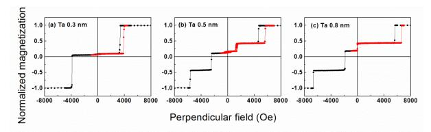
Figure II-7: Magnetic loops measured with perpendicular field for bottom SAF with increasing thicknesses of Ta insertion ( $x_{Ta}$ =0.3 (a), 0.5 (b) or 0.8 nm (c)). Minor loops on the top part of the SAF are included in red.
