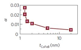
Figure I-8: Variation of damping parameter a as a function of CoFeB thickness [Ike-10].
