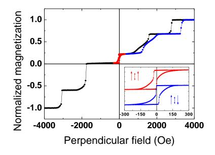
Figure III-21: Magnetic cycle measured by VSM with perpendicular field for a double junction with a FeCoB1.1/Tao.3/FeCoB1.1 storage layer. The inset shows minor loops performed on the free layer with either parallel (red) or antiparallel (blue) configuration of the reference layers.
