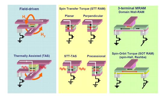
Figure I-7: Schematic representation of the different generation of MRAMs [Die-15].
