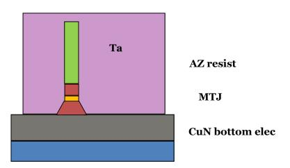
Figure V-7: Deposition of a positive resist (AZ) and optical lithography to define the bottom electrode.
