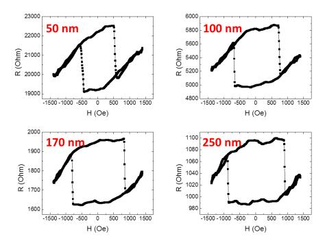
Figure IV-19: Resistance as a function of applied field for SAF<sub>1</sub>/SAF<sub>2</sub> structures patterned into circular nanopillars of different diameters.
