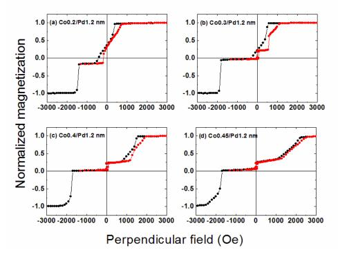
Figure III-17: Magnetic cycles measured by VSM with perpendicular applied field for samples with varying thickness of Co in the top Co/Pd SAF reference. (a) 0.2 nm (b) 0.3 nm (c) 0.4 nm (d) 0.45 nm.
