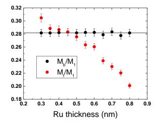
Figure IV-4: Normalized magnetizations  $M_b/M_1$  and  $M_t/M_1$  as a function of Ru thickness for junctions with bottom SAF reference and FeCoB1.4/Tao.2/Rux/FeCoB1.1/MgO top storage layer.
