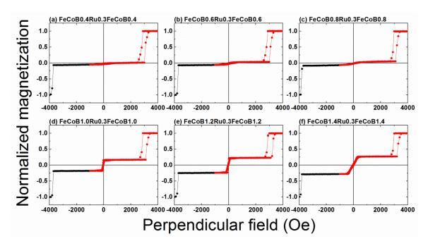
Figure III-6: Magnetic loops measured by VSM with perpendicular applied field for samples with a bottom SAF reference and varying thickness of FeCoB in the top electrode capped with MgO. The total FeCoB thickness goes from 0.8 (a) to 2.8 nm (f).
