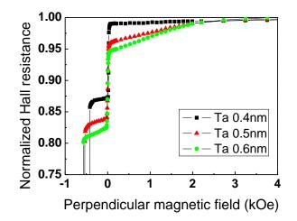
Figure II-3: Partial EHE loop performed on samples with x<sub>Ta</sub>=0.4, 0.5, and 0.6 nm.
