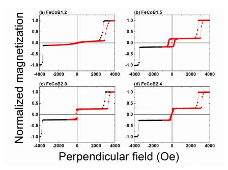
Figure III-8: Magnetic loops measured by VSM with perpendicular applied field for samples with a bottom SAF reference and varying thickness of FeCoB in the top electrode capped with MgO. (a) FeCoB1.2 (b) FeCoB1.5 (c) FeCoB2.0 (d) FeCoB2.4.
