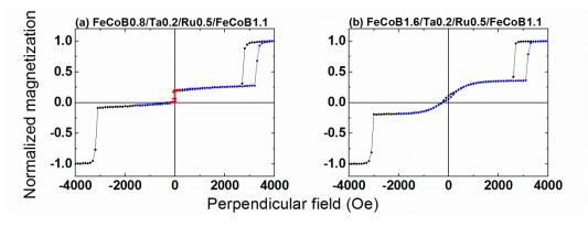
Figure IV-8: Magnetic loops measured by VSM with perpendicular applied field for samples with standard bottom SAF reference and a composite FeCoBx/Tao.2/Ruo.5/FeCoB1.1 storage layer. Examples with (a) thin 0.8 nm and (b) thick 1.6 nm bottom FeCoB layers are shown.
