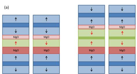
Figure IV-12: Schematic magnetic configurations optimizing STT efficiency in perpendicular double magnetic tunnel junctions: (a) antiparallel references and single ferromagnetic storage layer, (b) parallel references and synthetic antiferromagnetic storage layer.
