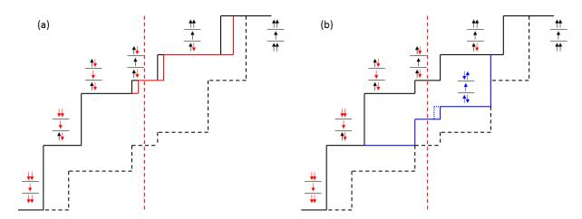
Figure III-23: Schematic representations of the field treatments needed to perform the minor loop on the free layer with (a) parallel or (b) antiparallel configuration of the references.
