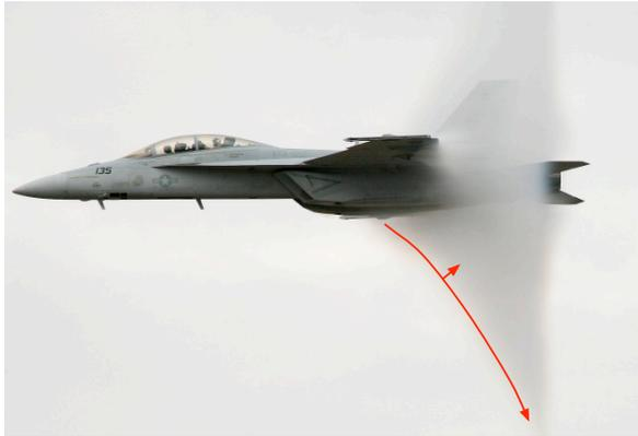
(a) Mach cone around a F-15. In red: the directions of anisotropy of the shock wave.
