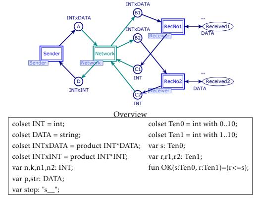
Figure 4.13 – Root net of the hierarchical protocol model
