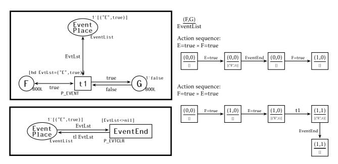
Figure 3.33 – Event-driven coloured Petri net model of Fig. 3.29
