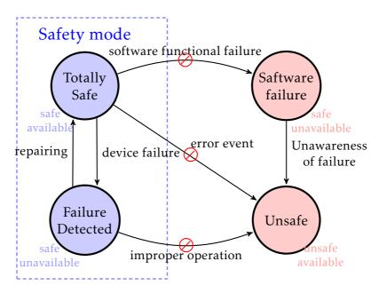
Figure 2.3 – The overall safety of a computer-controlled signalling system
