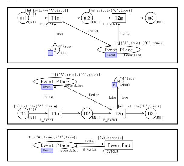
Figure 3.31 – Event-driven coloured Petri net model of Fig. 3.28
