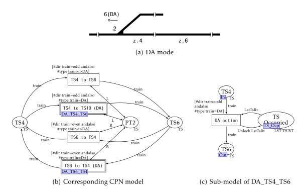
Figure 3.20 – A Petri net representation of "DA" mode
