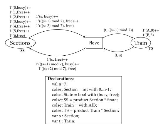
Figure 3.4 – A non-hierarchical coloured Petri net example
