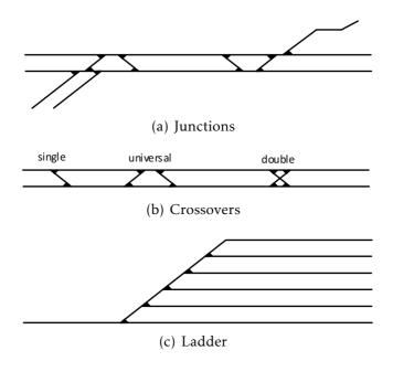
Figure 2.8 – Basic point arrangements
