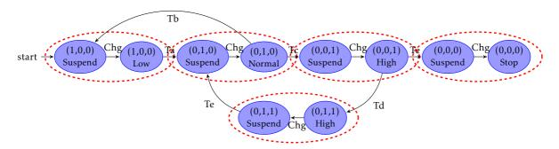
Figure 4.20 – The state-space of *B* machine "Prioritized\_Transitions"
