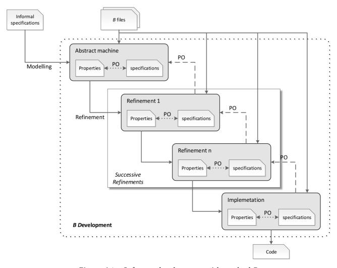
Figure 4.1 – Software development with method *B*
