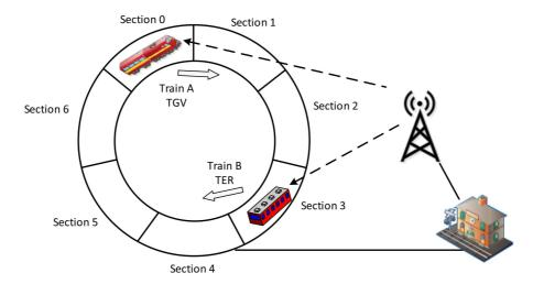
Figure 3.9 – A circular railway network with a signal centre and train priorities
