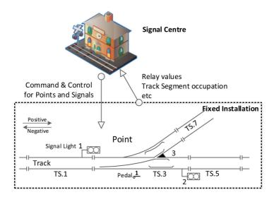
Figure 2.10 – An example of railway interlocking system
