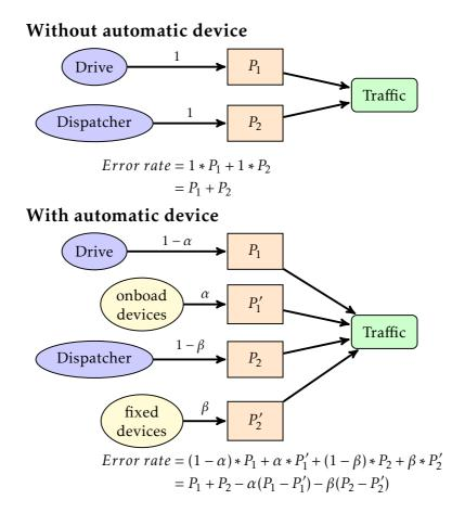
Figure 2.5 – The effect of the automatic devices in system safety
