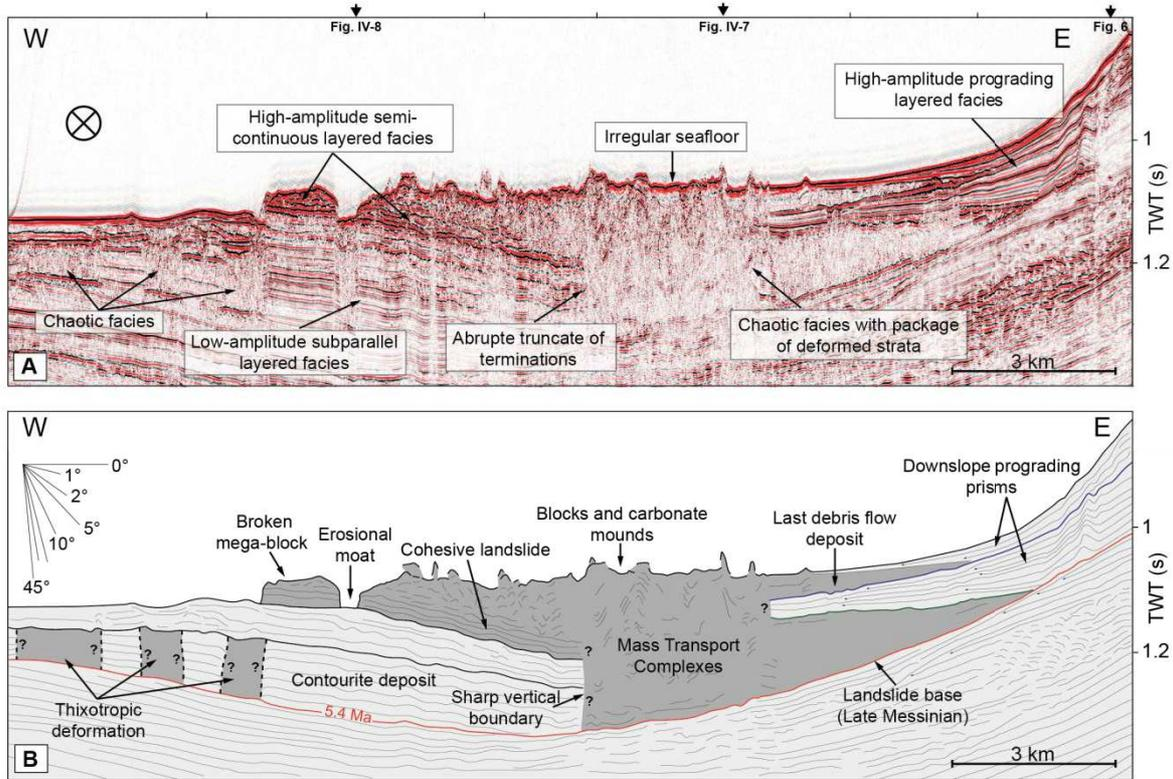
**Figure IV-10:** Dip-oriented seismic profile (see Fig. IV-2 for location) showing the northern basinward limit of the MTCs and its contact with the contourite. Note the irregular seafloor and the presence of a large kilometer-sized broken megablock in the toe domain. The basal décollement surface shows an asymmetrical concave-shape morphology, overlain by an elongated mounded-shape contourite with a steep landward lee-side on which the MTD pulls up and “emerges” to the surface.
