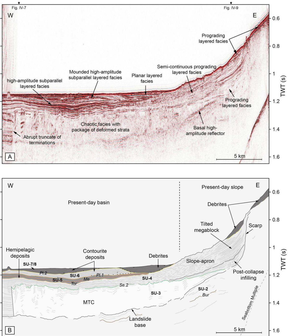
**Figure IV-10:** A) Uninterpreted and B) interpreted E-W-oriented seismic profile (see Fig. IV-3 for location) illustrating the dip geometries and the termination relationships of seismic facies in a basinward direction.
