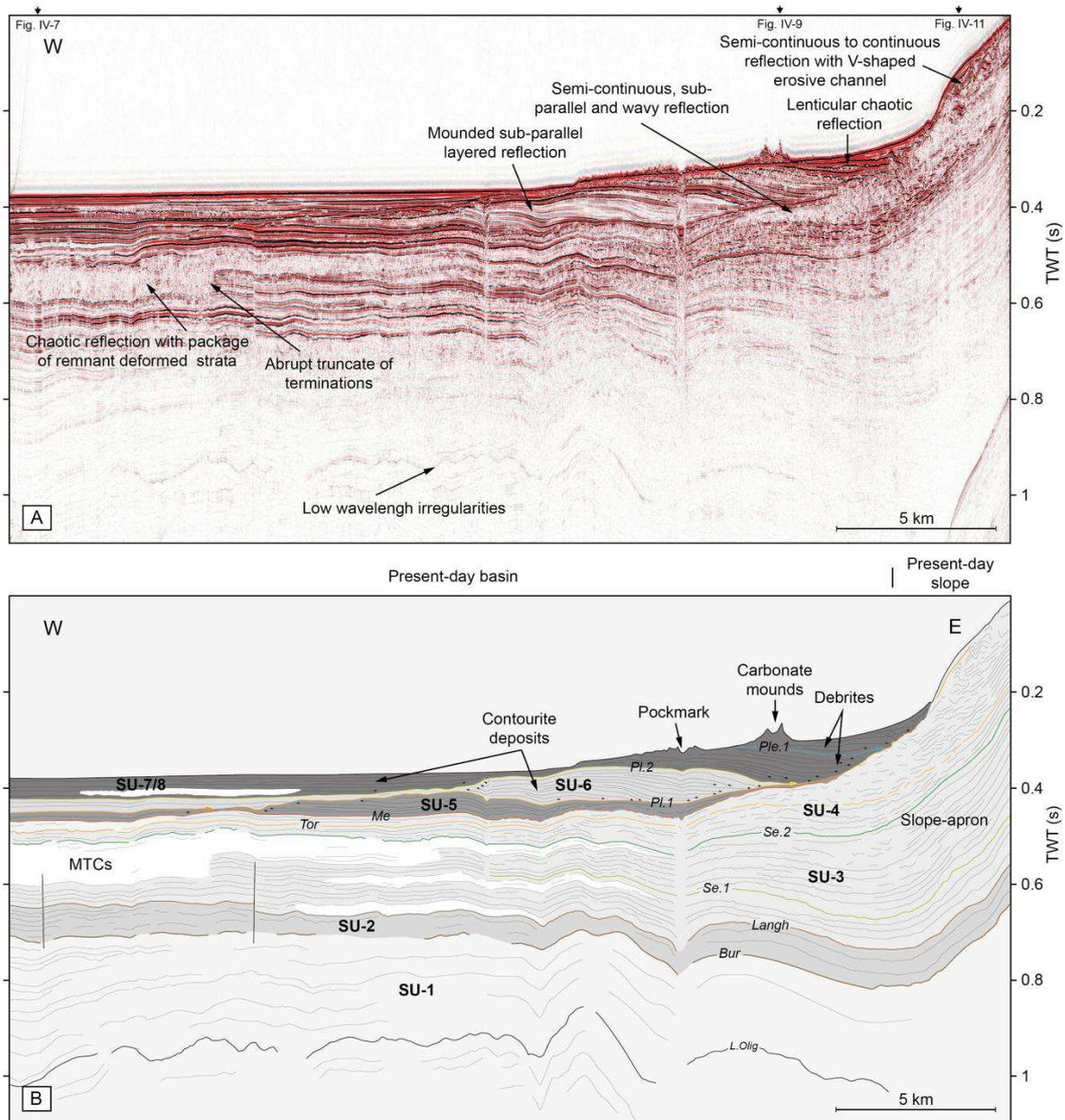
**Figure IV-8:** A) Uninterpreted and B) interpreted E-W-oriented seismic profile (see Fig. IV-3 for location) illustrating the dip geometries and the termination relationships of seismic facies in a basinward direction.
