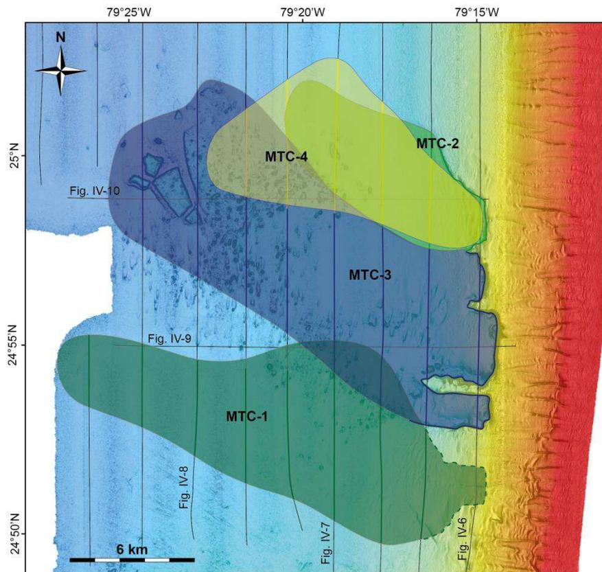
**Figure IV-11:** Map showing areal distribution of the MTCs and their associated failure scars on the western slope of the GBB, based on the overall multichannel seismic reflection lines (plain black lines).
