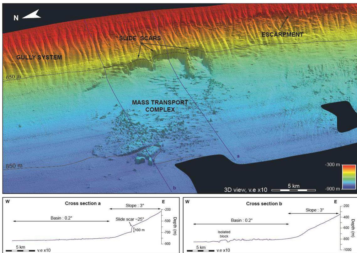
**Figure IV-3:** 3D view of the Mass Transport Complex facing west toward the headwall area with a vertical exaggeration of  $\times 10$ . Prominent features include a gully system extending in a great escarpment toward the south on the upper slope and a wide failure scarp and its associated Mass Transport Complex in the basin. (a) & (b) show the location of 2 cross sections through the MTC area.
