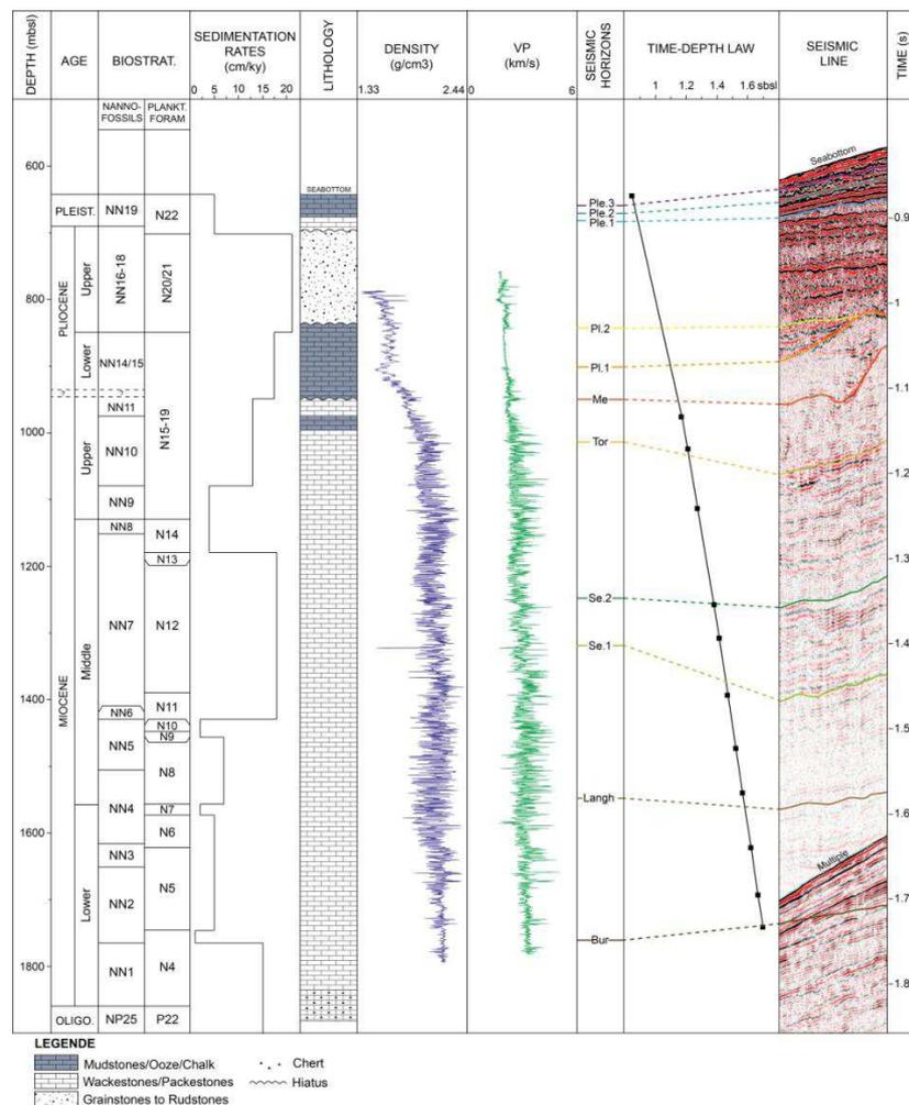
**Figure IV-5:** Well-to-seismic tie for establishment of a chronostratigraphy. Age, biostratigraphy, sedimentation rates, lithology, density and Vp log data and time-depth law are from ODP well 1007 (Eberli *et al.*, 1997). The seismic line is from the Carambar cruise (Mulder *et al.*, 2012).
