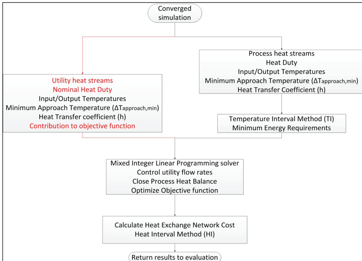
Figure 1:6 Breakdown of employed methodology for synthesis of optimal heat exchange network
