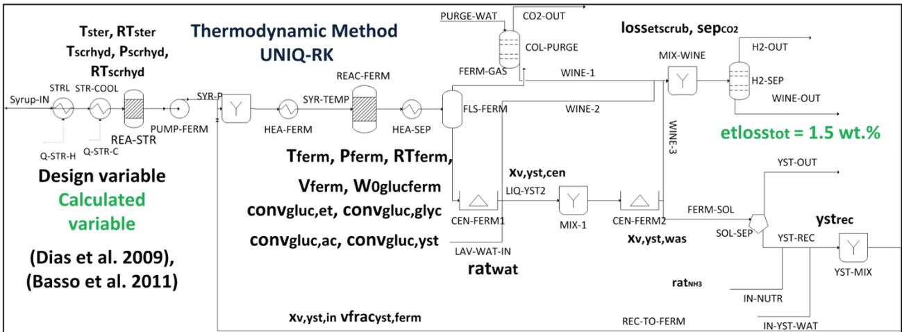
Figure 2:4 Process Flow Diagram fermentation section
