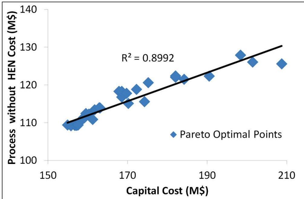
Figure 4:16 Process Cost vs. Capital Cost for Pareto optimal solutions
