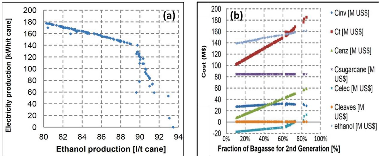
Figure 5:3 (a) Results of multi-objective optimization work applied on the studied process and (b) Evolution of costs of various components with fraction of bagasse sent to hydrolysis [21]
