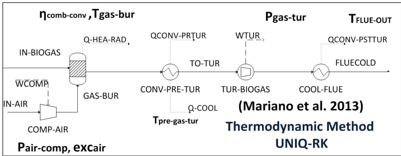
Figure 3:8 Process Flow Diagram for gas turbine section
