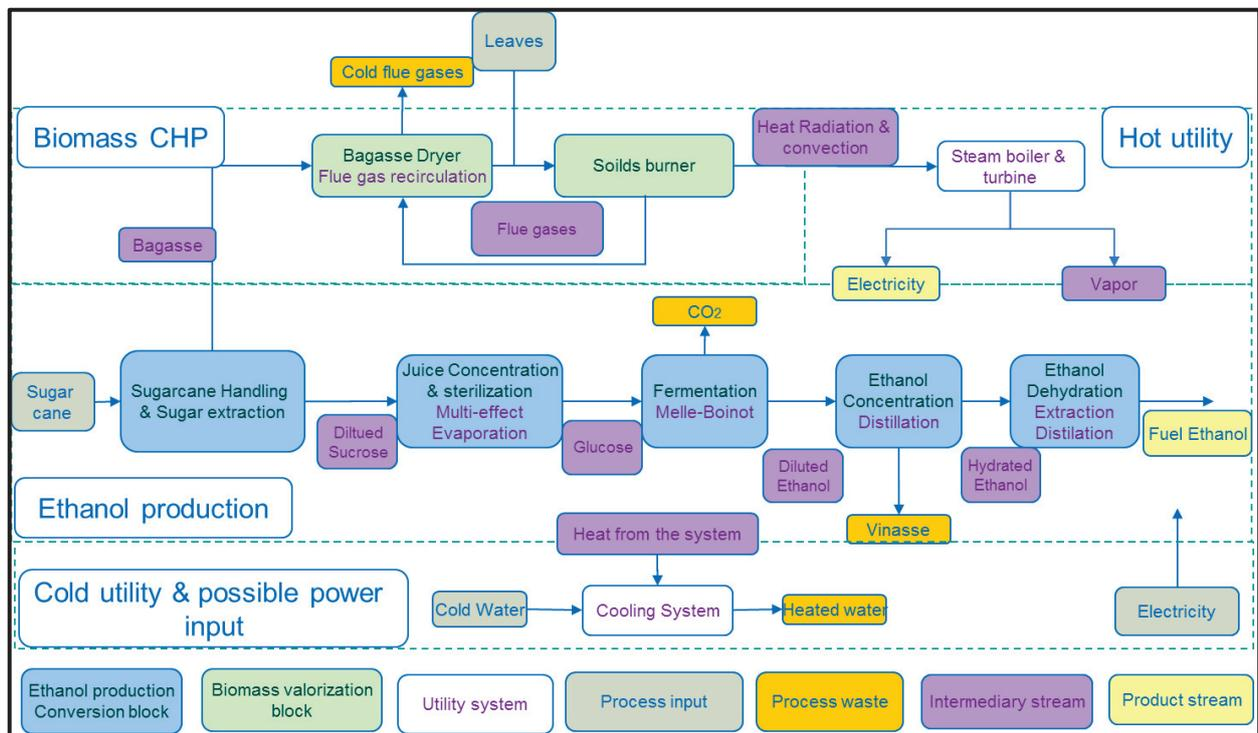
Figure 4:2 Block Flow Diagram for ethanol and power from sugarcane production process
