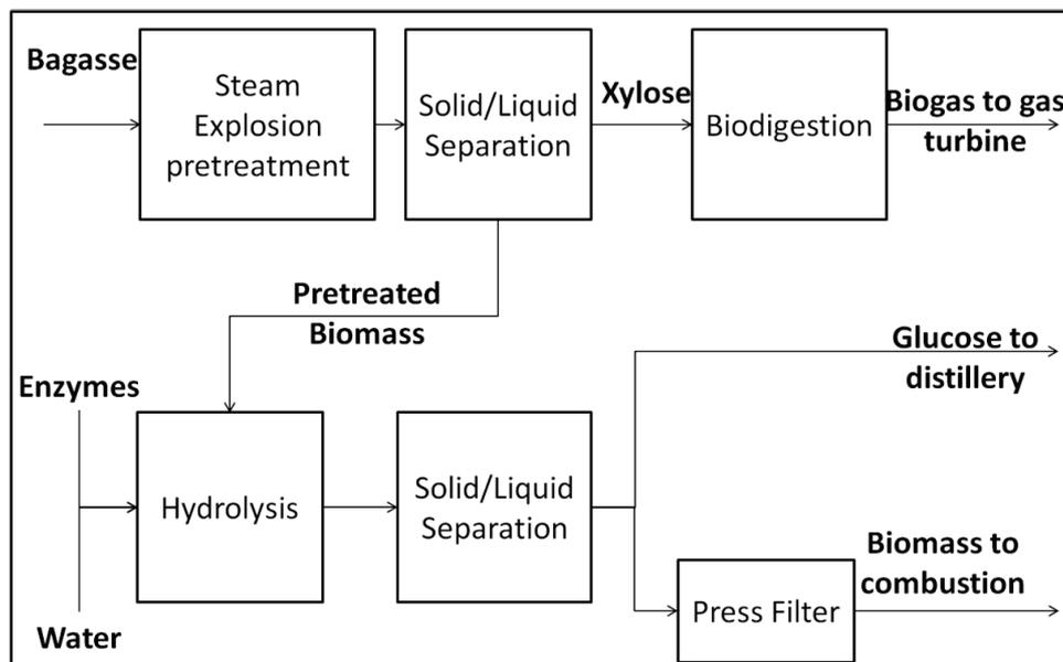
Figure 3:2 Block Flow Diagram for chosen bagasse hydrolysis scheme
