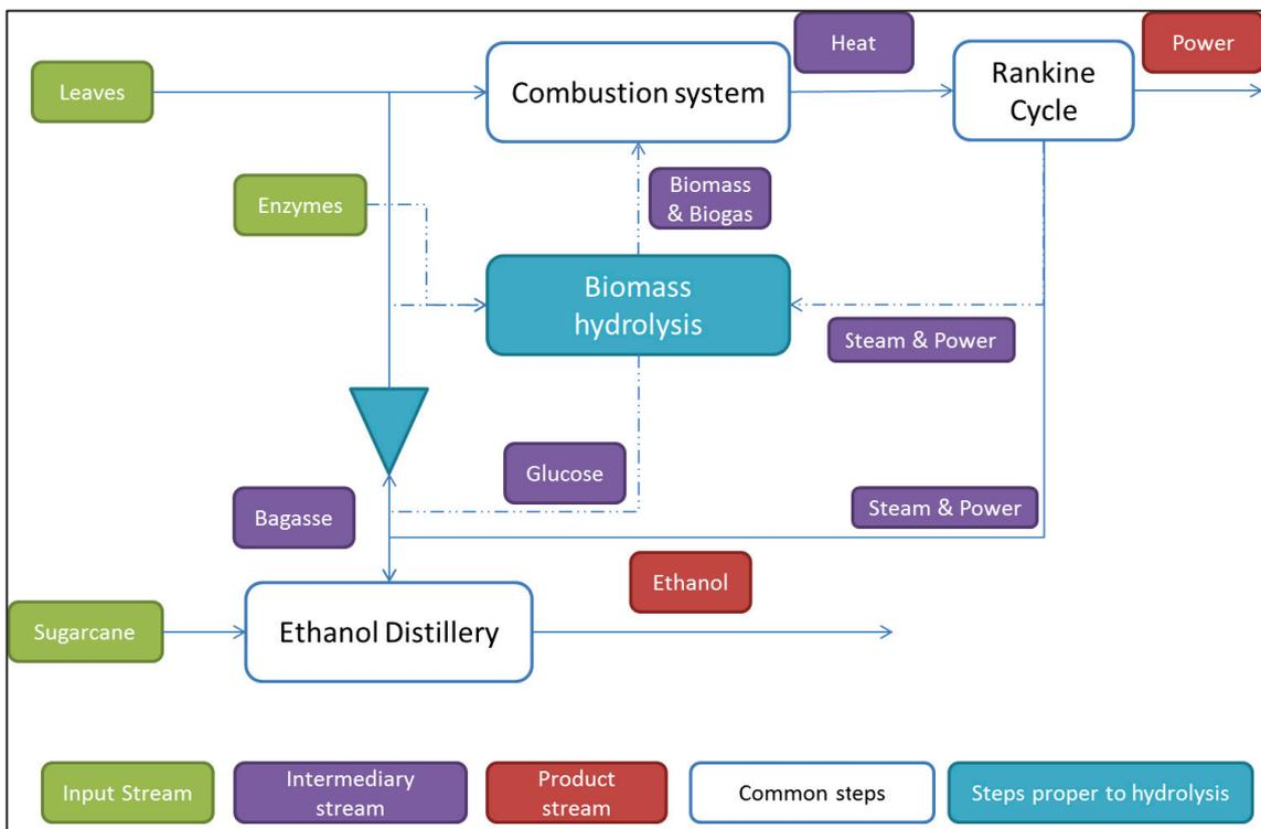
Figure 2 Block diagram for the two studied processes
