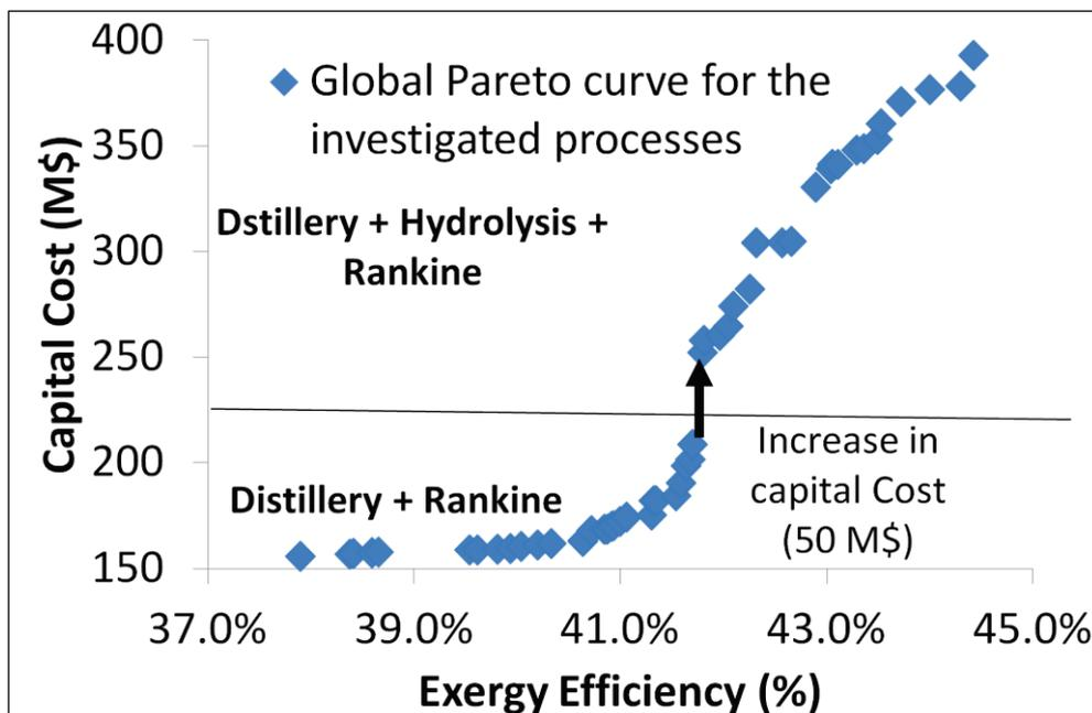
Figure 5:18 Pareto curve combining Pareto-optimal results for distillery + Rankine cogeneration + hydrolysis systems
