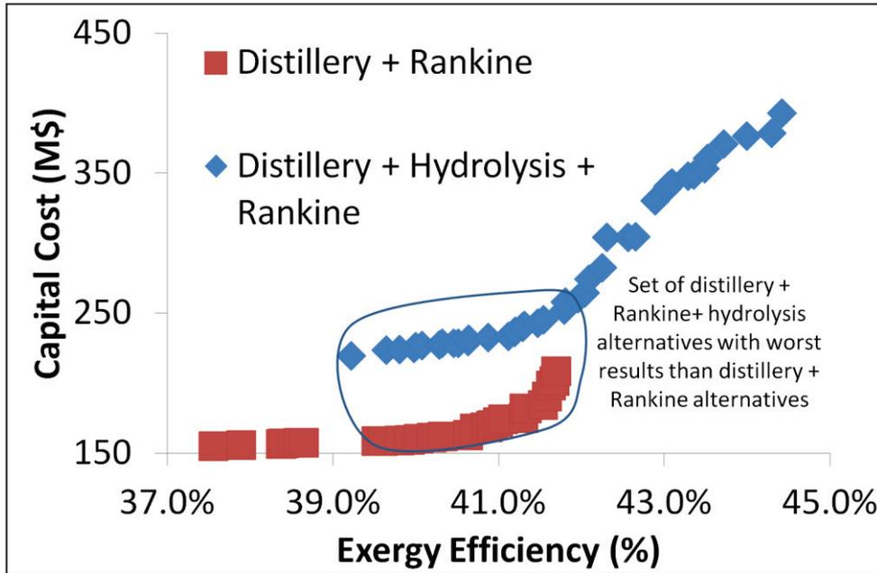
Figure 5:17 Comparison between Pareto results for distillery + Rankine cogeneration and distillery + Rankine cogeneration + hydrolysis cases
