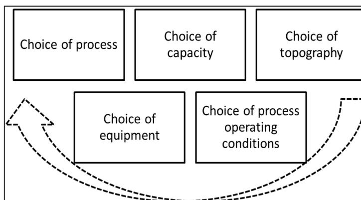
Figure 1:1 Elements of process design [1]
