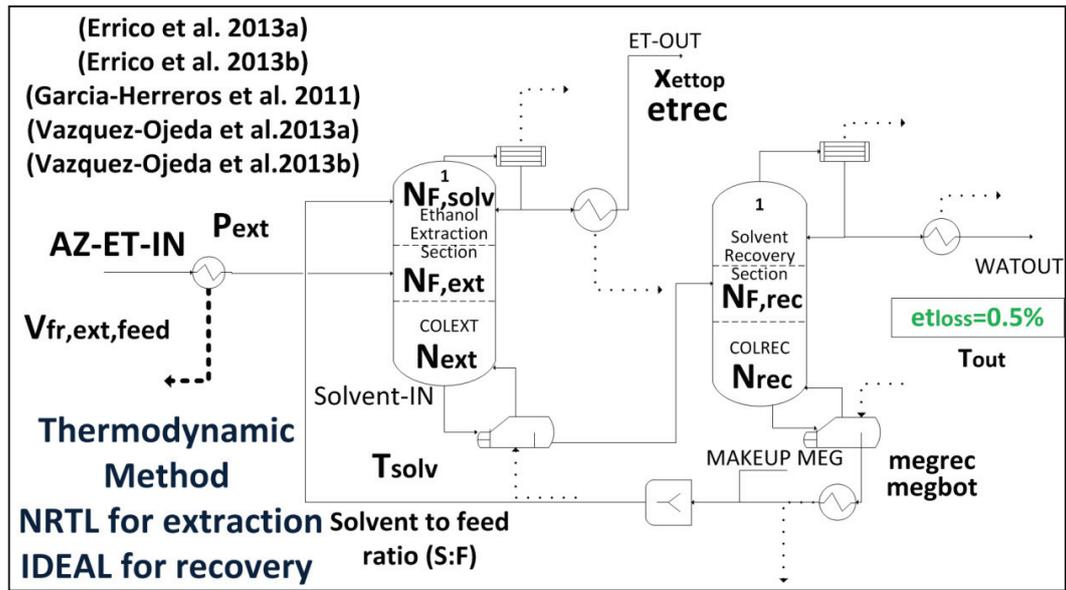
Figure 2:6 Process Flow Diagram for ethanol dehydration section: extractive distillation technology
