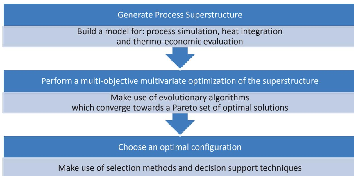
Figure 1 Summary of multi-objective method for optimal process design
