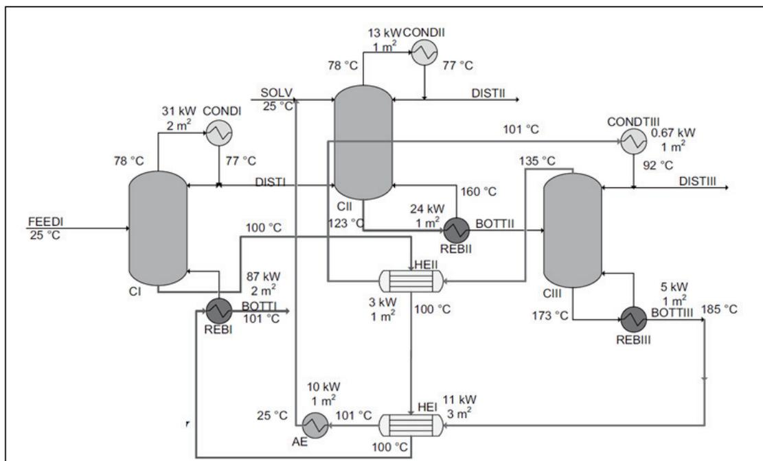
Figure 4:5 Optimized conventional scheme with heat integration as shown in [57]
