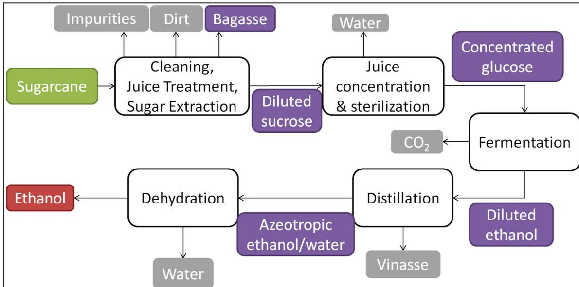
Figure 2:2 Block Flow Diagram for ethanol production section
