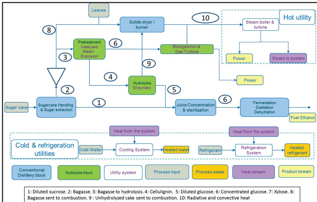
Figure 5:2 Block Flow Diagram for combined production process
