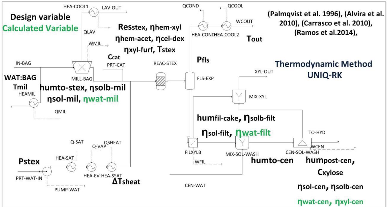
Figure 3:4 Process Flow Diagram for steam explosion pretreatment section
