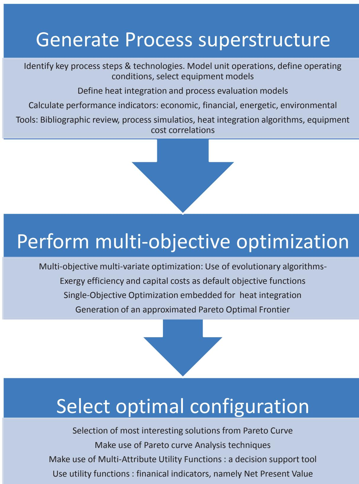
Figure 1:7 Break-down of methodology for the synthesis of optimal processes
