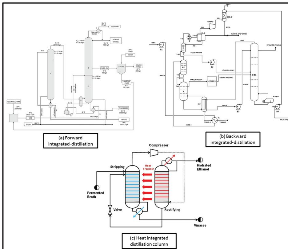
Figure 4:3 Illustrations of process design for (a) forward integrated distillation [49], (b) backward integrated distillation [44], and (c) heat integrated distillation column [50].
