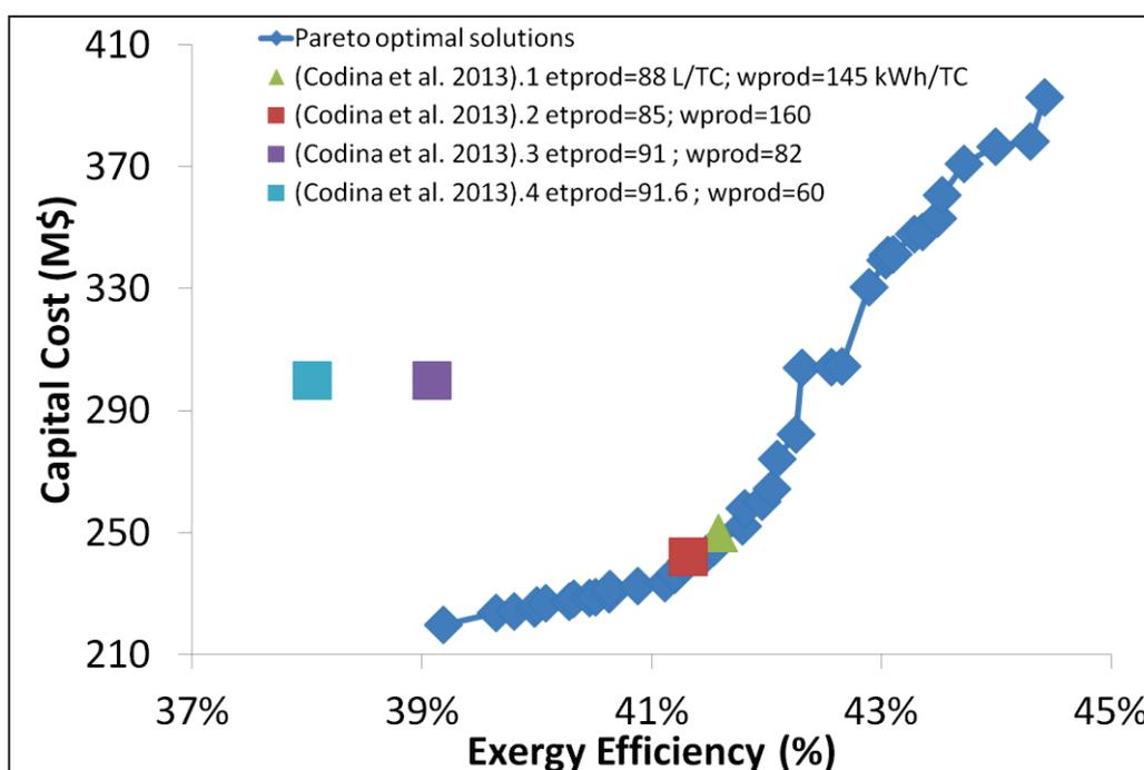
Figure 5:15 Optimization results: current optimization vs. (Codina et al. 2013) [21] plotted in exergy efficiency vs. capital cost graph
