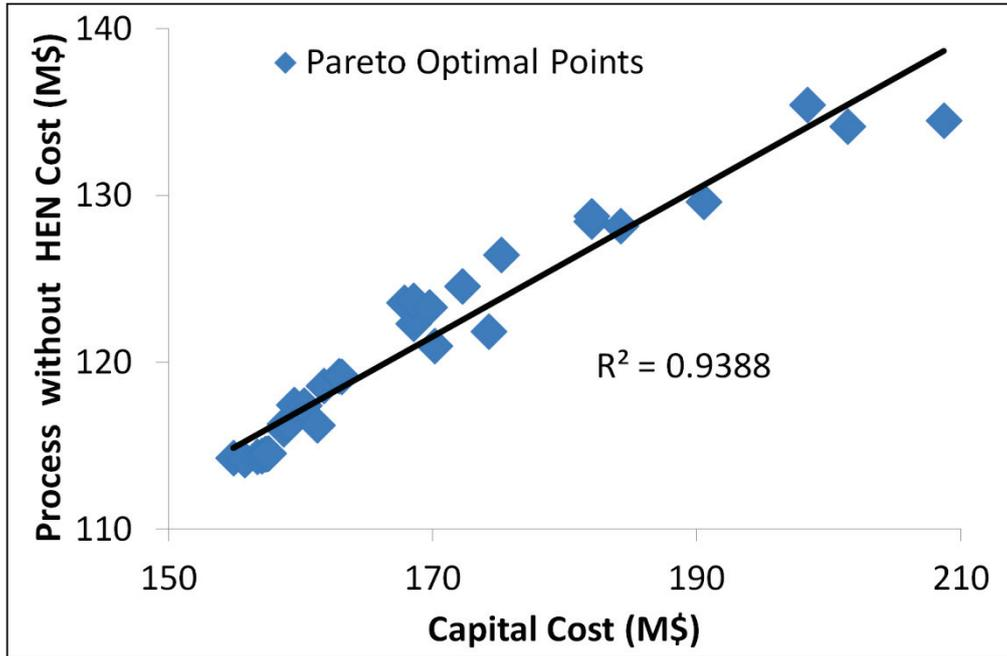
Figure 4:15 Heat Exchanger Cost vs. Capital Cost for Pareto-optimal solutions
