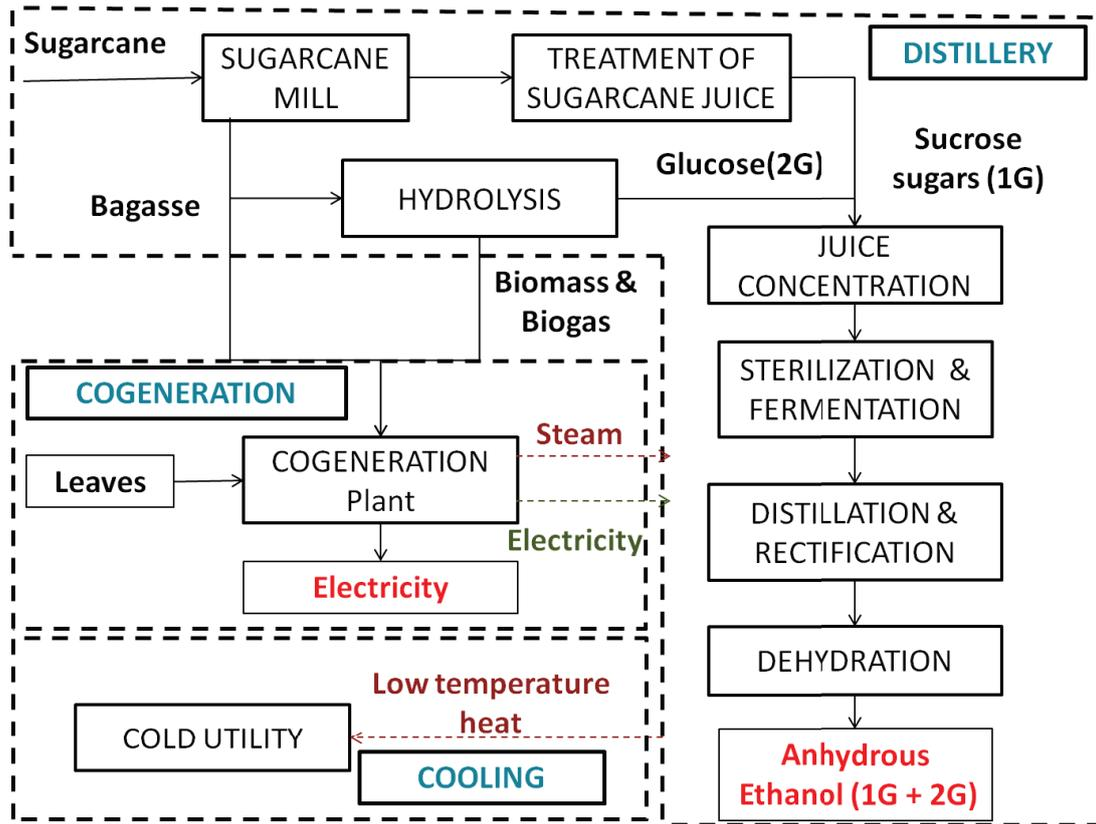
Figure 3:3 Overall scheme for bagasse hydrolysis process
