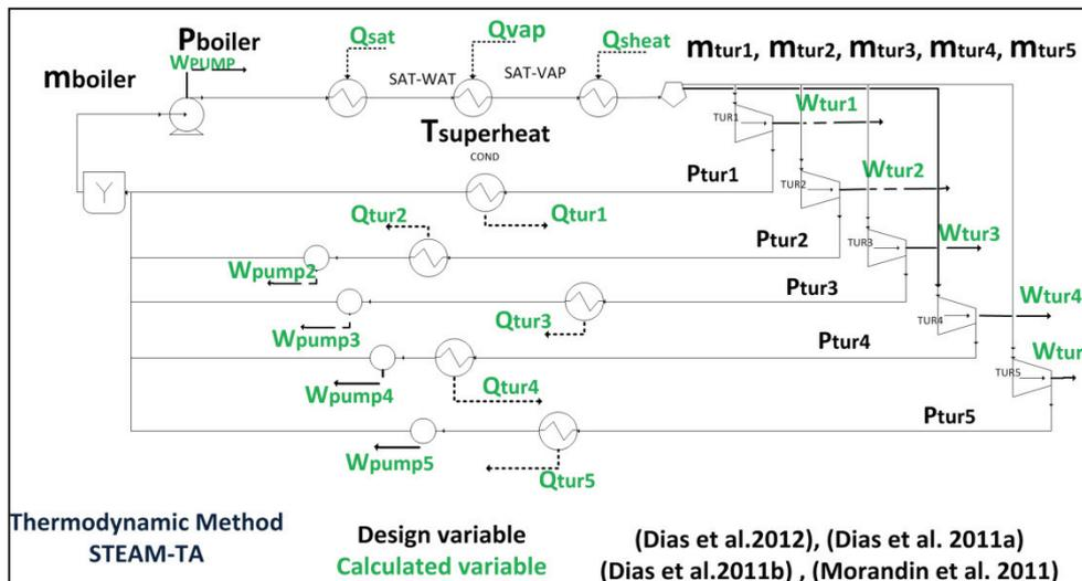
Figure 2:9 Process Flow Diagram for combined heat and power production system
