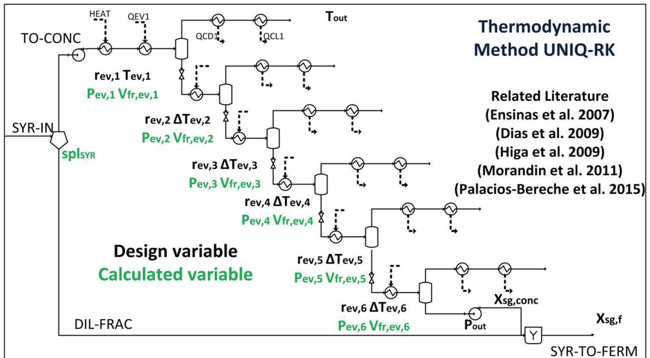
Figure 2:3 Process Flow Diagram for juice concentration section
