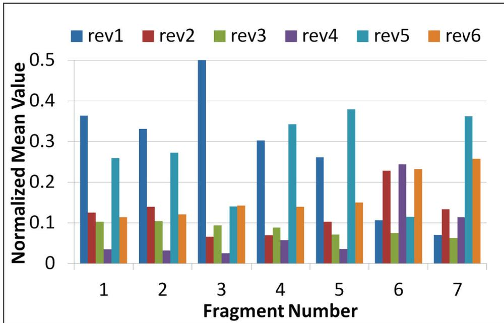
Figure 4:21 Variation of normalized mean vaporization rates along the Pareto fragments
