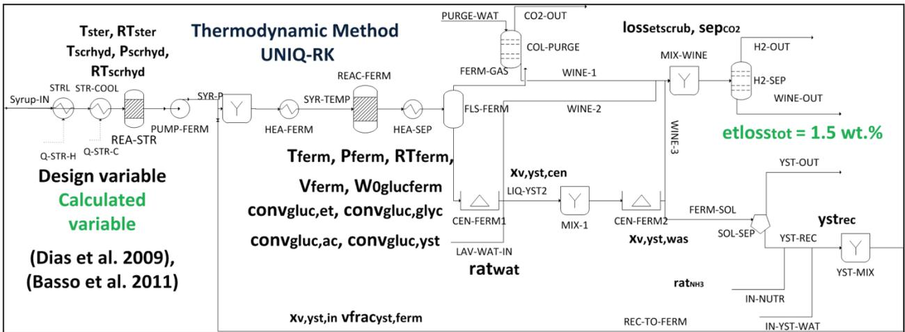
Figure 2:4 Process Flow Diagram fermentation section
