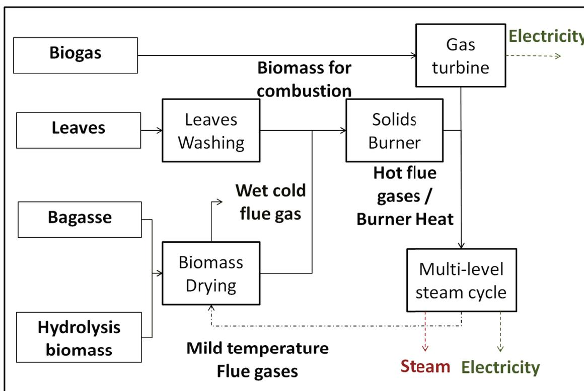
Figure 3:7 Block flow Diagram for the Cogeneration section
