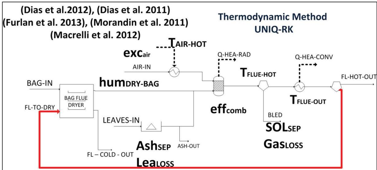
Figure 2:8 Process Flow Diagram for biomass burner
