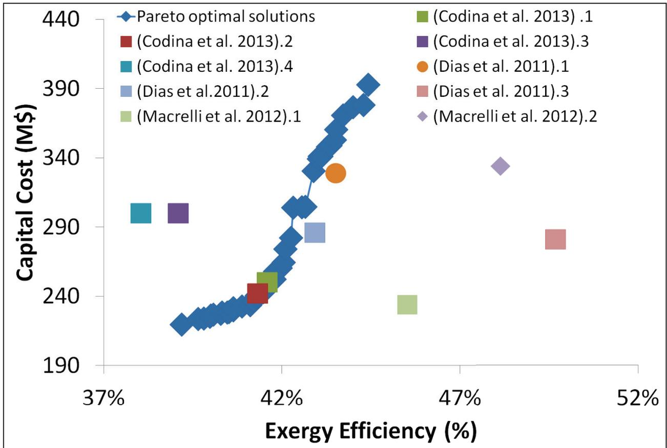
Figure 5:16 Obtained Pareto optimal results (distillery + cogeneration + enzymatic hydrolysis) vs. Various research results (Codina et al. 2013) [21], (Dias et al. 2011) [69] and (Macrelli et al. 2012) [64]
