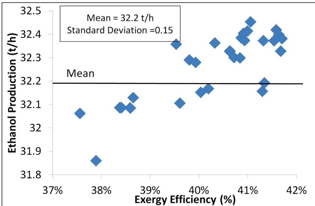
Figure 4:14 Ethanol production vs. exergy efficiency for Pareto-optimal solutions
