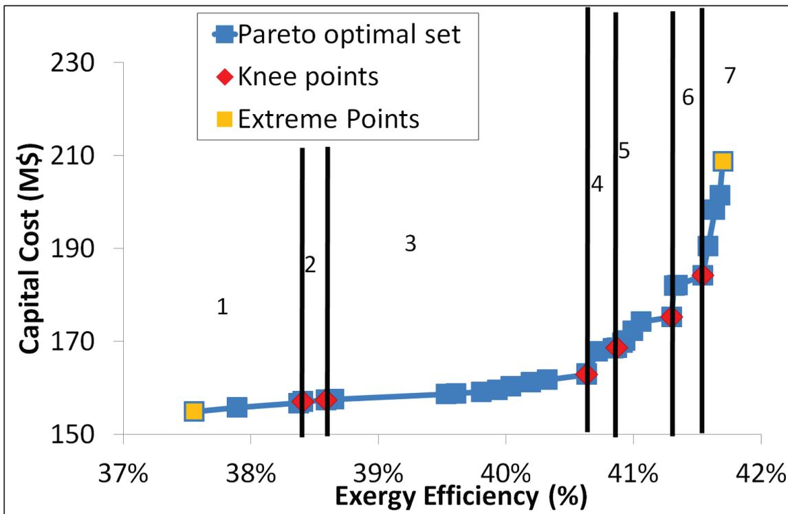
Figure 4:19 Pareto curve (capital cost vs. exergy efficiency) along with knee points and extreme points
