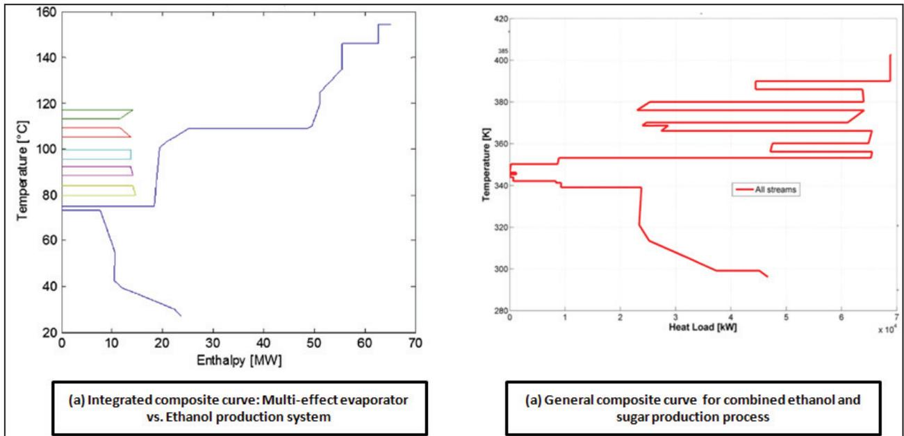
Figure 4:6 Composite curves for ethanol production process (a) Integrated composite curve [44], (b) General composite curve [28]
