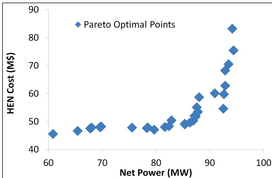
Figure 4:18 Relationship between heat exchanger cost and net power production
