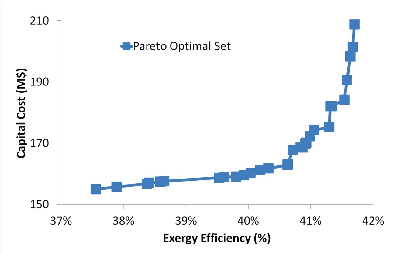
Figure 4:12 Graph for the final Pareto optimal Non Dominated Set: optimization of combined sugarcane distillery and cogeneration process
