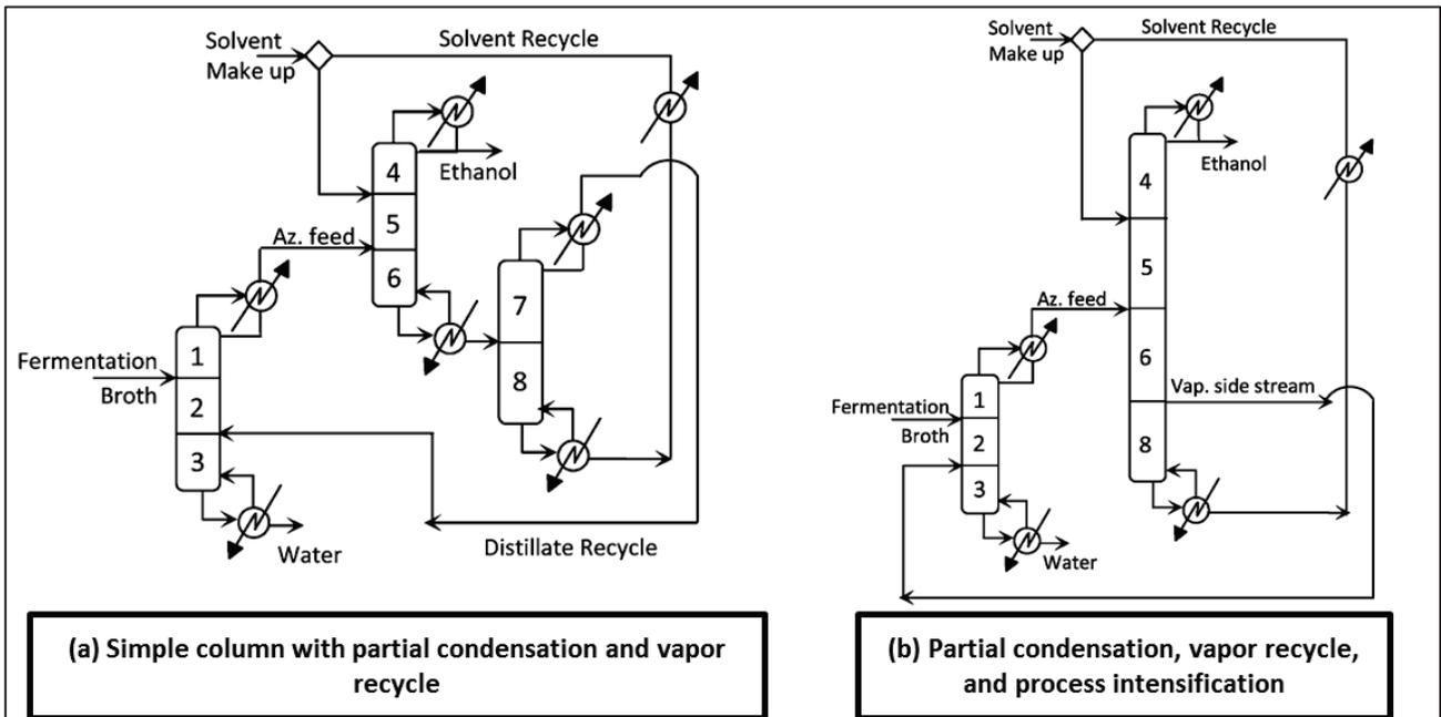
Figure 4:4 Illustration of the distillation configurations as extracted from (a) [83] and (b) [54]
