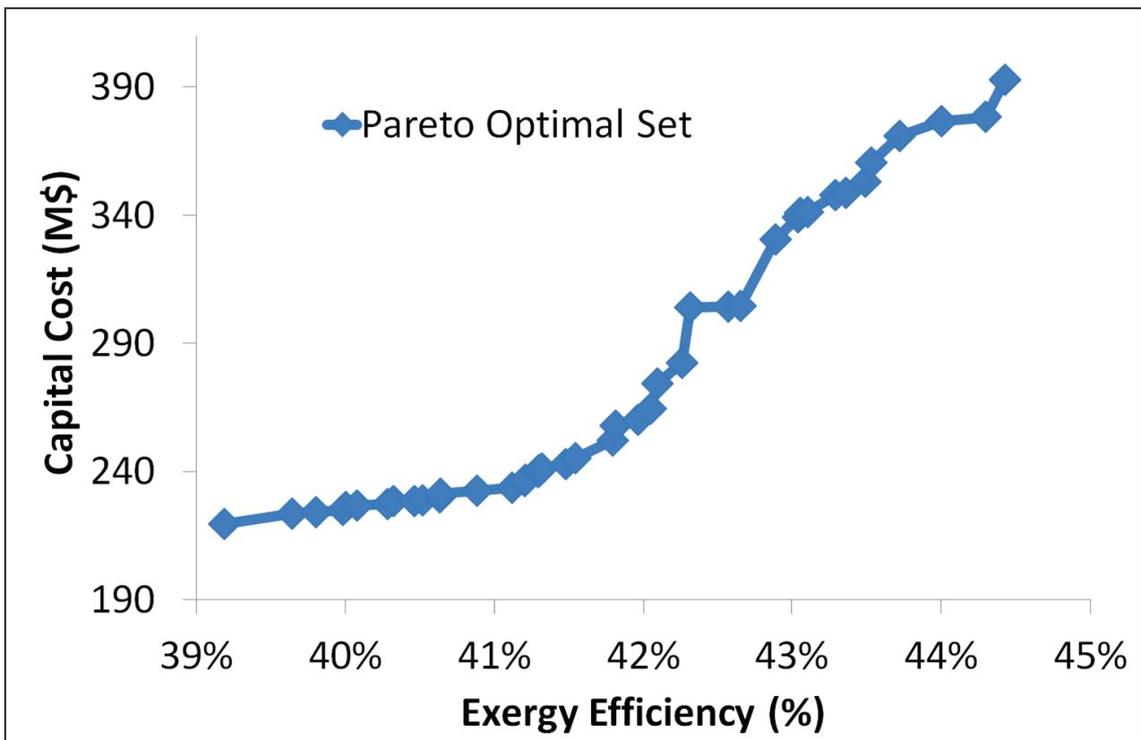
Figure 5:4 Pareto optimal set for combined distillery, hydrolysis and cogeneration configuration
