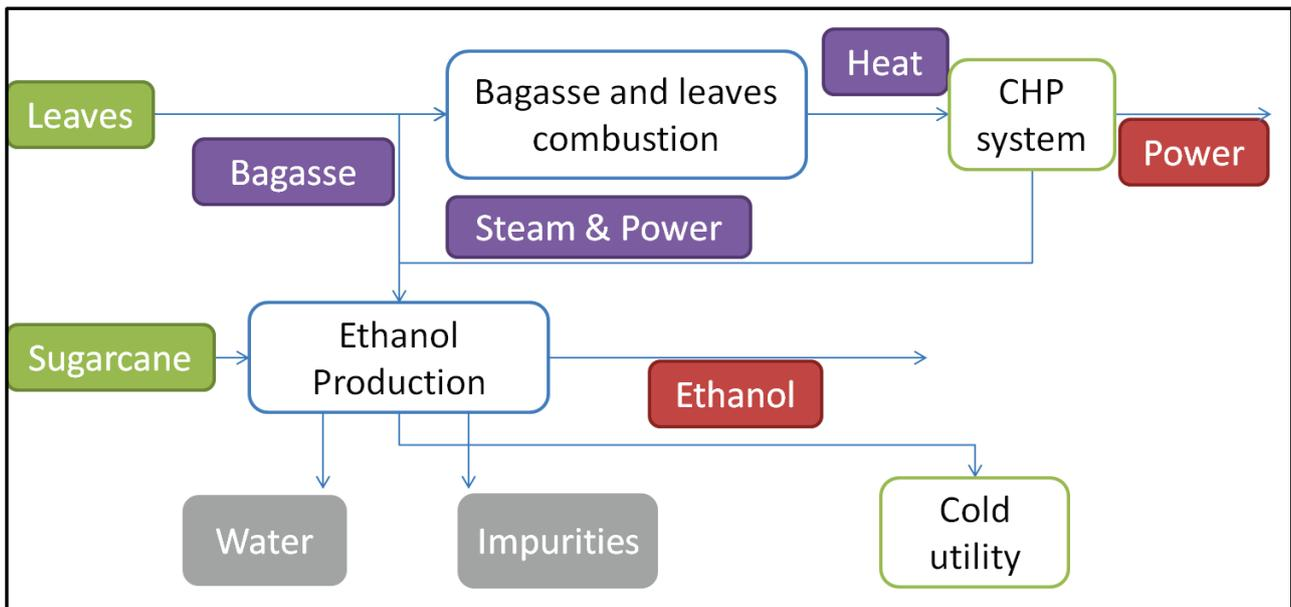
Figure 2:1 Overall scheme of sugarcane to ethanol and power process
