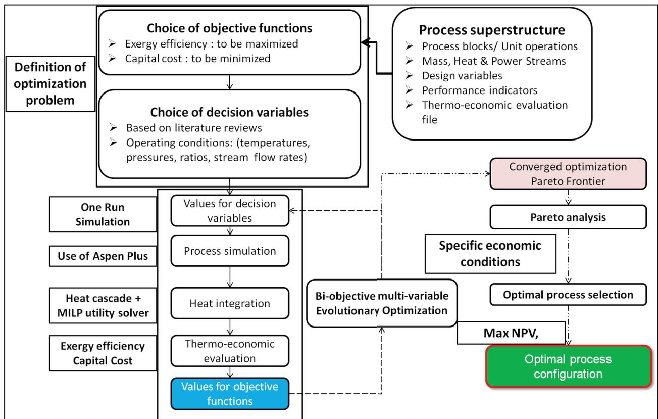
Figure 4:1 Overall scheme for proposed multi-objective optimal process design
