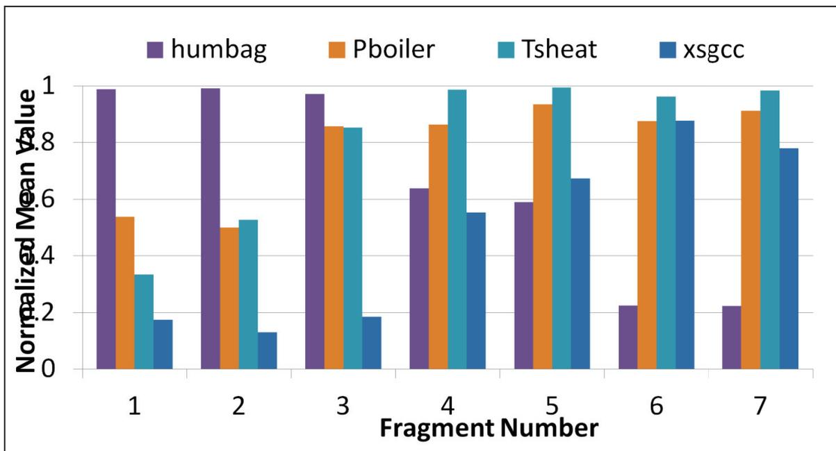
Figure 4:24 Variation of normalized values for bagasse humidity, boiler pressure, superheating temperature and sugar concentration
