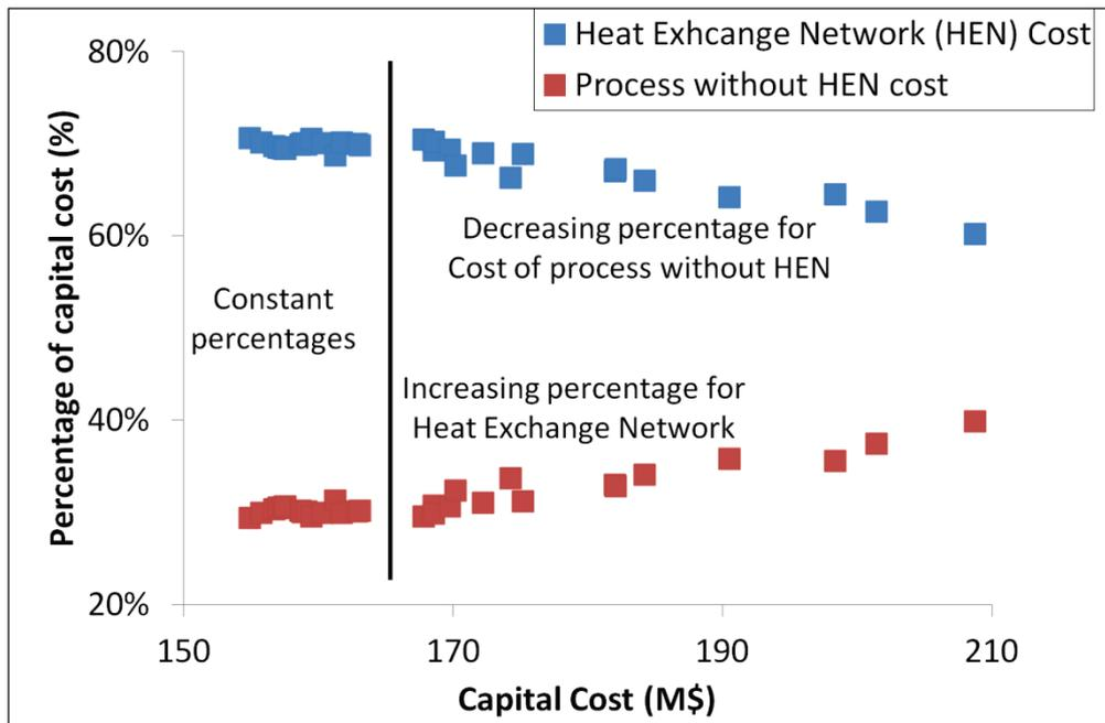
Figure 4:17 Percentage of capital cost: Relationship for Heat Exchanger Cost and Process Cost
