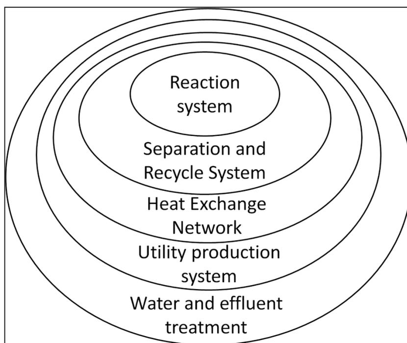
Figure 1:2 Graphic representation of onion model. Integral process design is obtained going from the reaction system outward to the effluent treatment system
