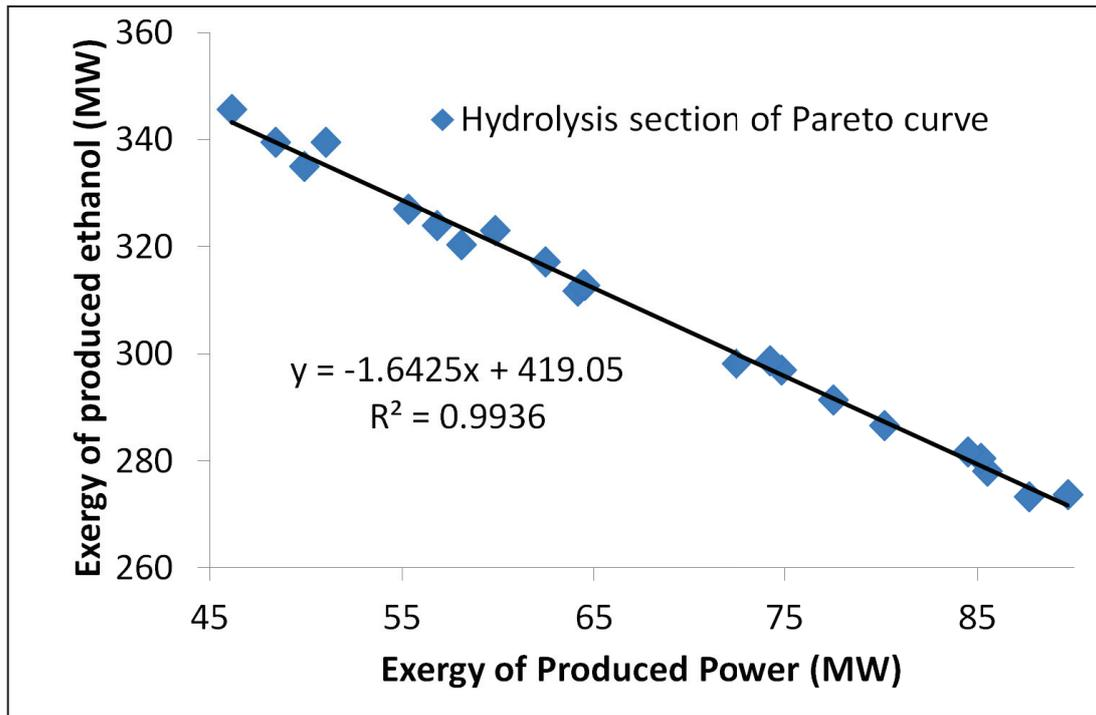
Figure 5:13 Evolution of ethanol production vs. power production for ethanol producing alternatives
