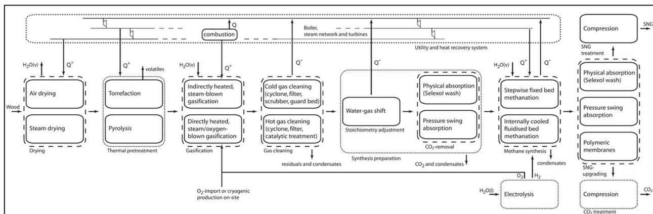
Figure 1:3 Superstructure for biomass methanation process [5]
