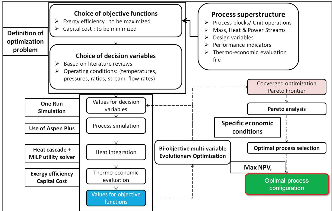
Figure 5:1 Overall scheme for proposed multi-objective optimal process design
