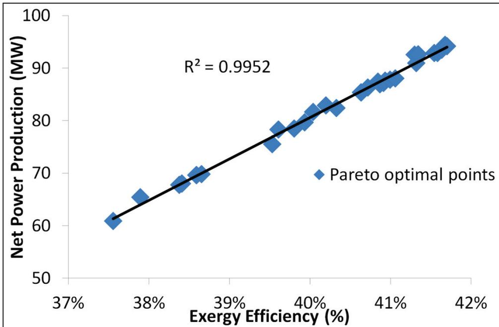
Figure 4:13 Net power production vs. exergy efficiency for Pareto-optimal solutions
