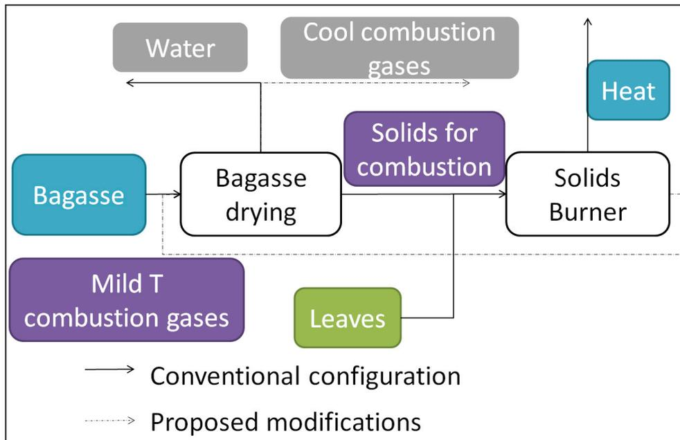
Figure 2:7 Block Flow Diagram for bagasse and leaves conventional valorization section
