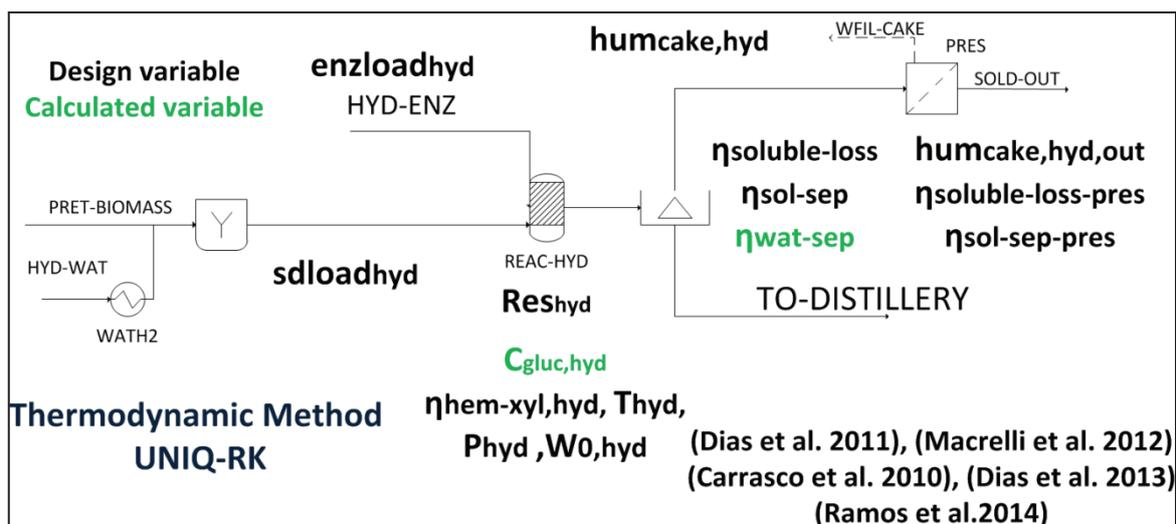
Figure 3:5 Process Flow Diagram for enzymatic hydrolysis section
