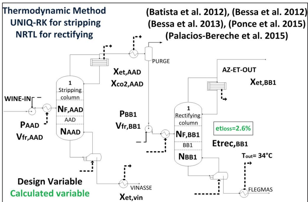
Figure 2:5 Process Flow Diagram for ethanol distillation section
