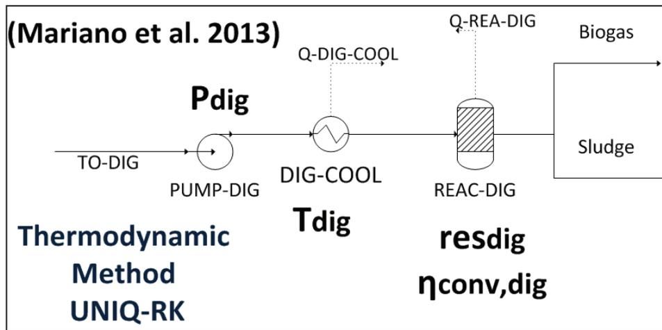
Figure 3:6 Process Flow Diagram for biodigestion section
