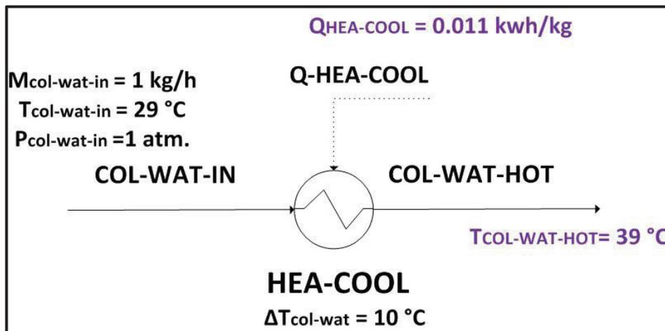
Figure 2:10 Process flow Diagram for process cooling water utility
