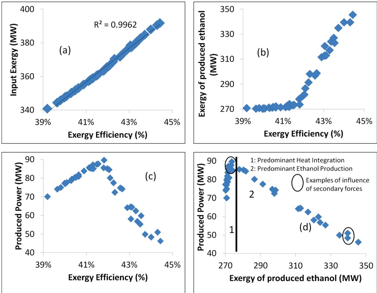
Figure 5:5 Relationships for optimal points between (a) exergy efficiency and produced exergy content (MW), (b) exergy efficiency and ethanol exergy content (MW), (c) exergy efficiency and net power production (MW), and (d) ethanol exergy and net power production.
