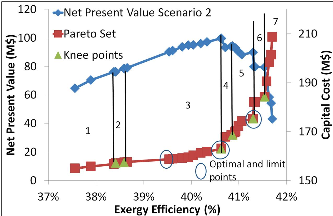
Figure 4:29 NPV vs. Exergy Efficiency & Capital cost vs. Exergy efficiency for optimal Pareto system. Identification of NPV based fragmentation
