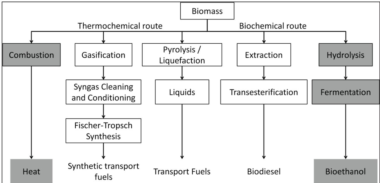
Figure 3:1 Diagram of the main biofuel production pathways [70] – Pathways considered in this chapter highlighted in grey
