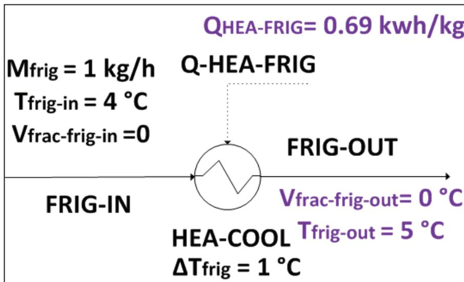
Figure 2:11 Process flow Diagram for process refrigerant utility
