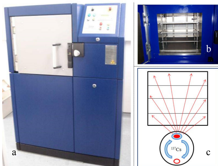
Figure II.1: a) \gamma source of ^{137}\text{Cs} at Arronax facilities, b) different irradiation levels and c) schematic of reaching \gamma rays from the source to different levels.
