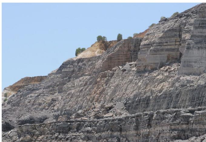
**Figure 3:** Highly fractured walls and detached blocks observed in an open pit coal mine (Australia)
