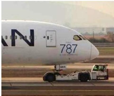
Figure 2.2: A towing tractor
