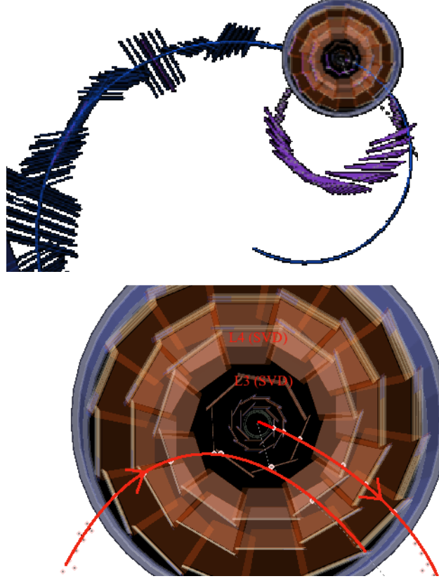
Figure 4.1: Illustration of the difficulty to reconstruct low momentum tracks. These two pictures are event displays of the Belle II detector, showing a transversal view of the detector. Two tracks were reconstructed by mistake instead of one curling track. On the upper view, the two reconstructed tracks are represented in blue and in the zoom below, we represent in red how the reconstructed track should have looked like.
