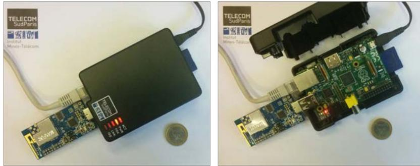
Figure 4.4: 6EdR hardware: Raspberry Pi with an Ethernet interface and a CM5000 mote as an IEEE 802.15.4 interface.
